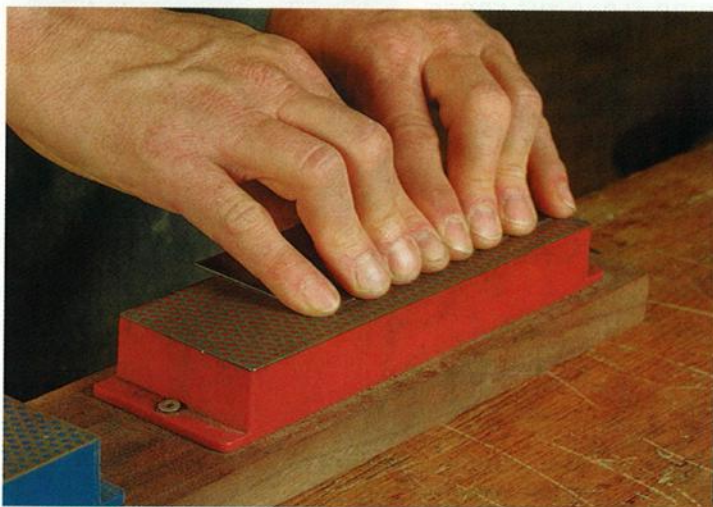
Hone the sides of the scraper. Polish the sides of the scraper on a fine diamond plate or sharpening stone.
