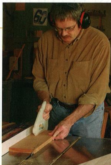
Slow going. A dull tablesaw blade requires more effort to feed stock into the cut, and the difference shows in the work. Although a dull blade won't look markedly different from a sharp one, it can leave stock looking burned and scarred.
