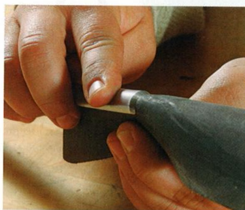
Put a curl in it. Faia simply folds the strop over to work the inside of the gouge.
