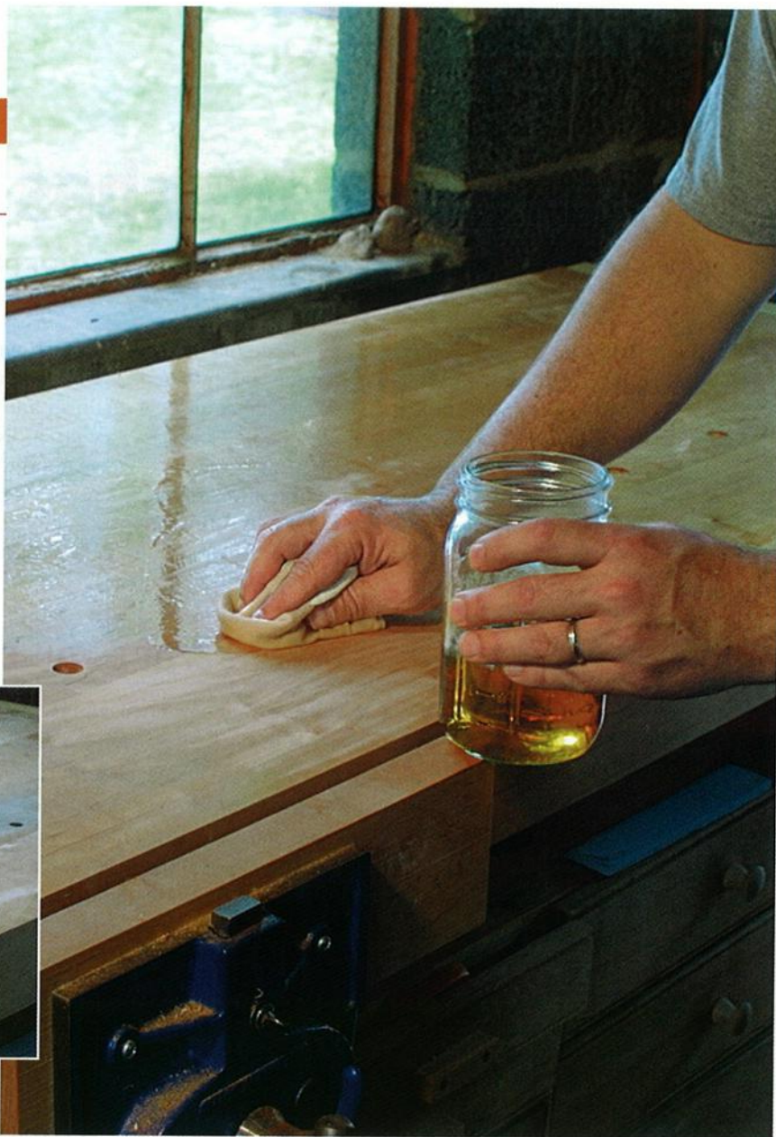
Lay it on heavy. Apply the oil-varnish mixture liberally and allow it to soak in for 10 minutes before wiping off the surplus with a clean cloth.
