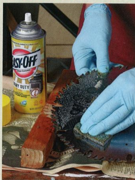
Use a cleaner on tablesaw blades. Spray it on the buildup and let it sit before scrubbing with a brass brush.
