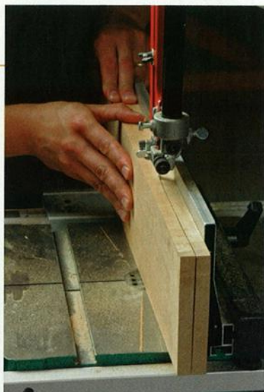
More push needed. The extra force required to feed stock into a dull bandsaw blade can cause the blade to wander. A rough, wavy cut is the result.
