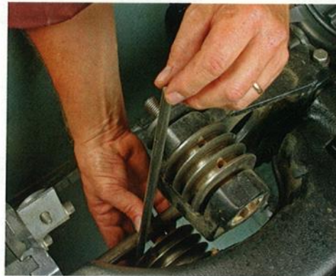
Align the pulleys. Use a length of drill rod or other straightedge to determine whether the motor and arbor pulleys are aligned with one another.
