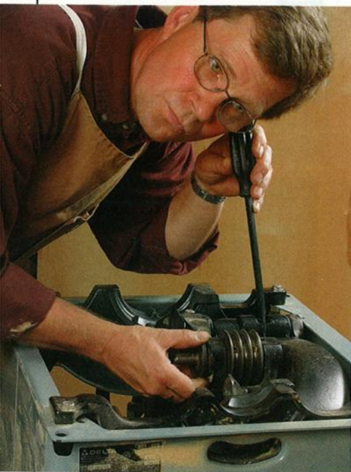
An old hot-rodder's trick. A long screwdriver, with the tip held firmly on the bearing housing, makes a good listening device for checking the condition of the bearings.
