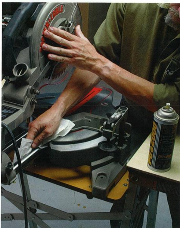
Lubricate with two different kinds of oil. Use penetrating oil on the sliding mechanism and light machine oil on pivot points for the head rotation.
