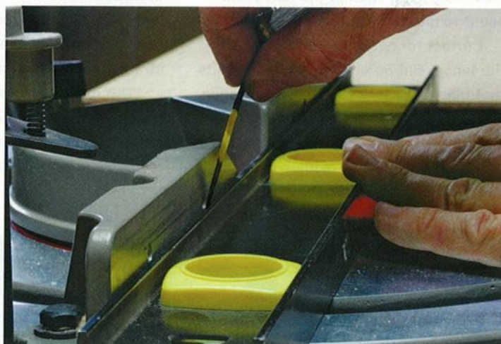
Start with a flat fence. Slightly bent fences may be pushed back into alignment. White checks the fence with feeler gauges.
