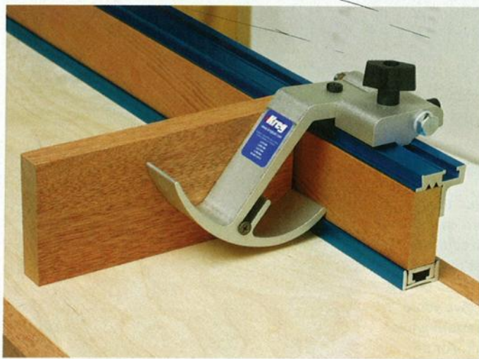
Stop block for miters. Screw a block of wood to the stop block to give mitered ends a larger surface to register against.
