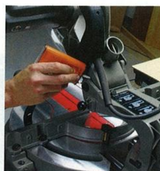
Lubricate with two different kinds of oil. Use penetrating oil on the sliding mechanism and light machine oil on pivot points for the head rotation.
