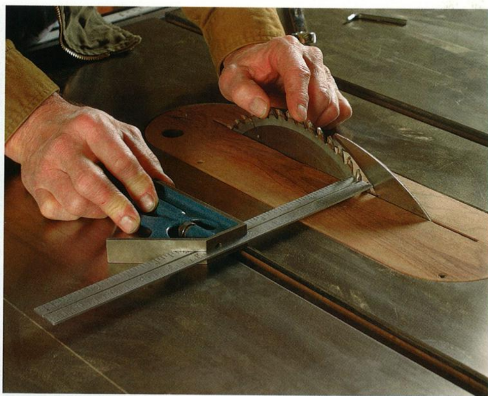
Adjust the miter slot. The combination square also can help check whether a table-saw's miter slot is parallel to the blade. Mark a tooth at the front of the blade and measure the distance from the blade to the slot. Next, rotate the marked tooth to the back of the blade opening and measure again. If the readings are different, you need to adjust your saw's tabletop or trunnions to bring the slot parallel with the blade.
