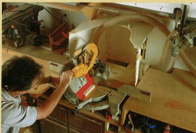
A built-in miter saw. Putting a miter saw into an existing bench provides support for long pieces and a dust-collection booth.
