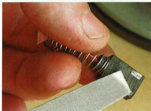
File to fit. The brushes should slide into the housing easily so that the spring can keep the brushes in good contact with the commutator. If the fit is tight, smooth the edges of the brush with a fine file.
