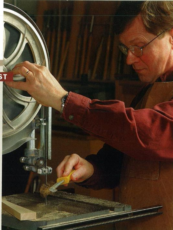
Clean bandsaw gullets. With the machine turned off, rotate the upper wheel by hand as you pass a brass brush over the blade.
