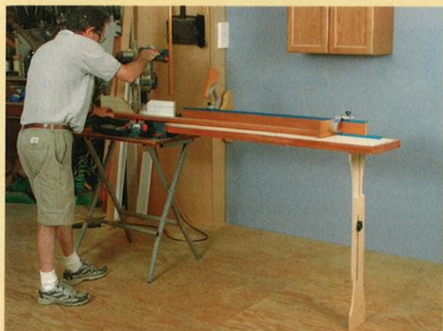
Good cuts need good support. A pair of extension wings with stop blocks support long pieces and make for accurate cuts.
