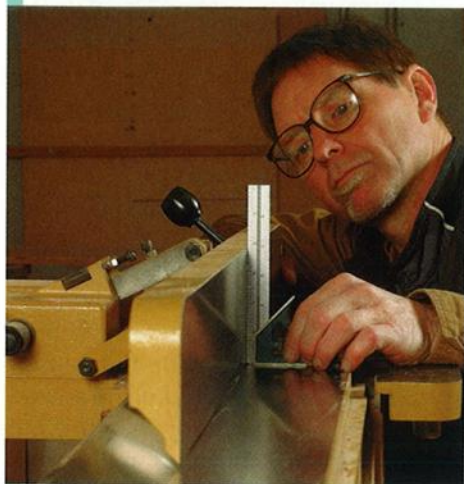
Check the fence. Use the combination square to ensure that a jointer's fence is set at 90° to the tables. Make similar checks on the tablesaw and bandsaw.
