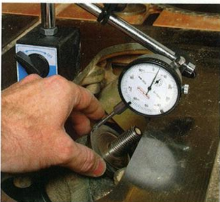
Check for runout. Set the pointer of the dial indicator perpendicular to the rim of the arbor flange. Rotate the flange to check for variations in flatness.
