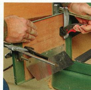
Let air sweep the floor. A thin plywood panel blocks all of the louver slots in the access door, except the lowest. Because that slot is still several inches above the new floor, install a sheet-metal louver to direct incoming air down to the floor. Attach the panel with construction adhesive.
