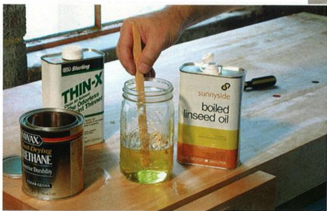
Mix the finish. Minick's mixture of oil, varnish, and paint thinner contains a higher proportion of resin than most Danish oils to give the bench greater protection. Each coat dries to the touch in about an hour.
