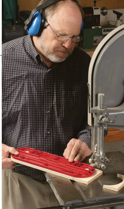
Round the ends. A bandsaw does this best, but a jigsaw also works. Leave about \frac{1}{16} in. of extra material.
