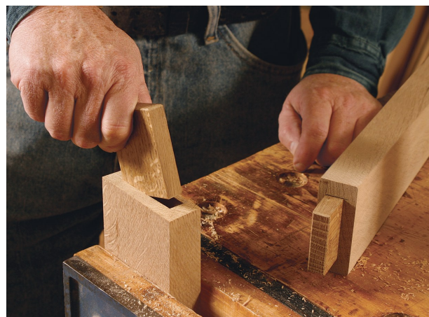
Square up the mortises. Although some people leave router-cut mortises rounded at the ends, shaping the tenons to fit, Rodel prefers to square up mortises with a chisel and mallet. Slip tenons should fit with only a bit of hand pressure.
