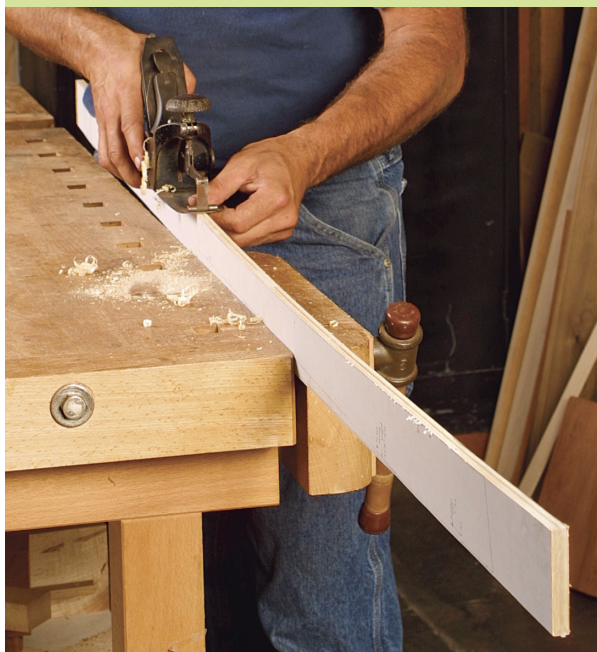
Plane a concave curve. Tune the sole to a slightly tighter inside radius than the curve to be planed and keep pressure on the nose with each pass.
