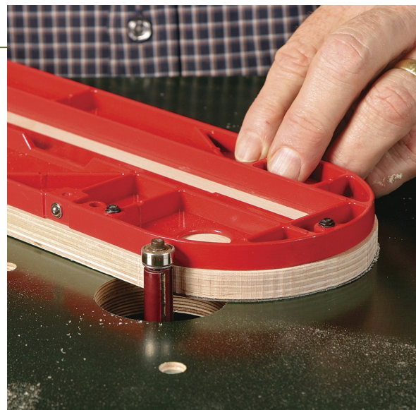
Trim the blank. Rout the insert flush to the throat plate with a bottom-bearing, flush-trimming bit.
