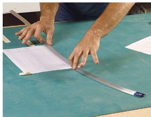
Commercial drawing tool. A flexible curve, available from a woodworking, art, or drafting-supply catalog, can be bent into a fair curve and will hold its form.
