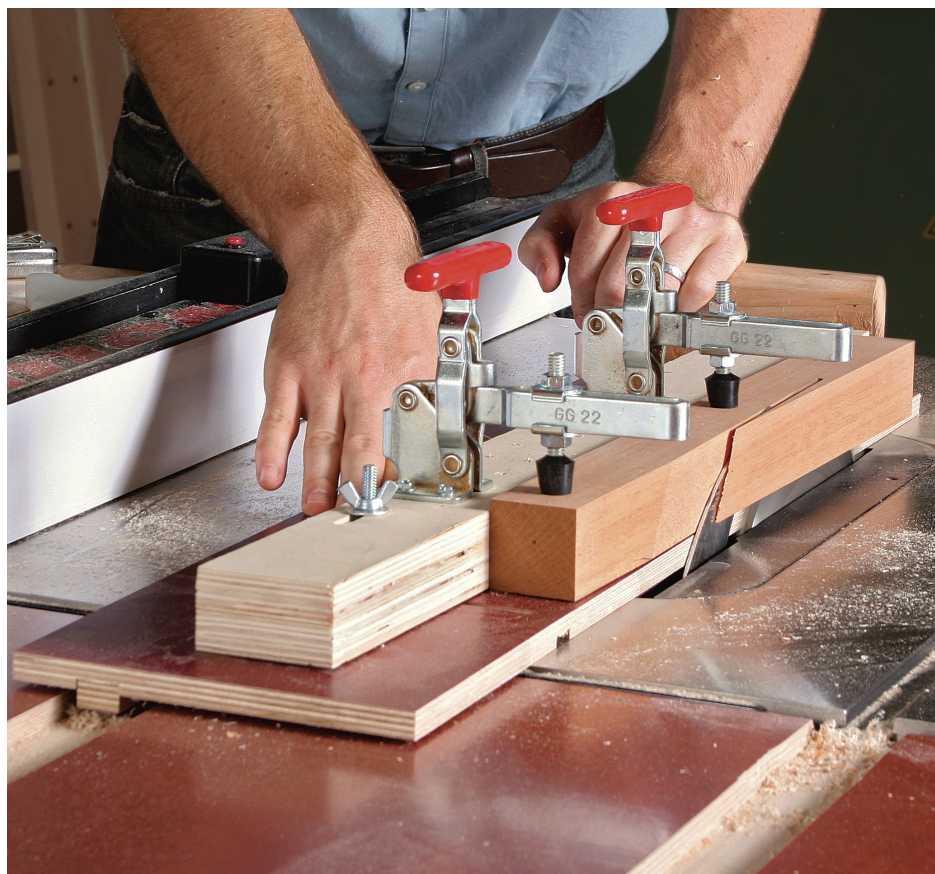
Slick jigs. A phenolic-plywood tapering jig rides in the miter slot and across the surface of the tablesaw. Since the blade also trimmed the edge of the jig, that edge is the reference line.
