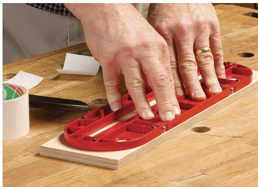
Throat plate becomes template. Attach the throat plate to the blank with double-sided tape.
