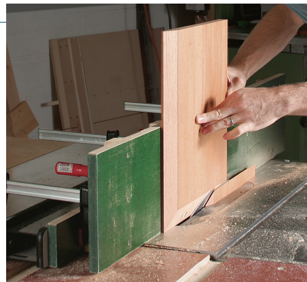
Versatile tablesaw fence. The shorter, sacrificial side is used with a dado set to cut rabbets (left). The tall side is perfect for raising a panel (above). The extra height supports the tall panel as it slides easily across the fence.
