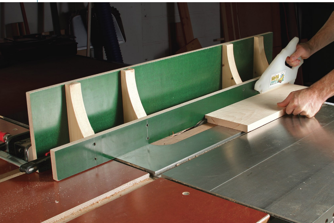
Versatile tablesaw fence. The shorter, sacrificial side is used with a dado set to cut rabbets (left). The tall side is perfect for raising a panel (above). The extra height supports the tall panel as it slides easily across the fence.
