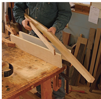
Angle block orients the leg. Cut the block to the angle needed, then set it against one side of the leg and add the wedges. Cut the mortise with a plunge router.
