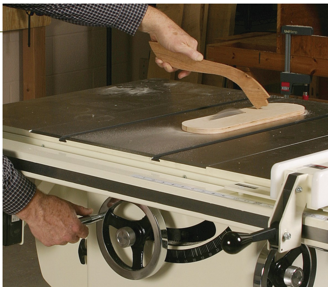
Two openings to cut. Hold down the blank with a push stick (left), staying away from where the blade will come through. Raise the blade slowly. Afterward, mark the opening for the blade-guard assembly (above) and cut it with a bandsaw or jigsaw.
