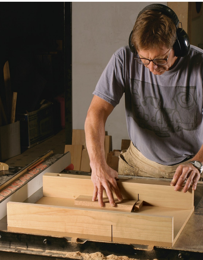
Every saw needs one. A shopmade sled makes more accurate crosscuts than a miter gauge can.
