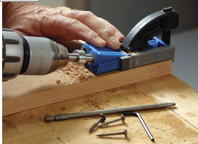
Pocket holes in a jiffy. The R3 jig attaches easily to the workpiece with almost any bar or C-clamp. The lip on the end references the edge of the workpiece.
