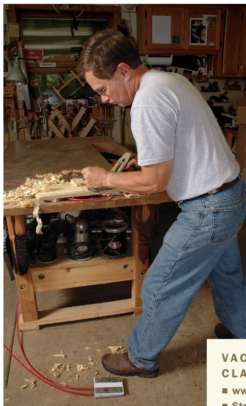
Clamping without clamps. The VacuClamp system holds a workpiece in place using vacuum pressure. To release the workpiece, simply press the foot switch.
