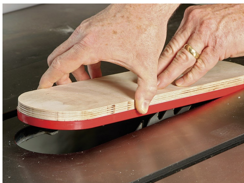
Don't remove the blank. Even at its lowest height, a 10-in. blade prevents a blank from dropping into the throat. So you'll want to cut the blade opening while the blank is taped to the insert.
