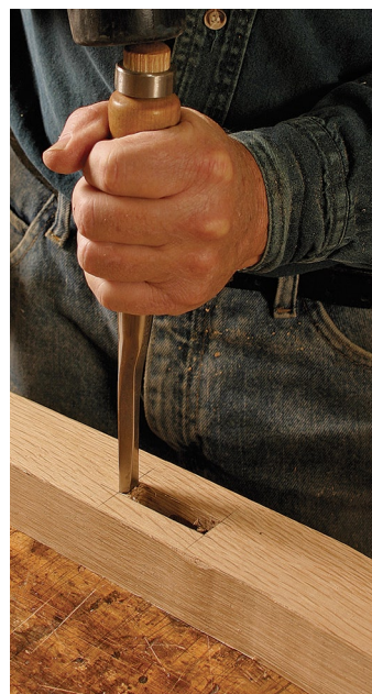
Square up the mortises. Although some people leave router-cut mortises rounded at the ends, shaping the tenons to fit, Rodel prefers to square up mortises with a chisel and mallet. Slip tenons should fit with only a bit of hand pressure.
