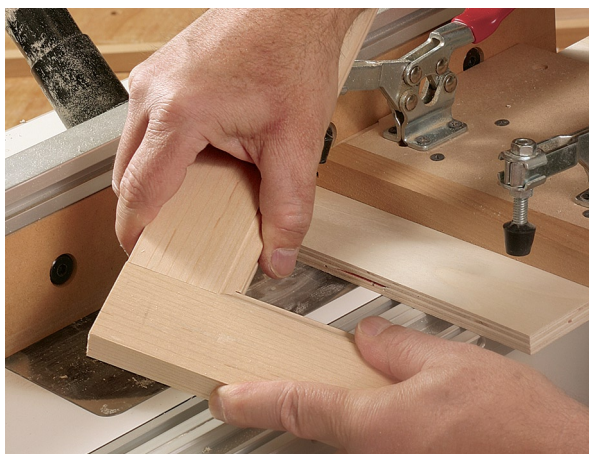
The finished joint. The router-table sled lets you cut the ends of the rails square, producing a tight cope-and-stick joint with no tearout.
