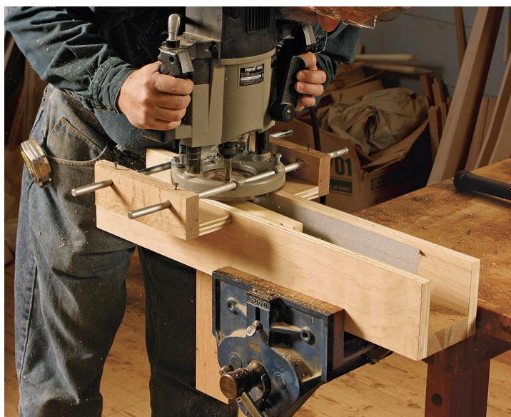
Mortise the ends of workpieces. Mortises in end grain, typically for slip tenons, are easily cut by wedging the work vertically in the router box.
