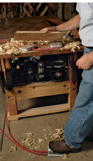
Clamping without clamps. The VacuClamp system holds a workpiece in place using vacuum pressure. To release the workpiece, simply press the foot switch.
