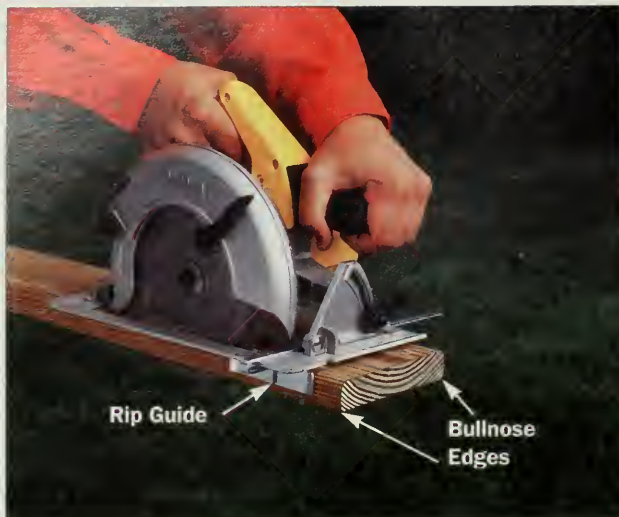
Figure 1: Rip the rounded bullnose edges from \frac{3}{4} decking boards using a rip-guide attachment on your circular saw. Then rip the boards again to final width.
