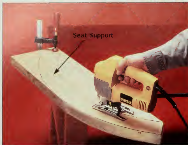
Figure 1: Cut curved parts with a jigsaw after enlarging the shapes from the grids in the drawing. Cut one example of each curved part, then use it as a template to mark all similar ones.
