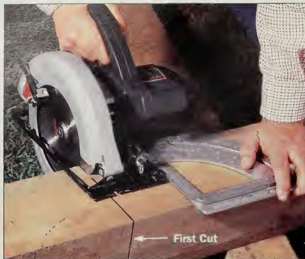
Figure 1: Cut tops of posts with two passes of your circular saw. Be sure to use a square to guide the saw, and practice on scrap first. Caution: wear a dust mask when cutting and sanding treated lumber.
