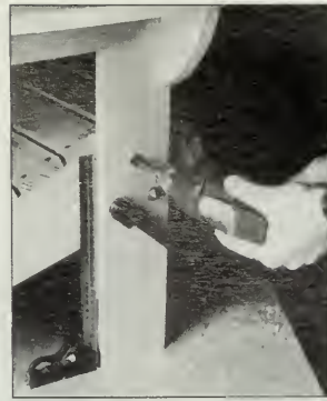
Figure 5: Make sure the legs are square to the ground before drilling the bolt holes.
