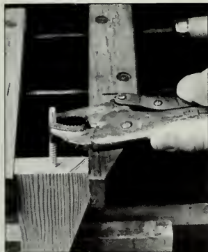
Figure 3: Use clamps to hold the ends of the braces (K, L) when screwing in the hanger bolts. This will keep the wood from splitting.
