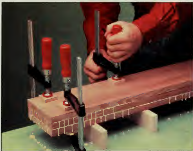
Figure 1: Fabricate the thick material for the back legs by laminating three thicknesses of ordinary \frac{3}{4} -inch lumber. Use a waterproof glue and align the edges of the boards.
