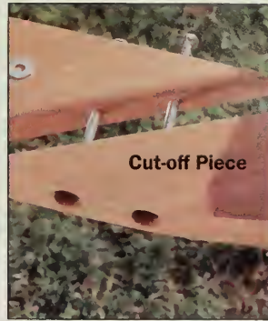
Figure 9: Begin the slide by cutting the rail at an angle and flipping the cut-off piece around. Round off the corner and bolt the piece on.
