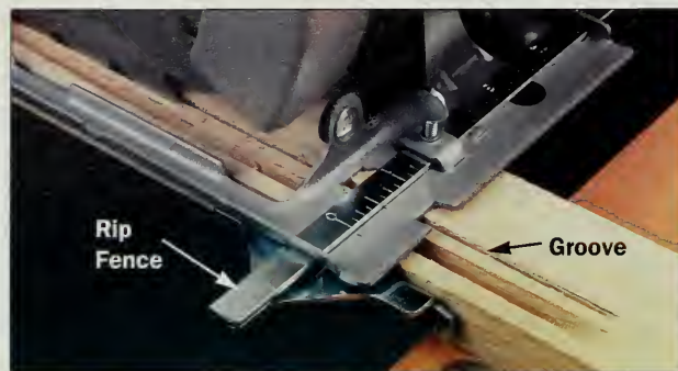
Figure 9: Cut a groove by making several passes in a long board with a circular saw, then cut off what you need. Use a rip fence.
