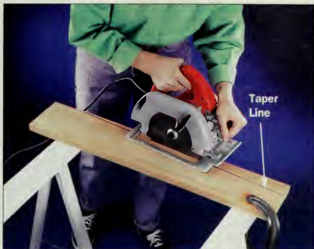
Figure 1: Cut the chair parts with your circular saw. Make tapered cuts for the arms of the chair.
