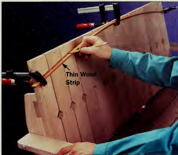
Figure 5: After the back is in place, draw a smooth curve at the top of the back by following a flexible strip of wood, called a “batten,” clamped at the center and ends.
