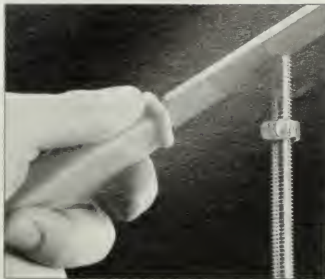
Figure 1: File cut ends of threaded rod to remove the burr. Backing the nut off will clean the threads.
