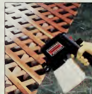
Figure 6: Paint lattice panels with a paint sprayer. You can paint on the ground or paint the whole arbor after completion.
