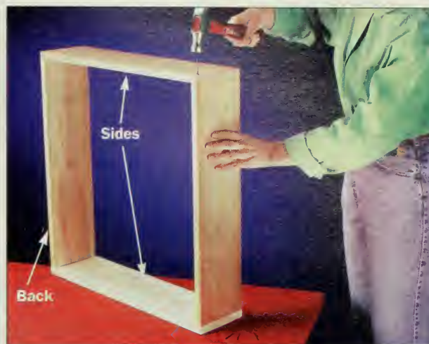
Figure 2: Nail together a box to begin the chair assembly. Nail through the sides and into the front and back pieces.
