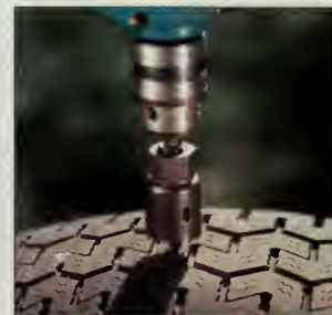
Figure 15: Tires for the climber need a drainage hole in the bottom. Use only bias-ply tires.
