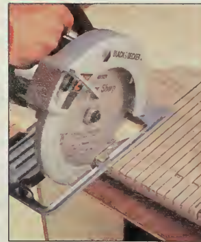
Figure 10: Kerf-cut plywood so it can bend at the bottom of the slide. With care, you can cut the kerfs by eye, just following the cut before.
