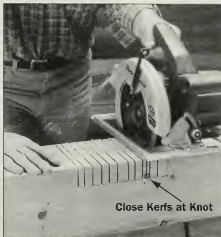
Figure 2: Begin sawing just inside one mark. Cut a series of kerfs ½ inch to ¾ inch apart. Make many close cuts through hard knots.
