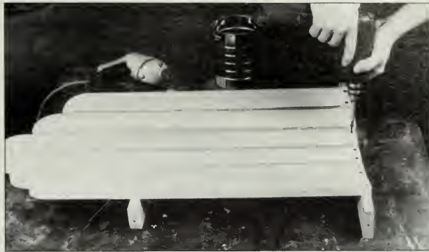
Figure 4: Screw the back slats to the lower brace first, then attach the middle brace 10 1/4 inches above it.
