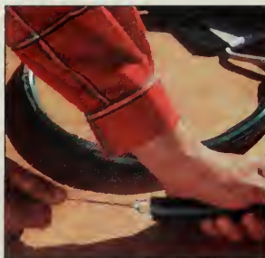
Figure 13: Pull swing chain through 3/4-inch garden hose with a wire. The hose protects children's fingers and keeps the chain from rusting.
