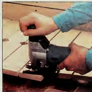
Figure 6: Cut the curve at the top of the back with a jigsaw and fine-toothed blade. Cut as close to the line as you can without cutting it away.
