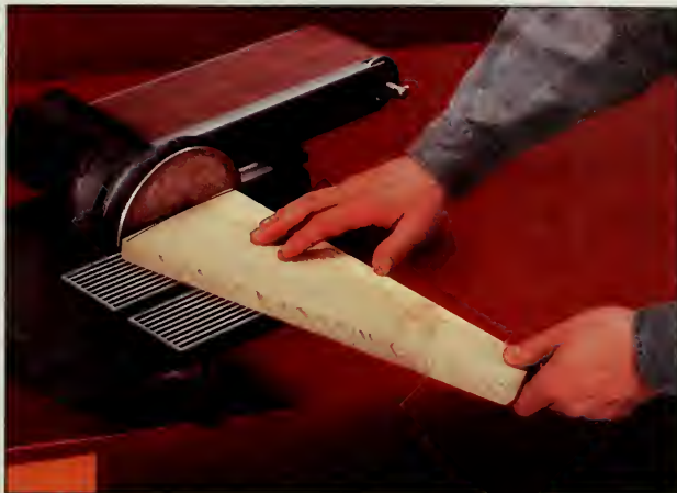
Figure 3: Sand the front ends of the seat slats to a curve using either a disc sander, as shown here, or by clamping each piece in a vise and using a belt sander.
