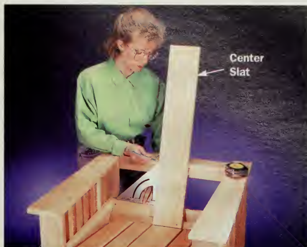
Figure 6: Add back and seat slats, starting in the middle and working out. Keep the slats square to the frame.
