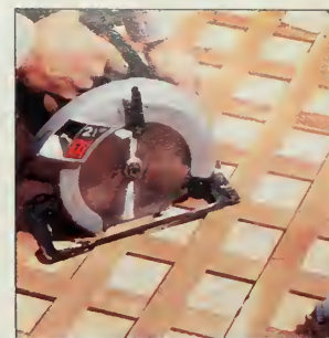
Figure 5: Support lattice panels with scrap plywood for cutting. A carbide blade will cut through the staples without dulling.
