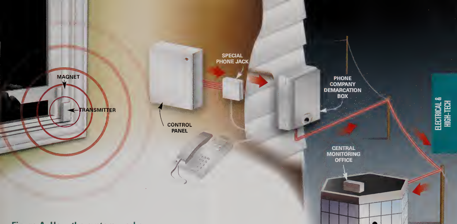
Figure A: How the system works
