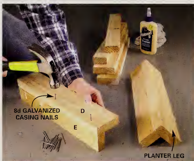
3 RIP 5/4 decking material and cut it to length for the legs. Glue and nail a 3-in. piece to a 2-in. piece.
