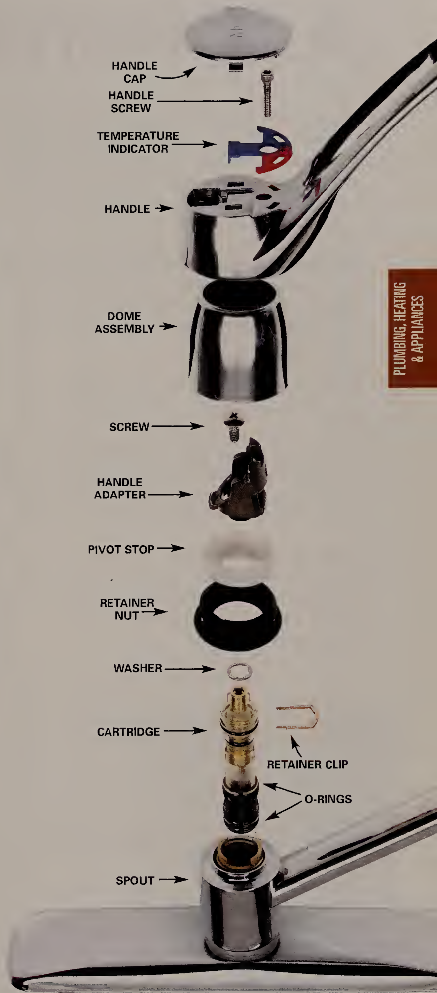
Figure B: Cartridge Faucet Parts
