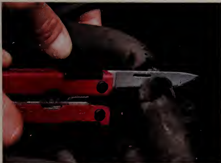
Cut out the bad section of hose
