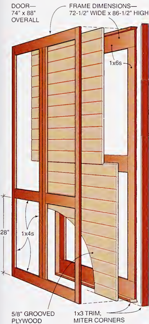
FIGURE C Sliding door details
