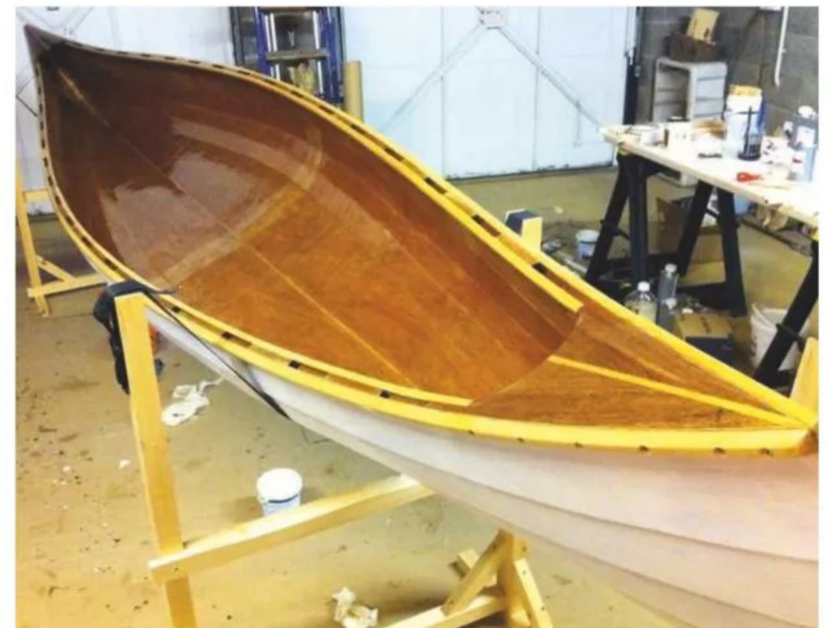
16 A coat of self-etch primer was then applied to the hull's exterior
