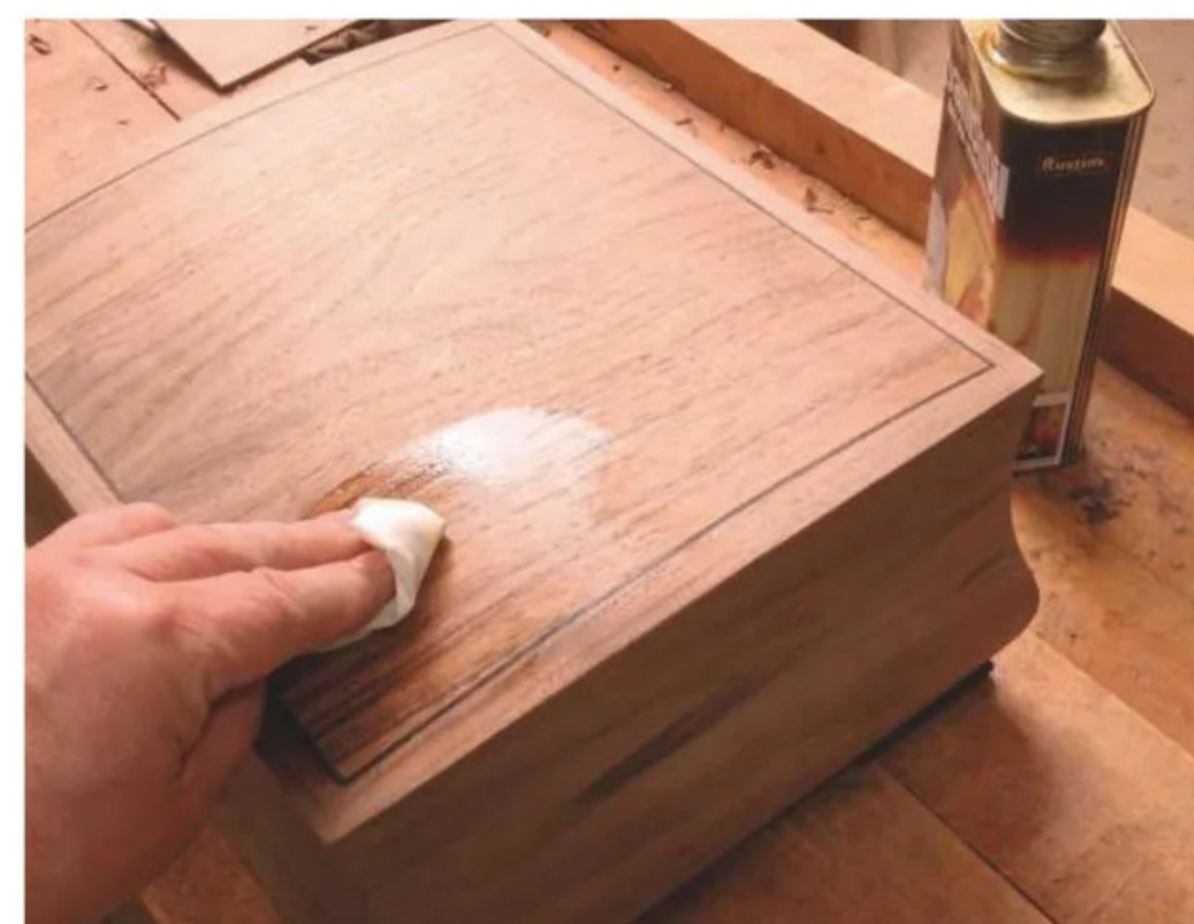
17 Danish oil rubbed into bare wood, such as this English walnut, produces a tough semi-matt finish that can be improved with age
