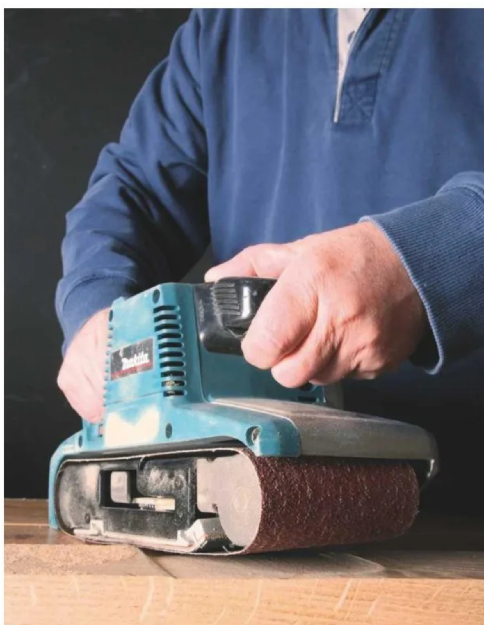
5 Although the belt sander is fast and powerful for removing wood, it's not widely used by fine furniture makers
