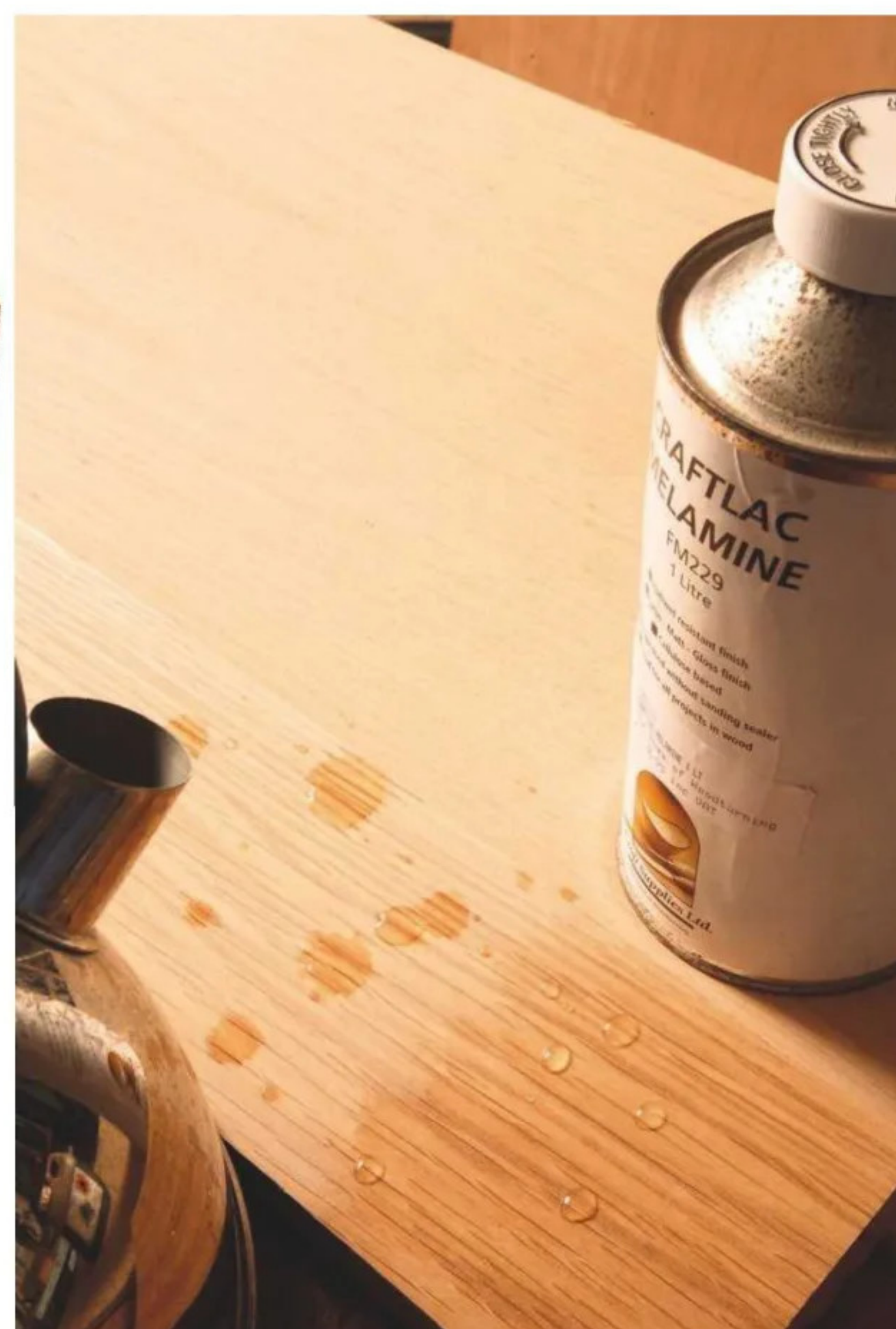
20 Synthetic lacquers, such as melamine, can briefly resist wetness or even boiling water as demonstrated on the bottom corner of this board
