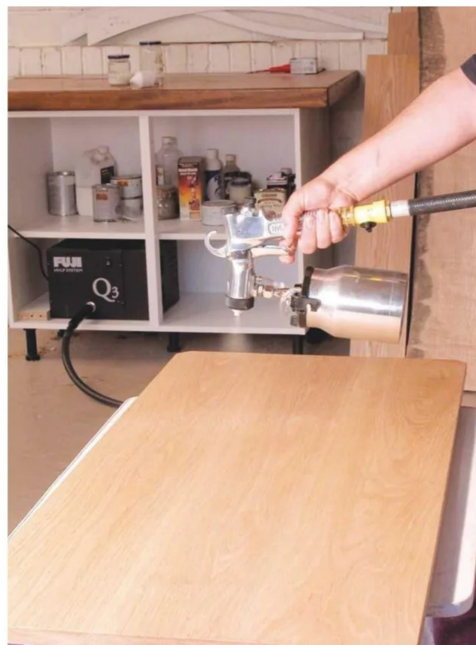
23 For spraying, water-based finishes are best applied with a high volume low pressure – HVLP – system, which provides an even coating with relatively large water droplets
