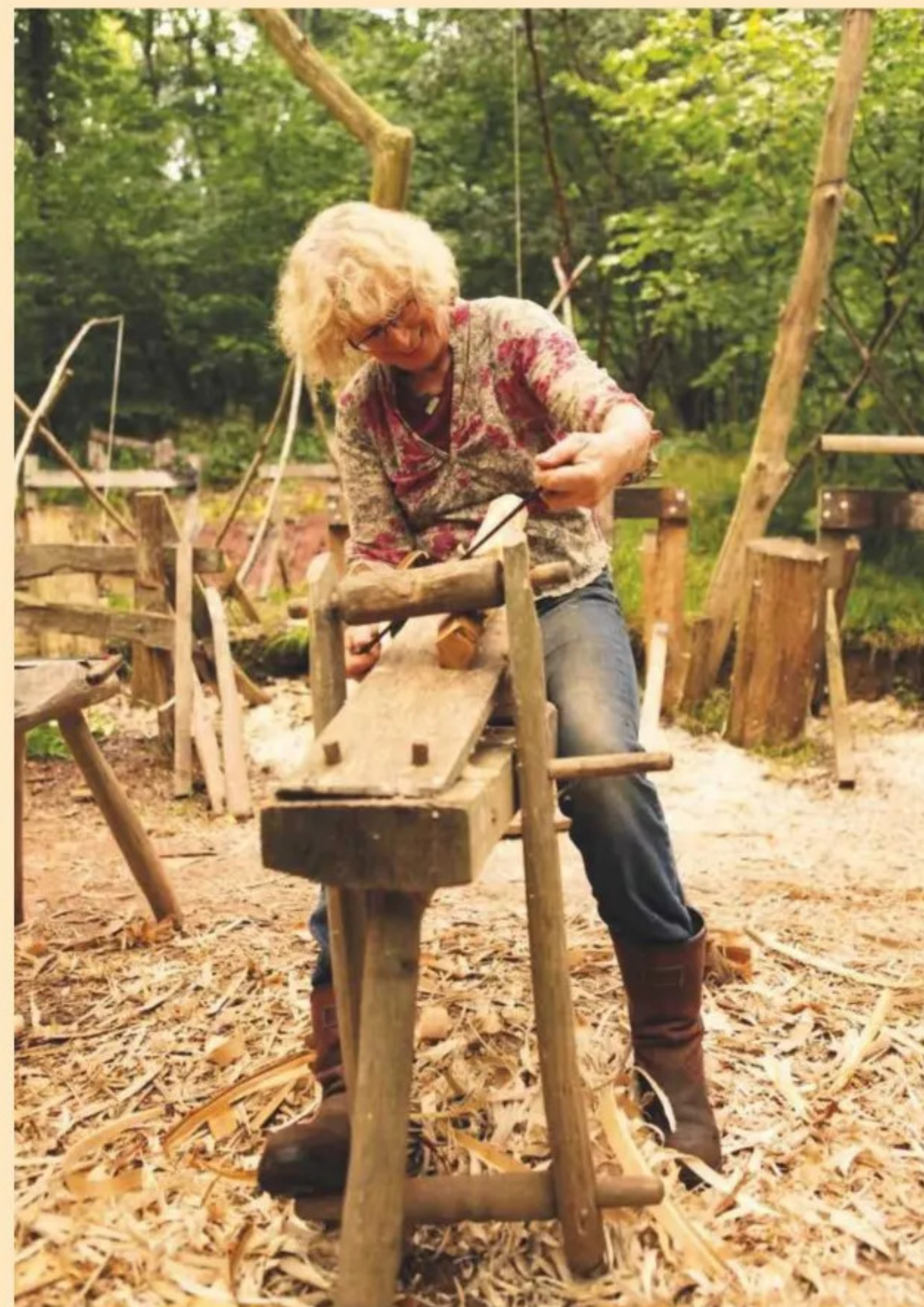
Drawkniving on the shavehorse – getting the stock as near round as possible, so that it's ready to turn
