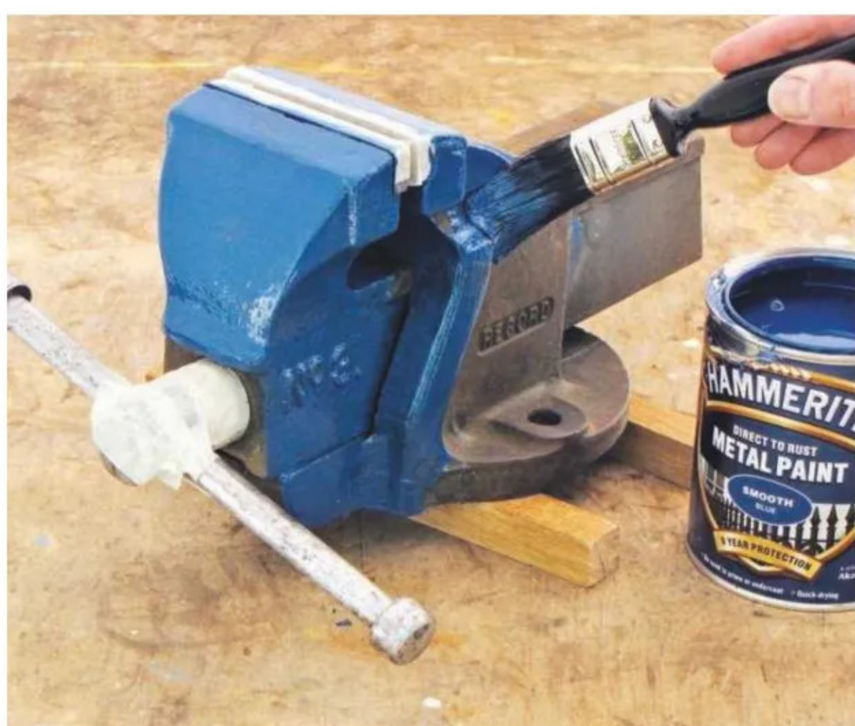
9 Brush on two coats of Hammerite – no primer or undercoat required here; wrap bristles in cling film after painting
