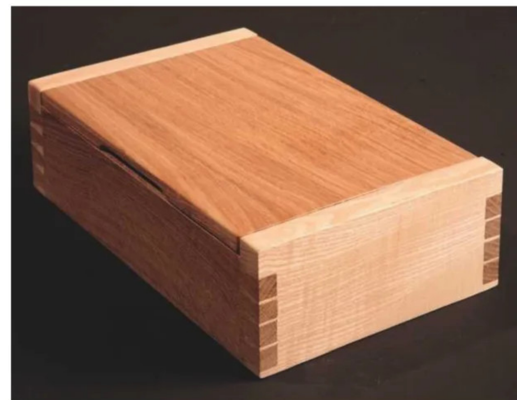
16 In place of wax, using petroleum jelly brings out the contrasting colours of this Welsh ash and oak box while producing a lustrous matt finish
