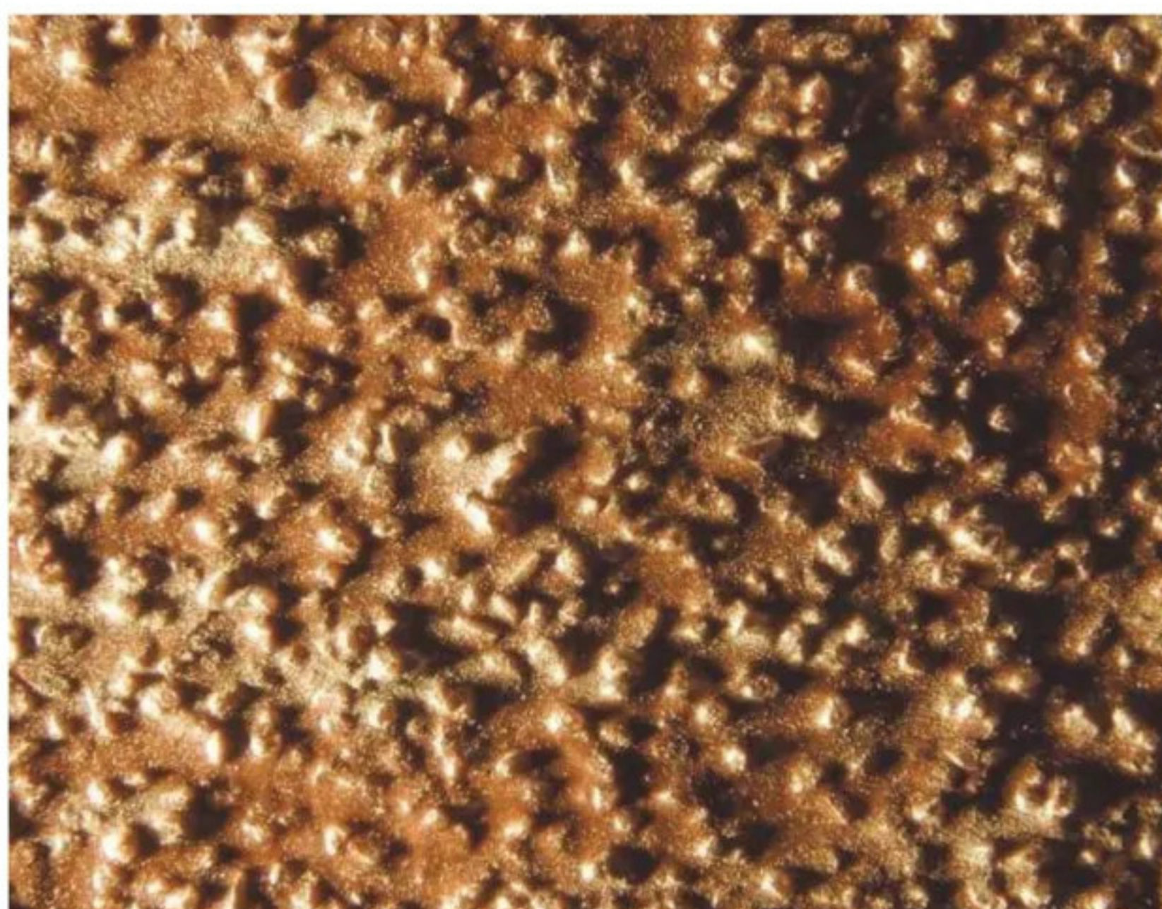
4 Commonly known as 'sandpaper' seen here with a large magnification, abrasive sheets have a layer of wood-cutting grit glued to the surface
