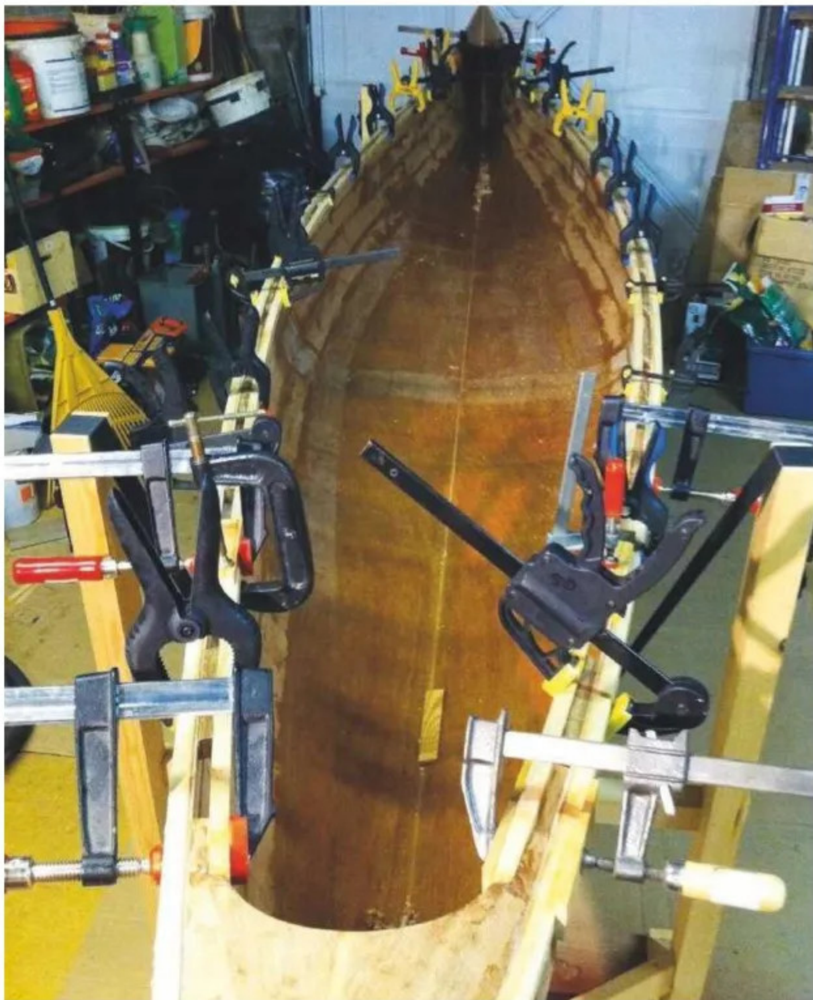
13 Holding the gunnel strips and decking in place requires an extraordinary number of clamps!
