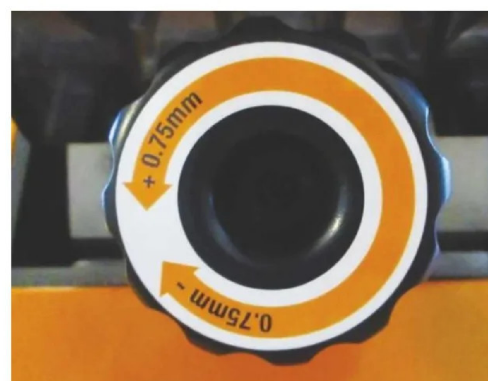
Infed adjustment shows the approximate adjustment distance
