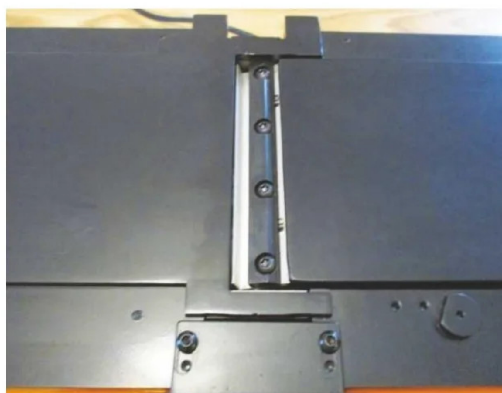
The exposed blade drum needs a guard!
