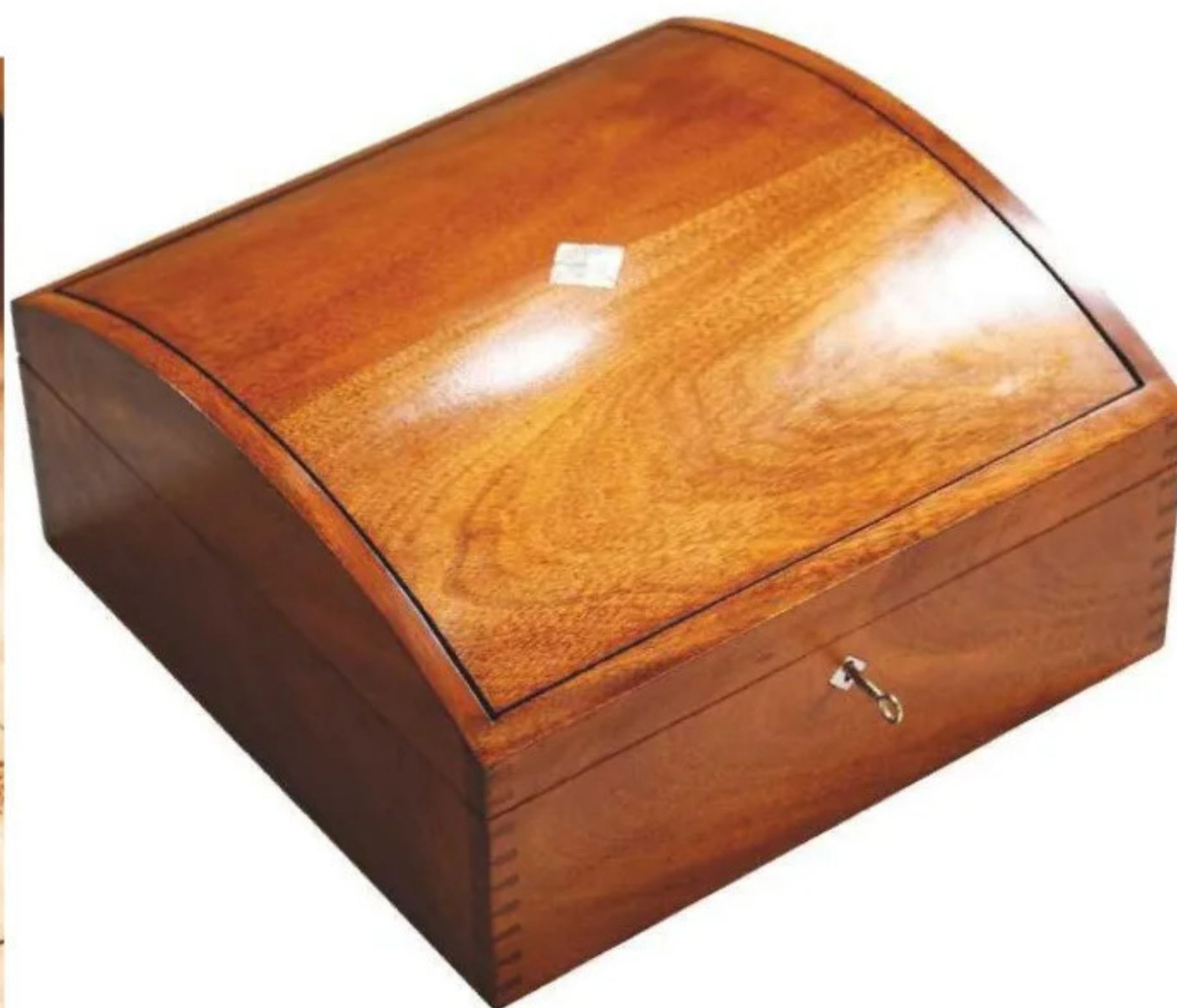
19 To prevent shellac taking on too high a gloss, it can be rubbed with waxed fine steel wool
