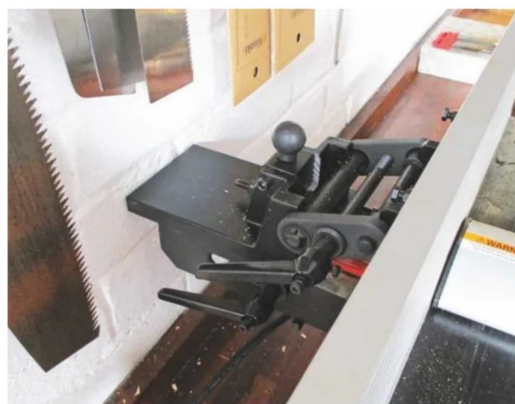
Fence adjustment prevents use up against a wall
