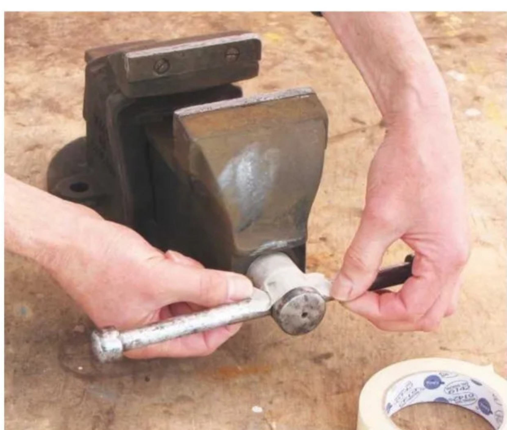
8 Dust and dry thoroughly, using a heat gun if necessary; mask off the handle and jaws before you begin painting
