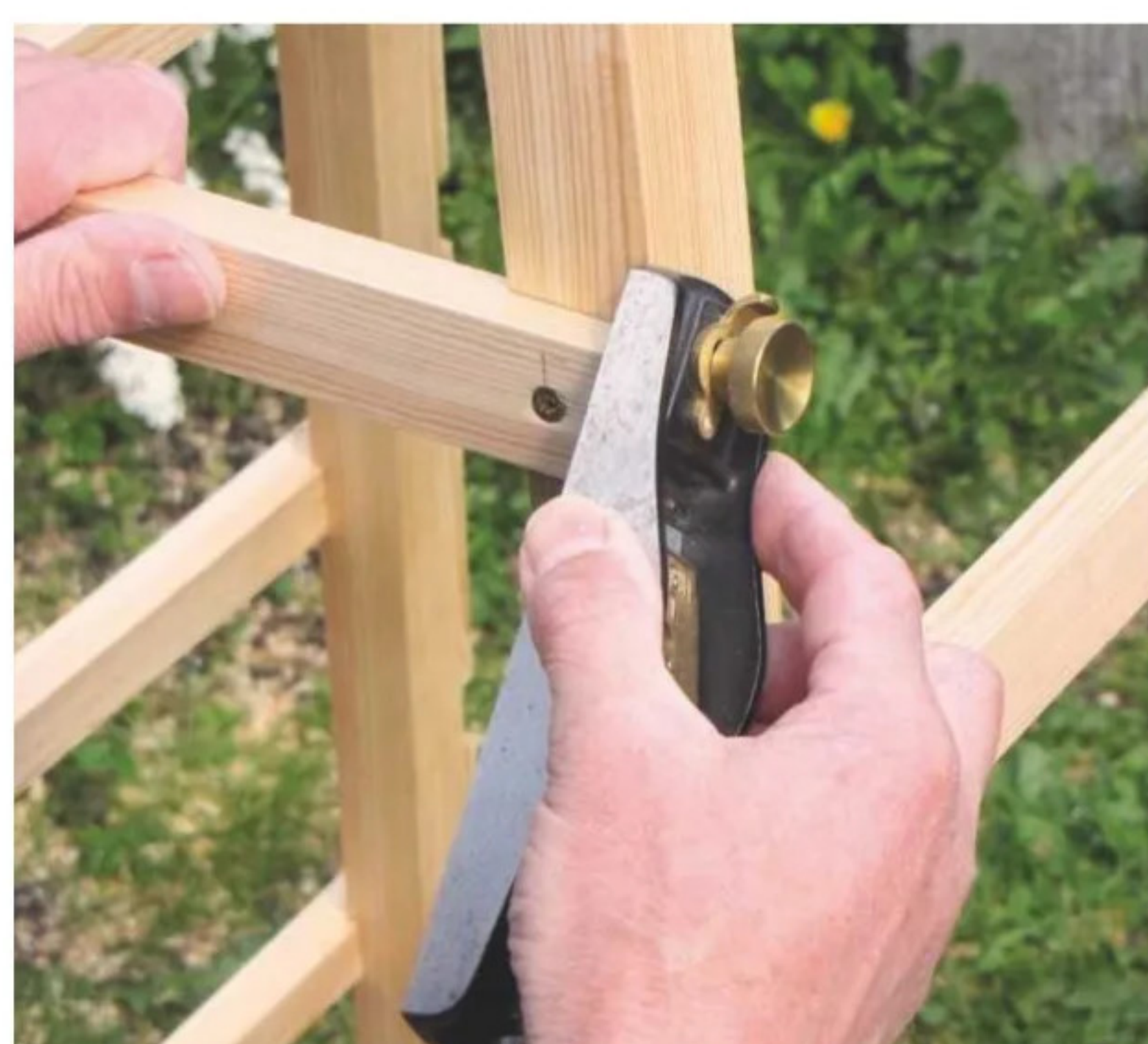
15 Using a block plane, trim ends that may be slightly proud, then sand the edges so they're ready for finishing
