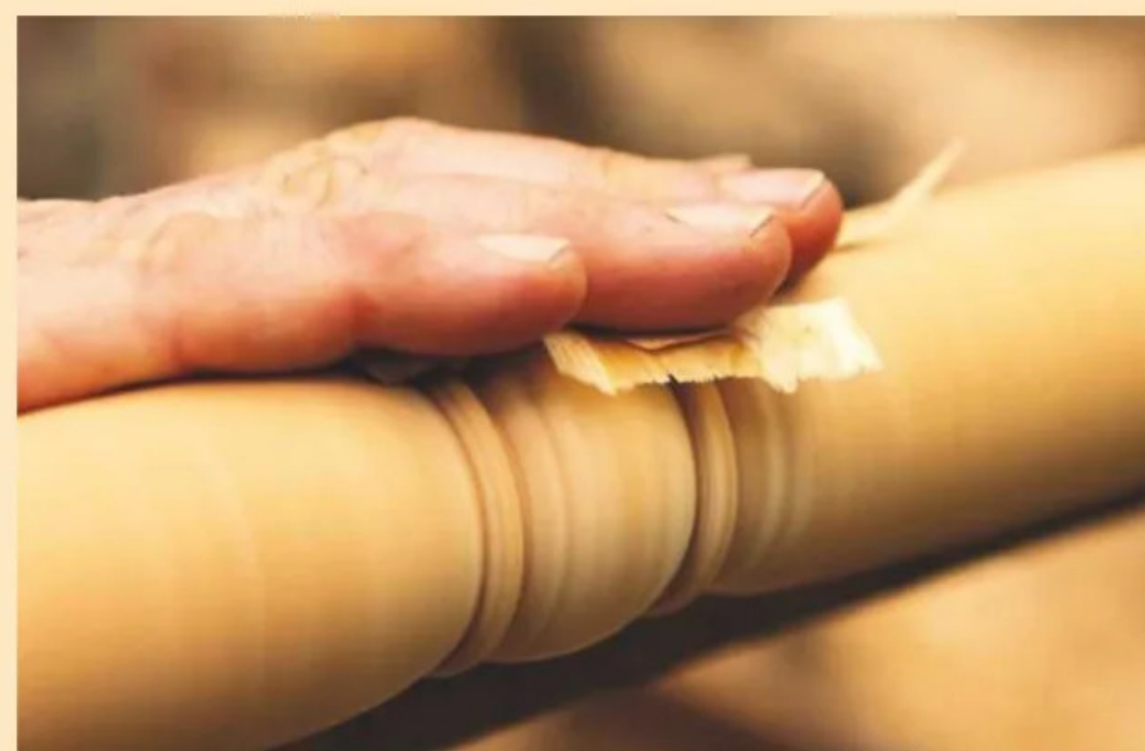
A handful of shavings is used to burnish and smooth
