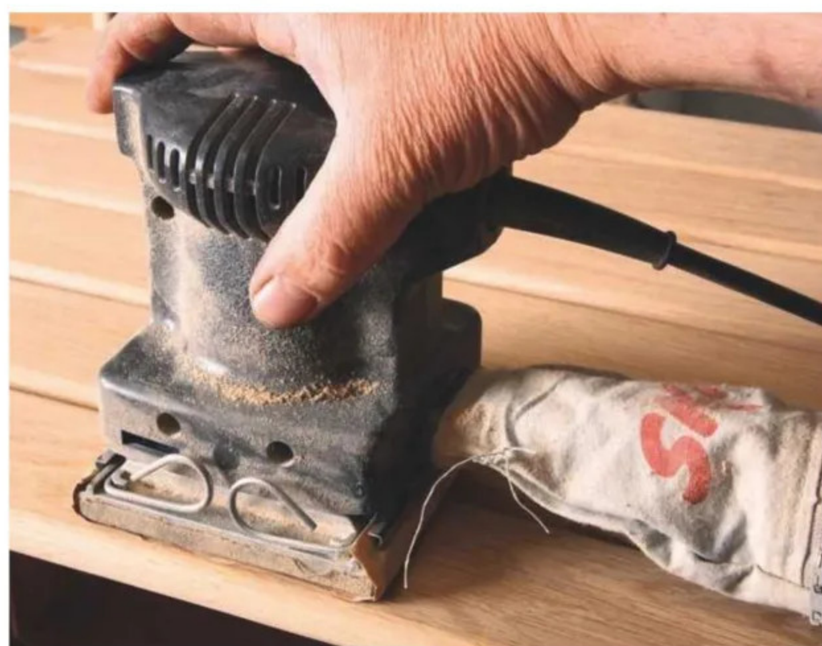
6 A small hand-held sander produces spiral tracks on the wood's surface. The paper oscillates in a circular motion while the tool is swept across it
