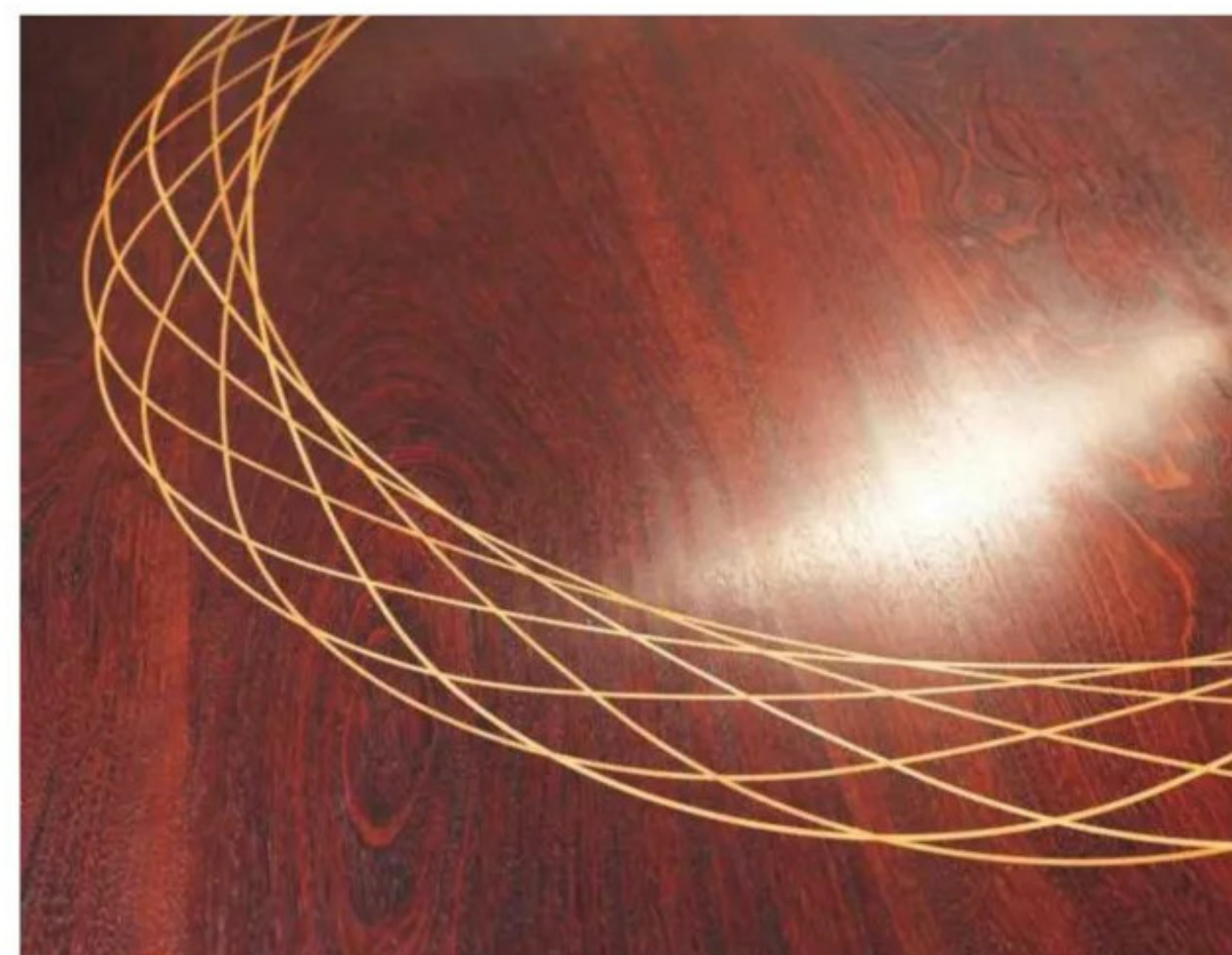
24 A clear fine semi-matt finish that doesn't clog up the grain brings out the best wood figuring and decoration
