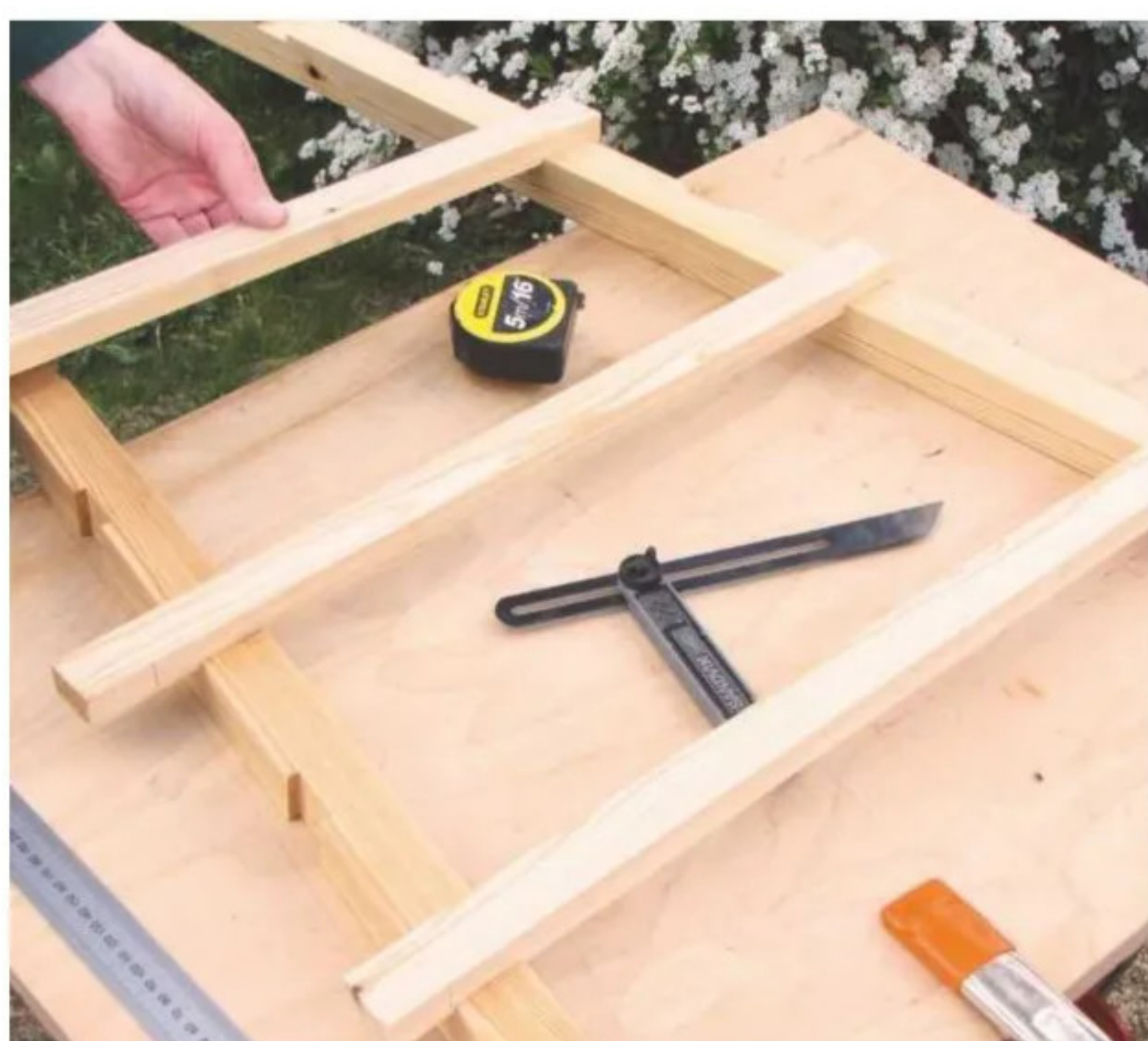
11 Cramp a pair of legs to the bench so they meet at the top. You can then mark the length of each rail in turn
