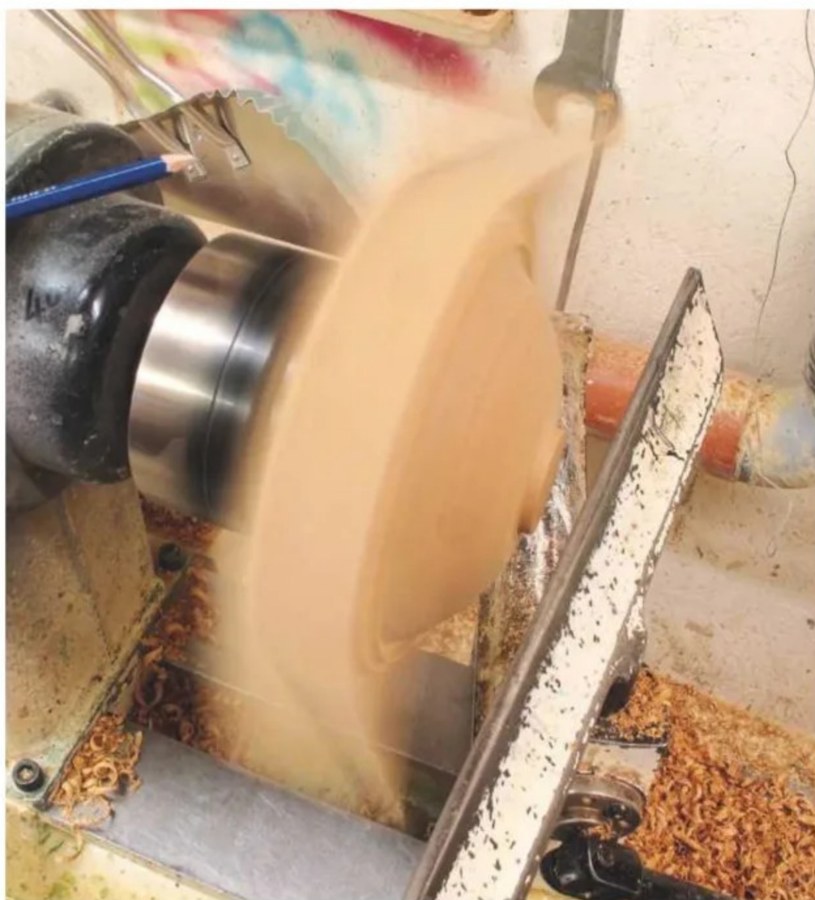
10 Drawing a thick line – as I've done here – allows you to see it as the lathe spins. To produce the desired shape, the tool's bevel needs to follow this line around
