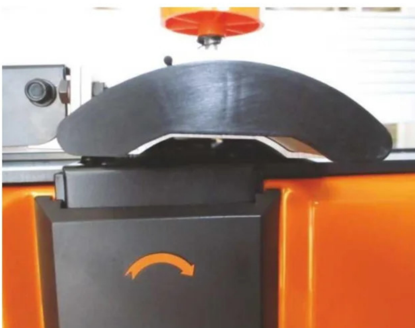
The guard doesn't sit centrally over the drum
