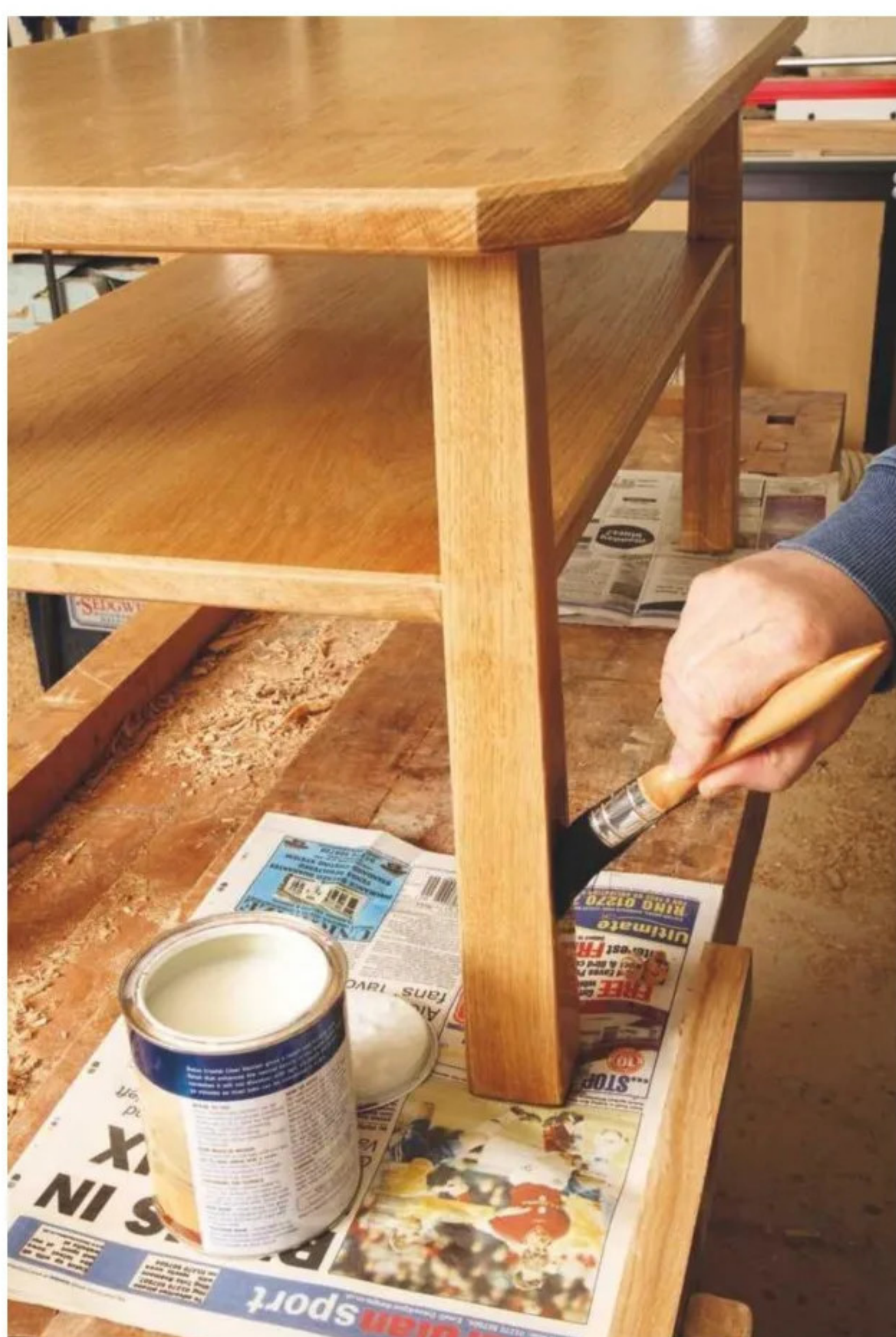
21 Water-borne varnishes use small amounts of solvent – low VOC – by suspending the varnish as a fine emulsion in water
