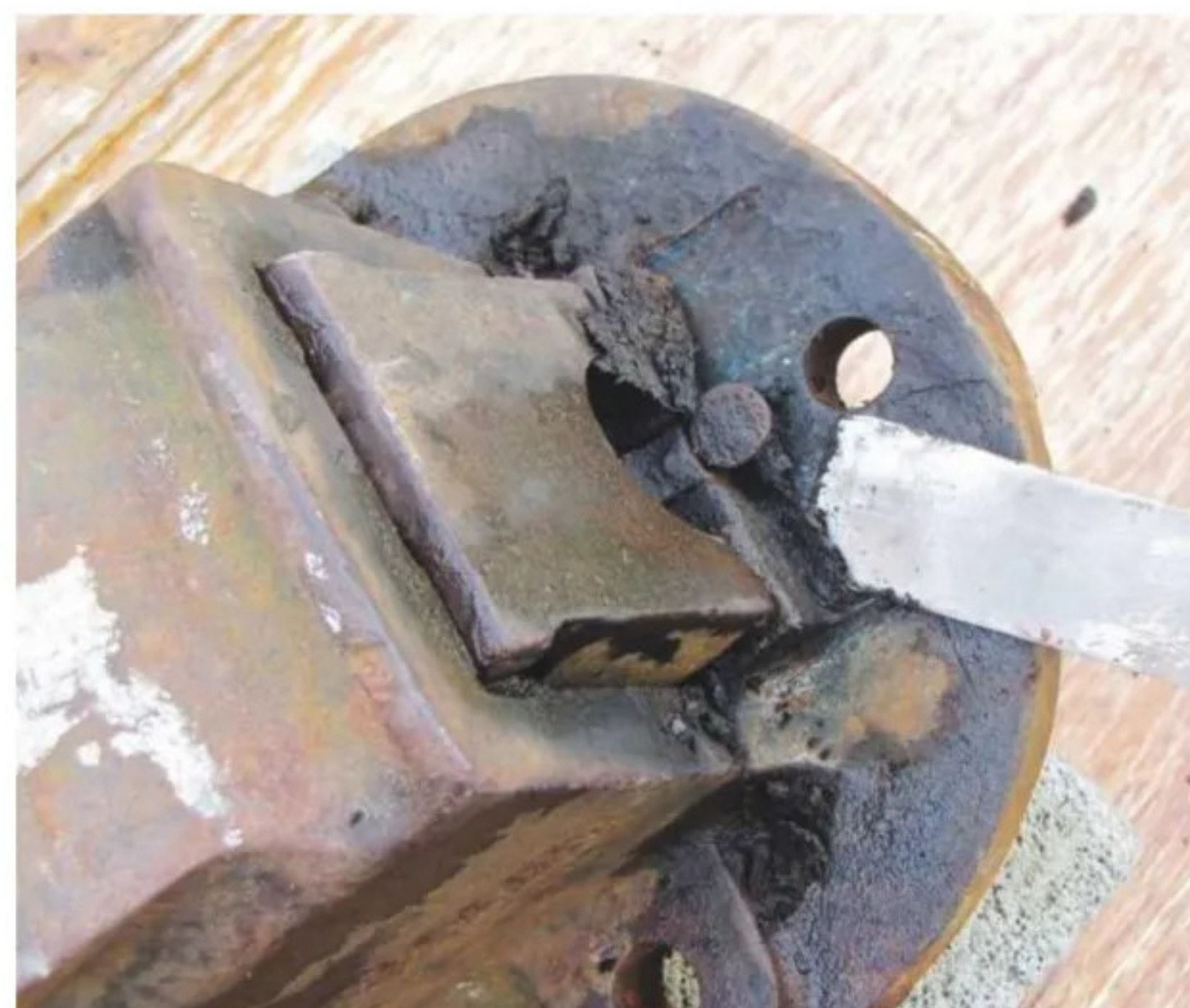
2 Scraping off congealed material and loose rust before using Restore solution to help the process
