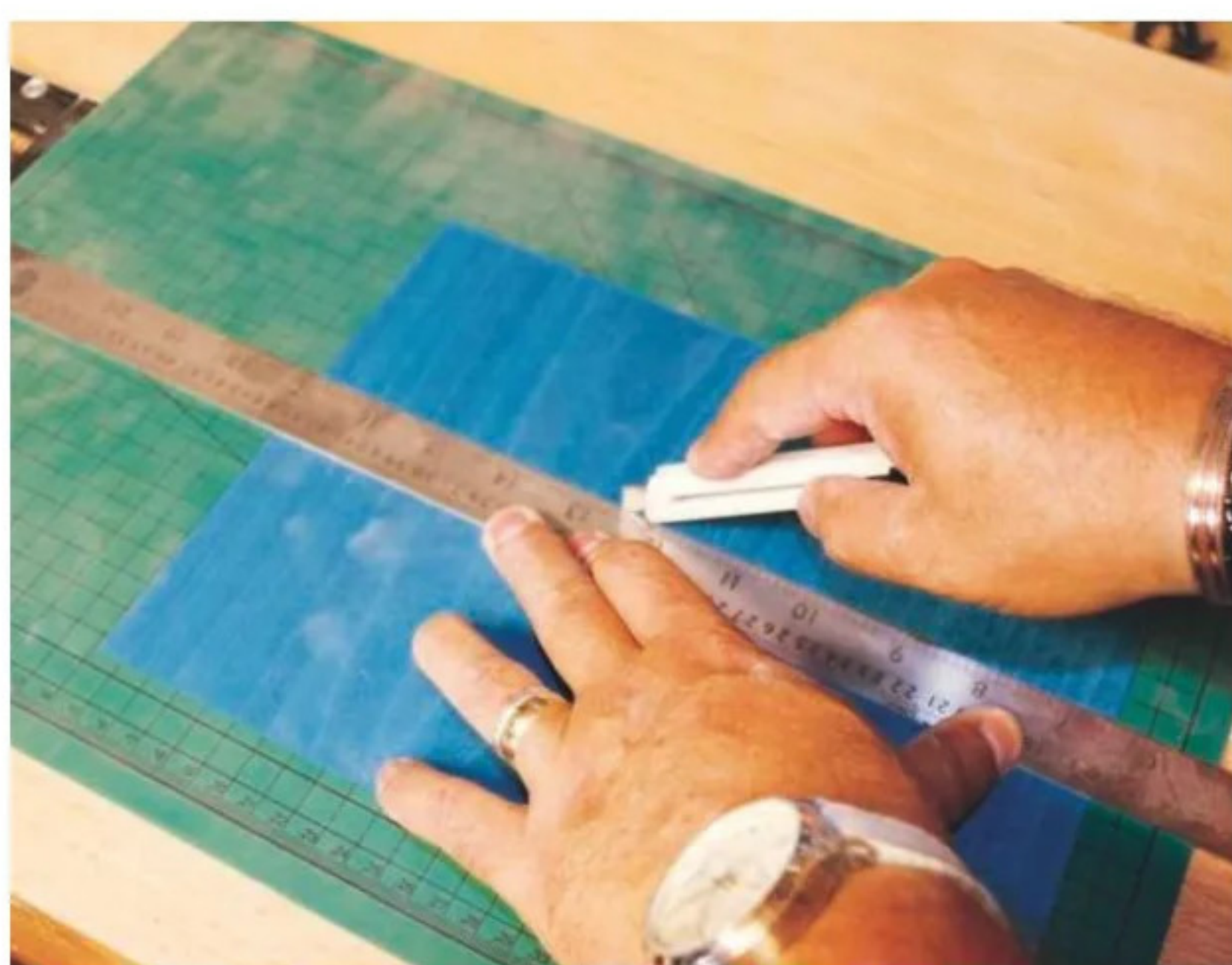
The veneers cut easily with the aid of a sharp knife and straightedge
