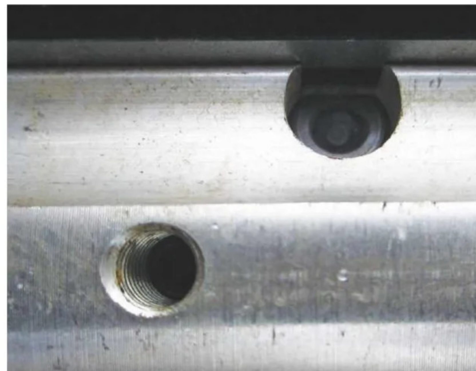
Blade adjustment screws are easy to access
