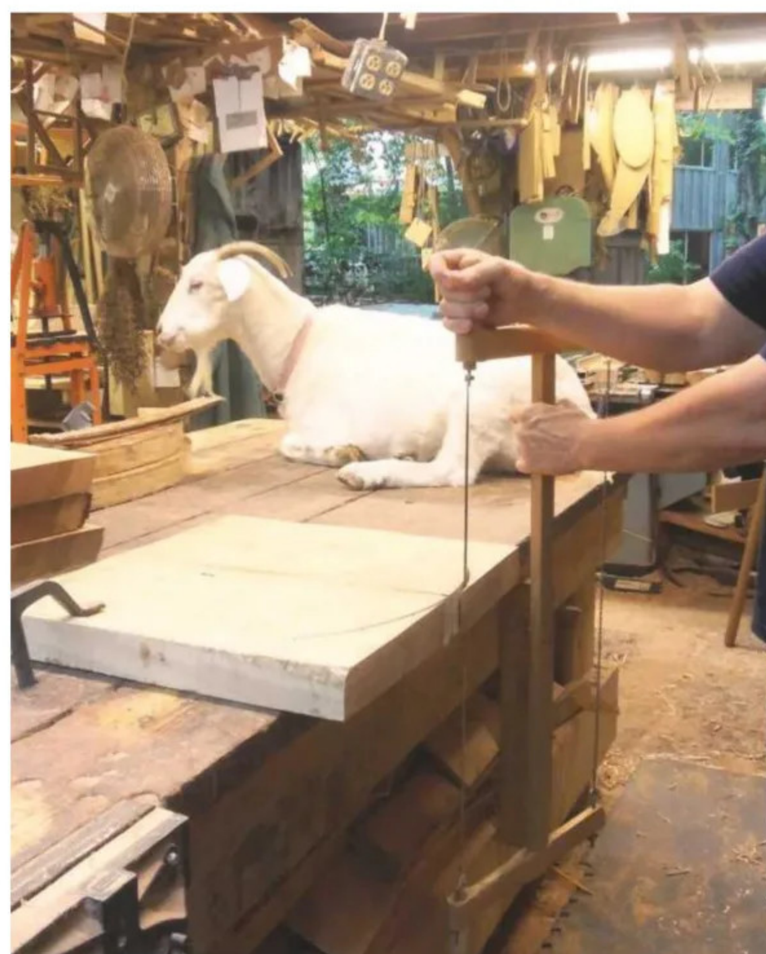
2 Frame sawing a seat out of 50mm curly maple
