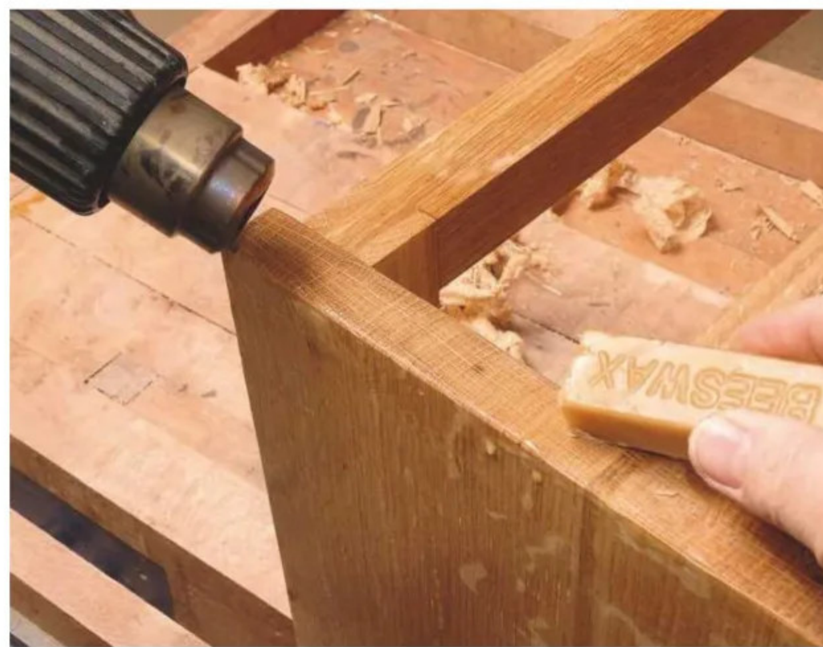
12 Warming the wood with a hot air blower allows the wax to soak deep into the end-grain as well as saturating between wood fibres
