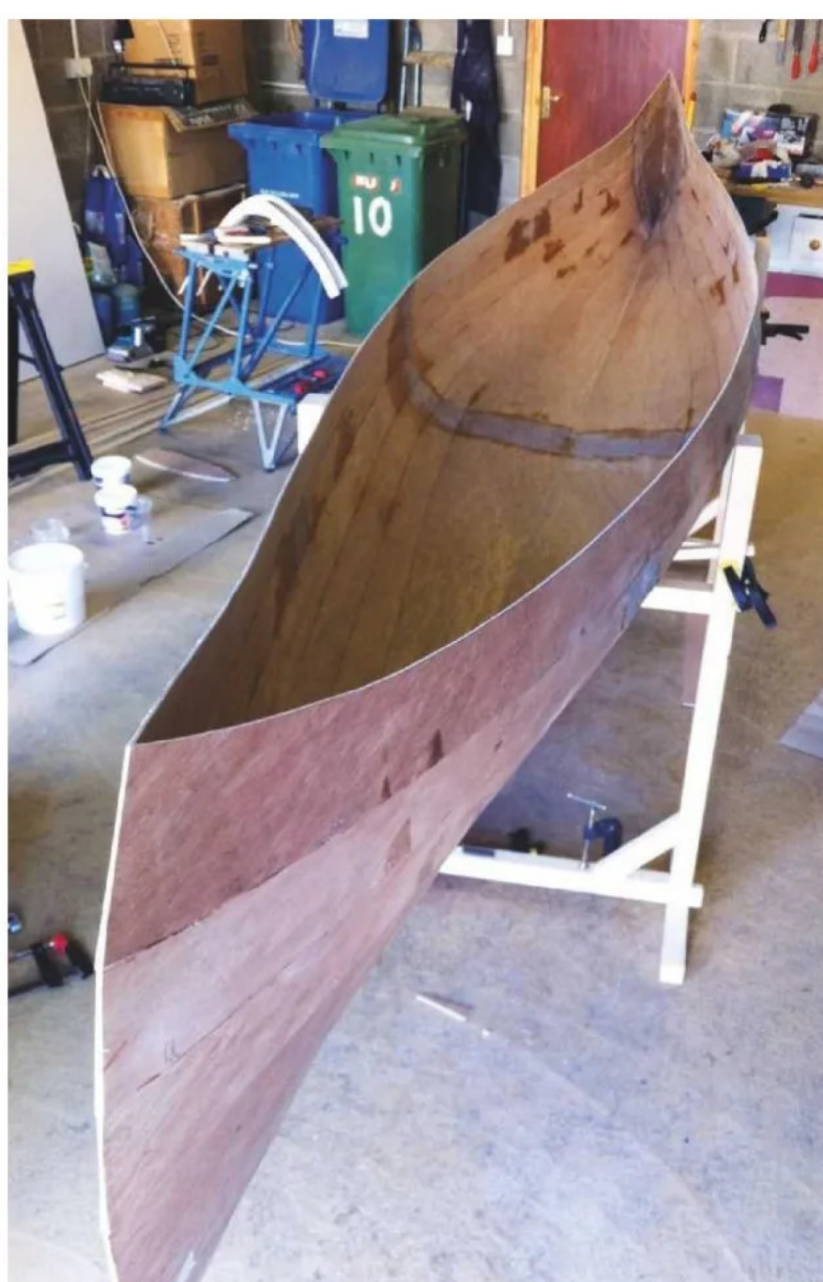
10 After the epoxy had gone off, the copper wire could then be removed
