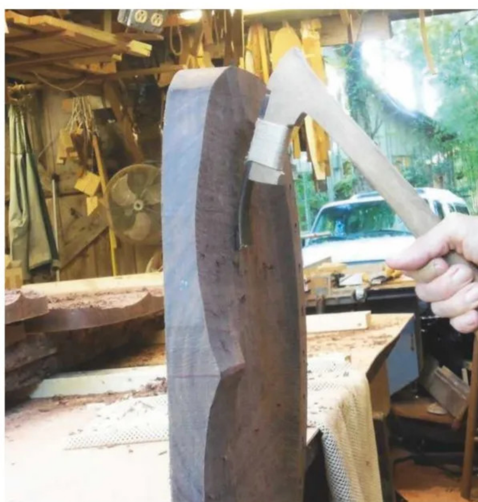
5 Adzing a chair seat using a blade from the Pacific Northwest Natives
