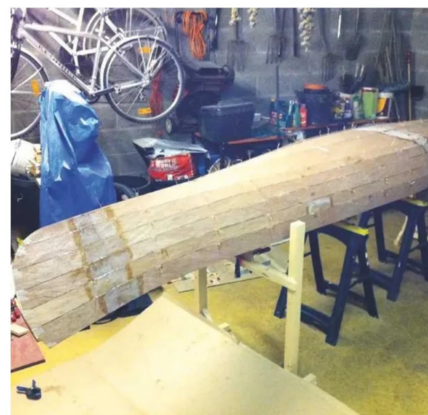
9 ... which turned out to be a frantic process that involved having to re-tie and apply more wire
