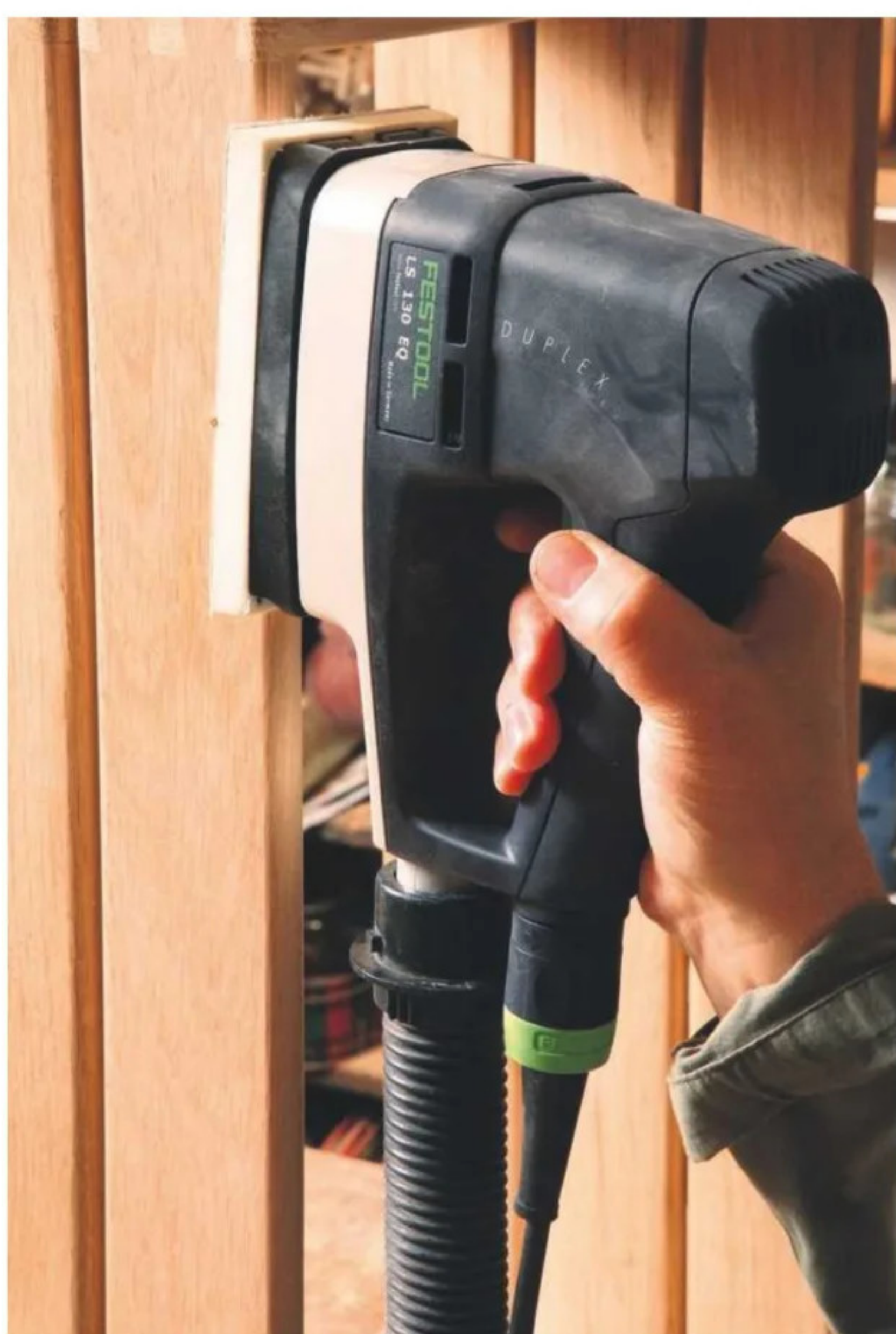
8 A linear sander is ideal for following the wood grain pattern, especially on edges
