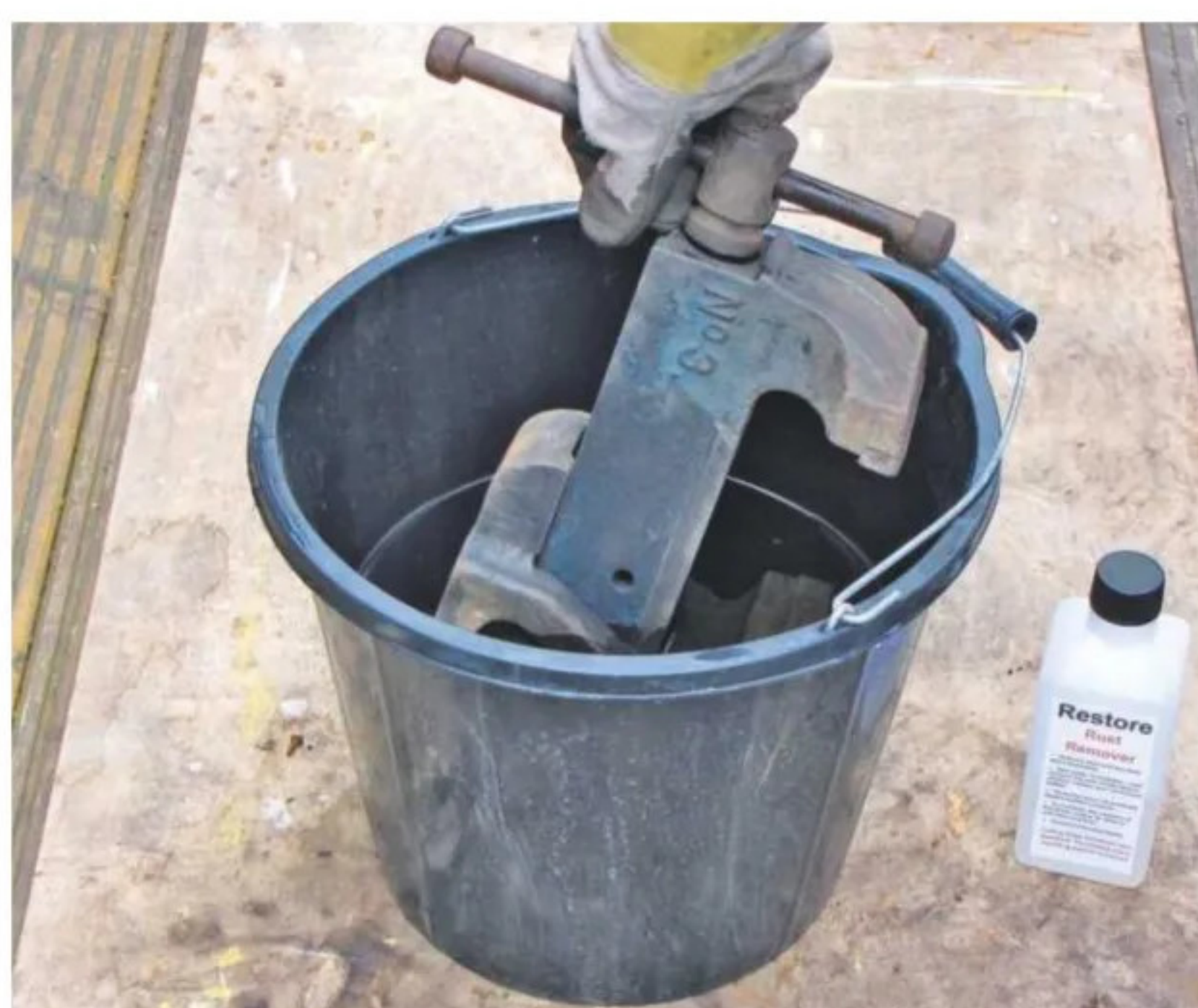
4 Dip the vice in a suitable container of Restore Rust Remover, turning end on end if not fully immersed
