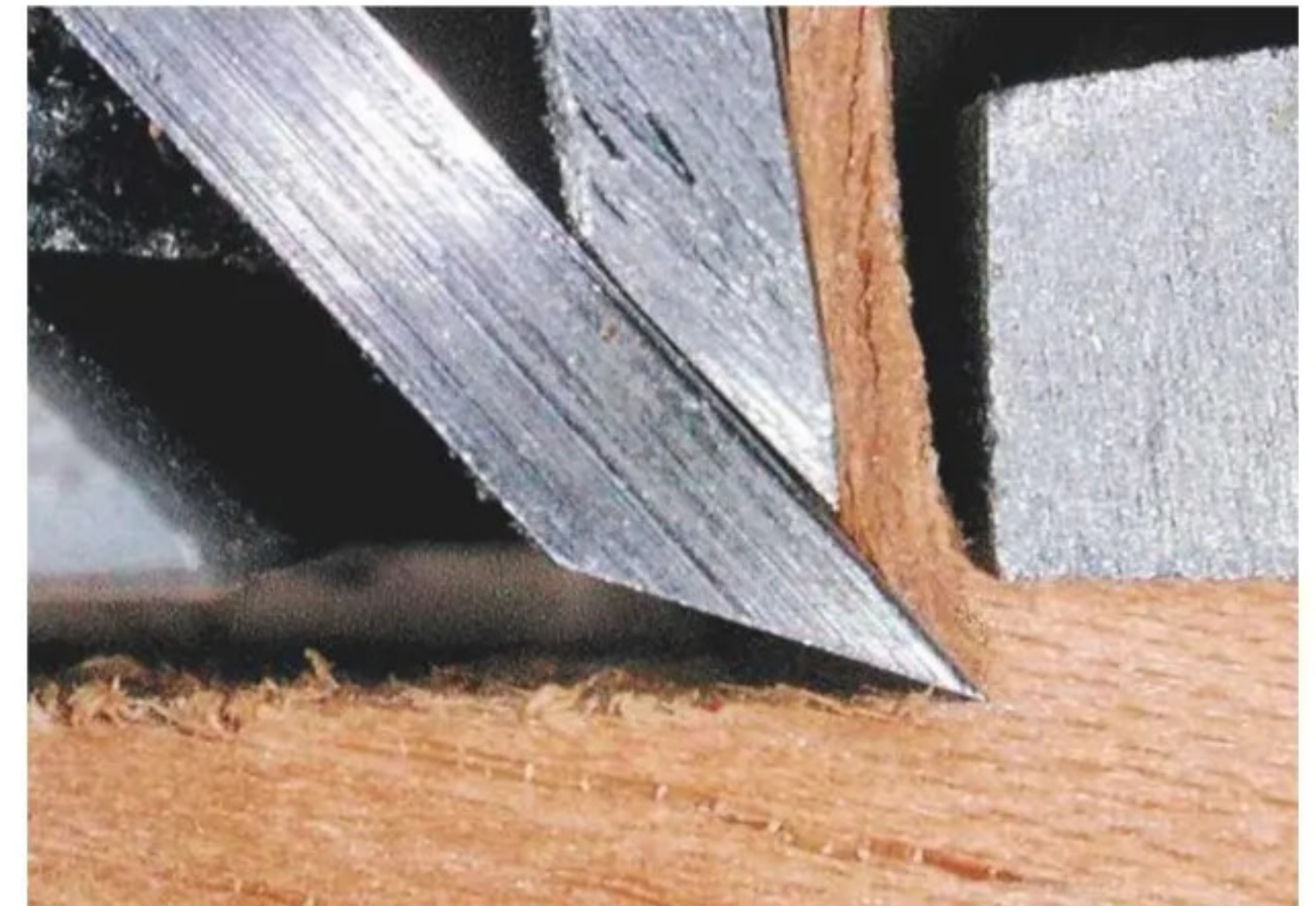
5 Planing against the grain, using a cap iron and fine shaving aperture
