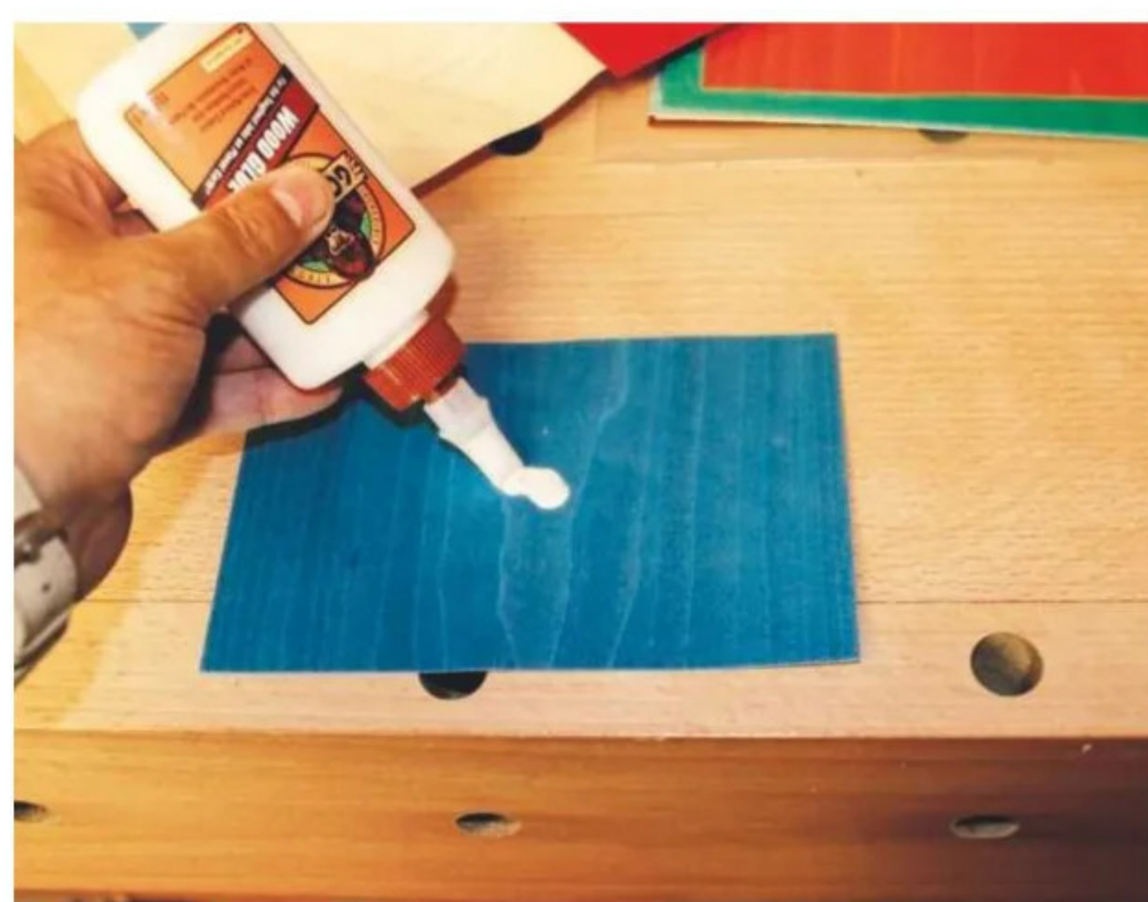
Apply PVA glue and spread thinly over the entire surface area
