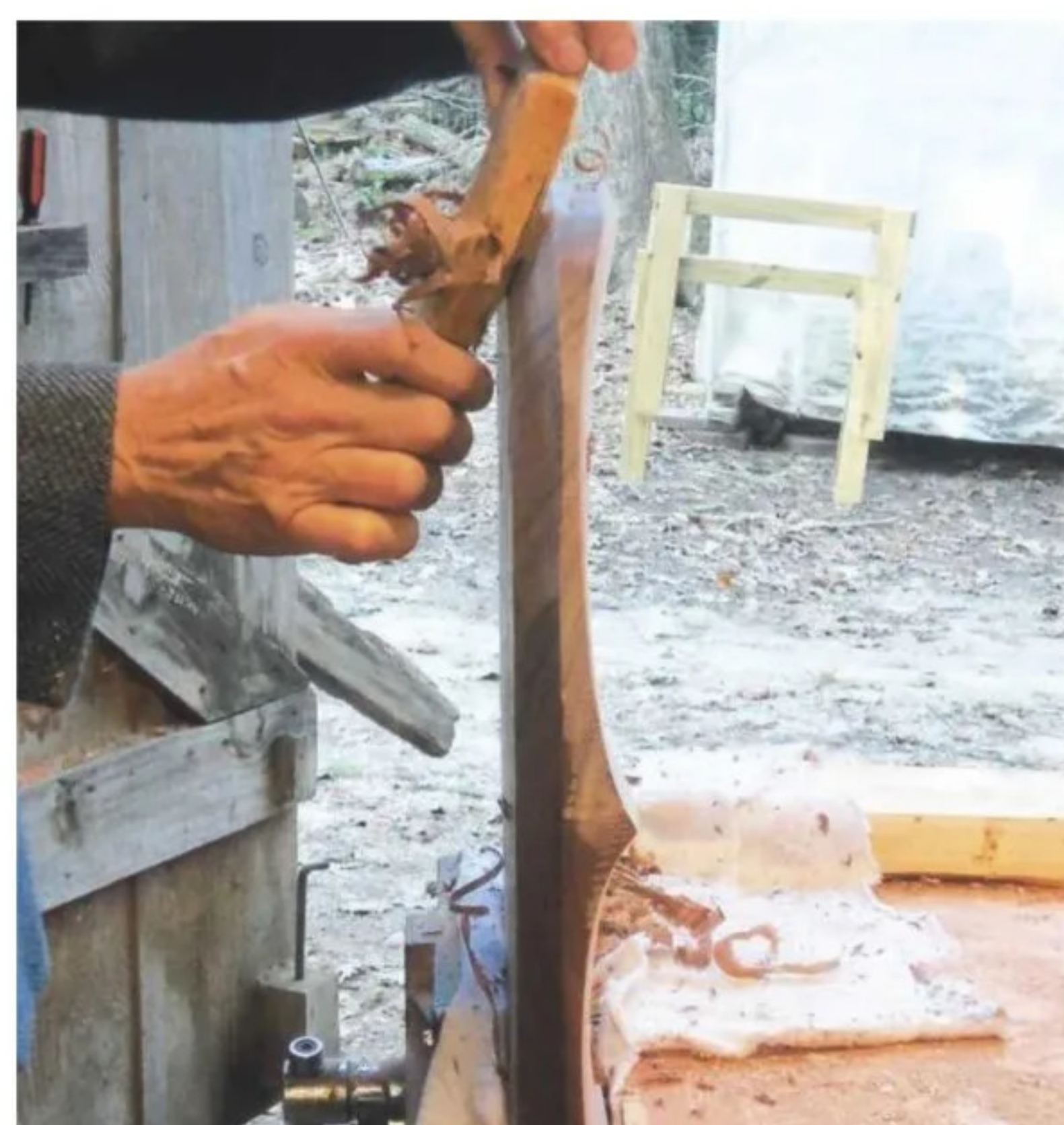
6 Bevelling the seat with a wooden spokeshave
