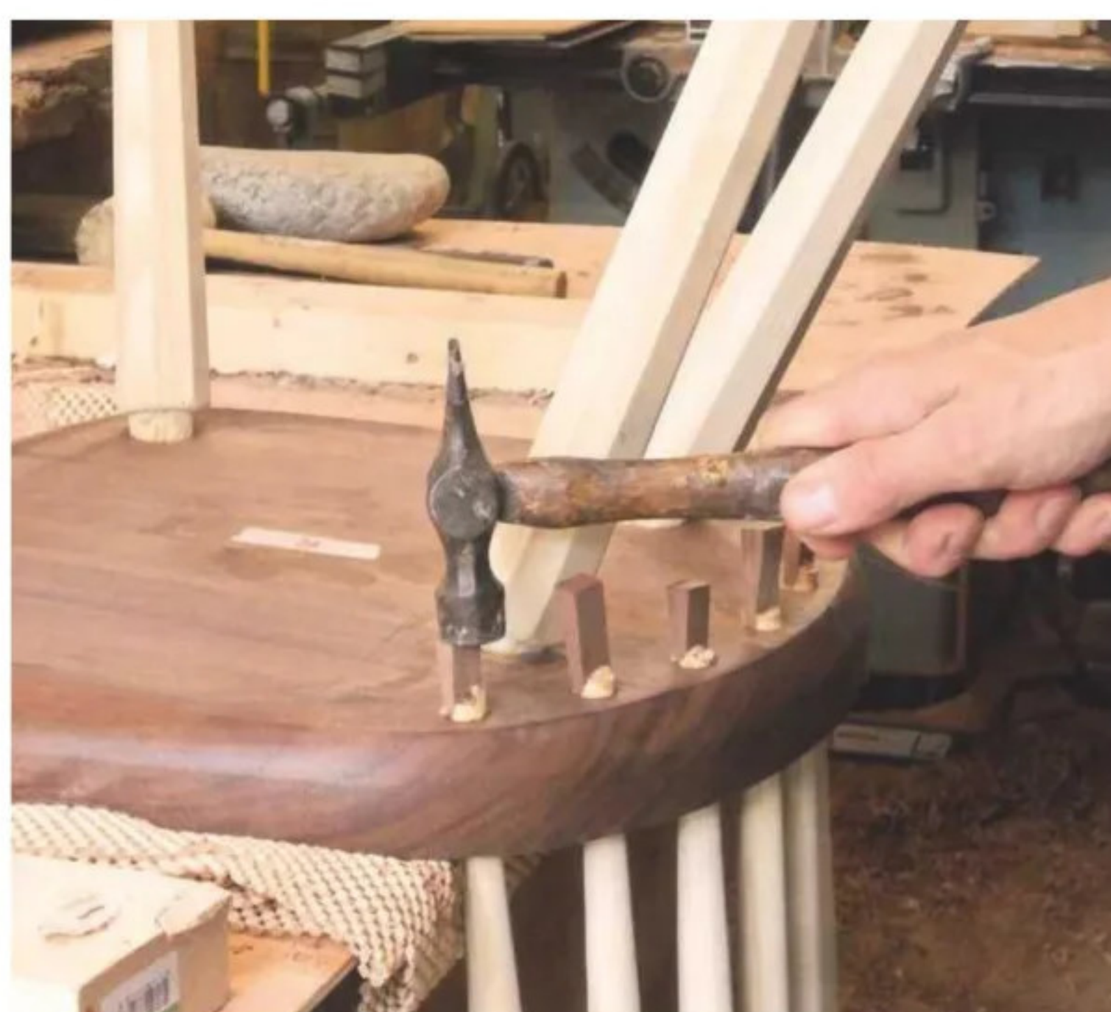
7 Wedging spindles and driving in walnut wedges
