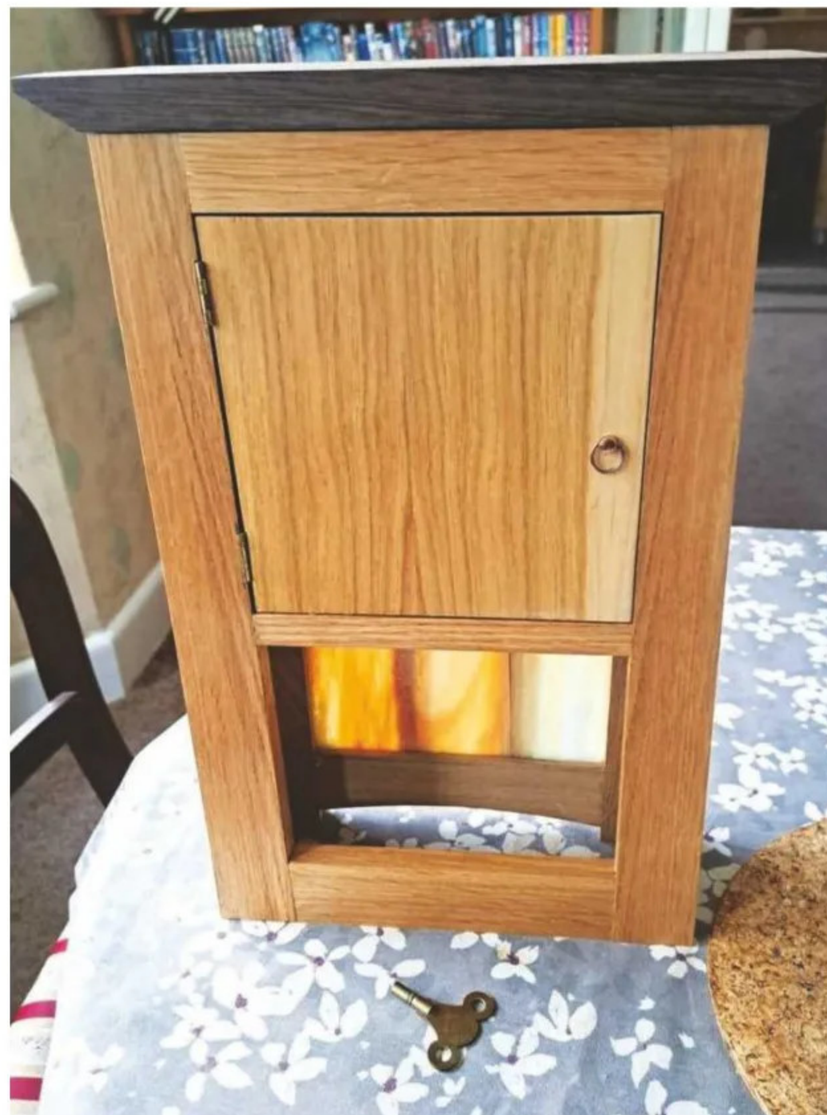
10 The access door for the chimes was made from veneered plywood, fitted in place with small brass hinges
