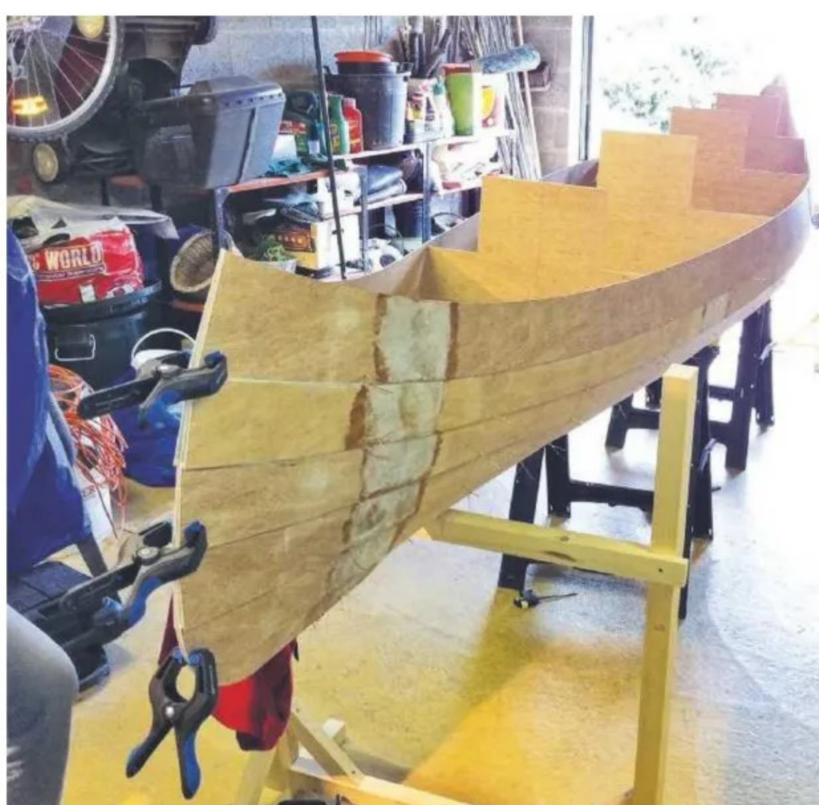
8 The panels were stitched together with copper wire and epoxy...
