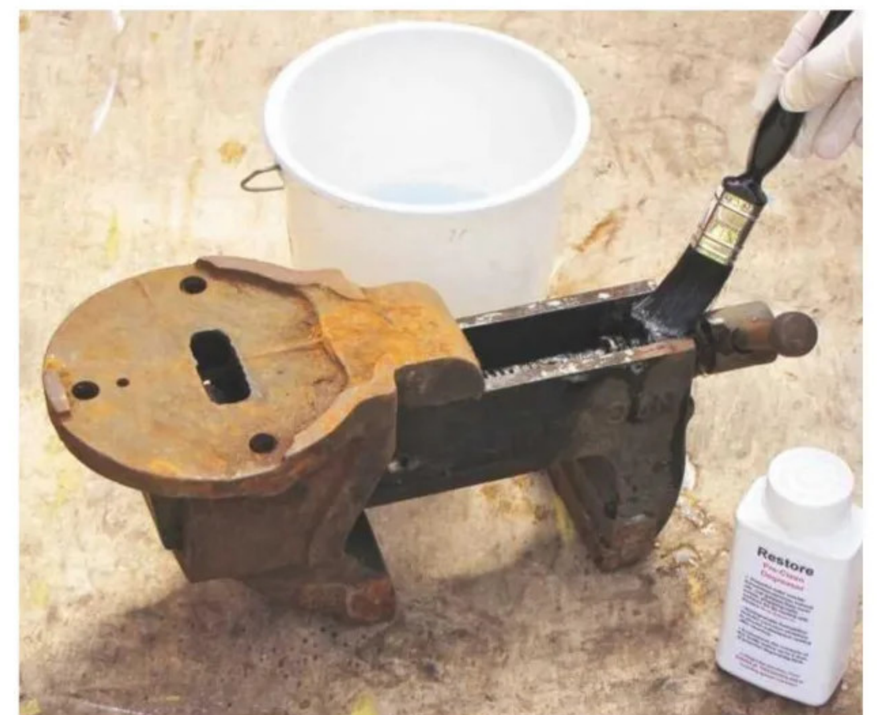
3 Liberally brush on diluted Pre-Clean Degreaser to remove oil or grease residue; rinse with hot water
