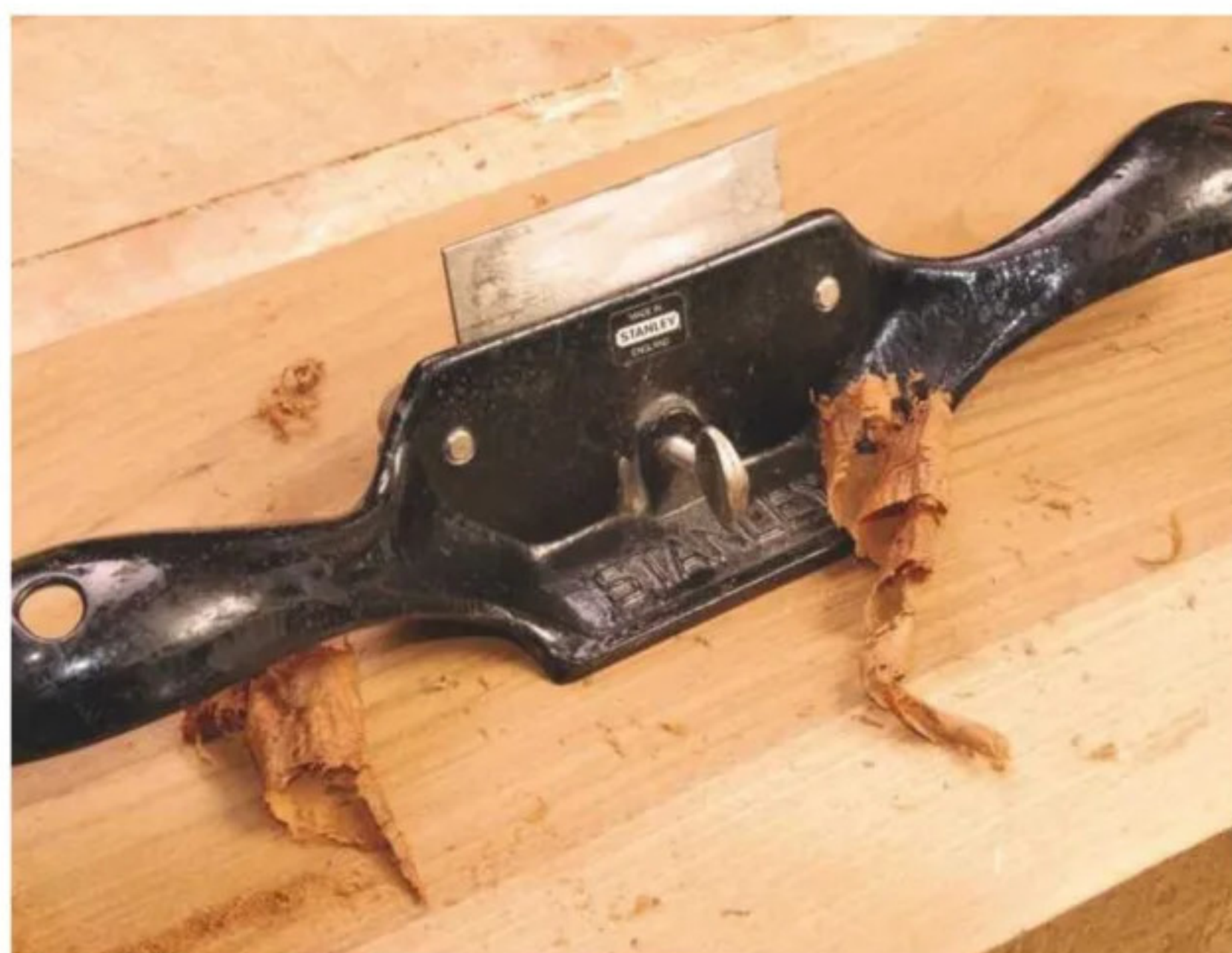
3 One of the most basic tools for flattening a wooden surface is the scraper blade, here mounted in a cast handle to take strain off the thumb
