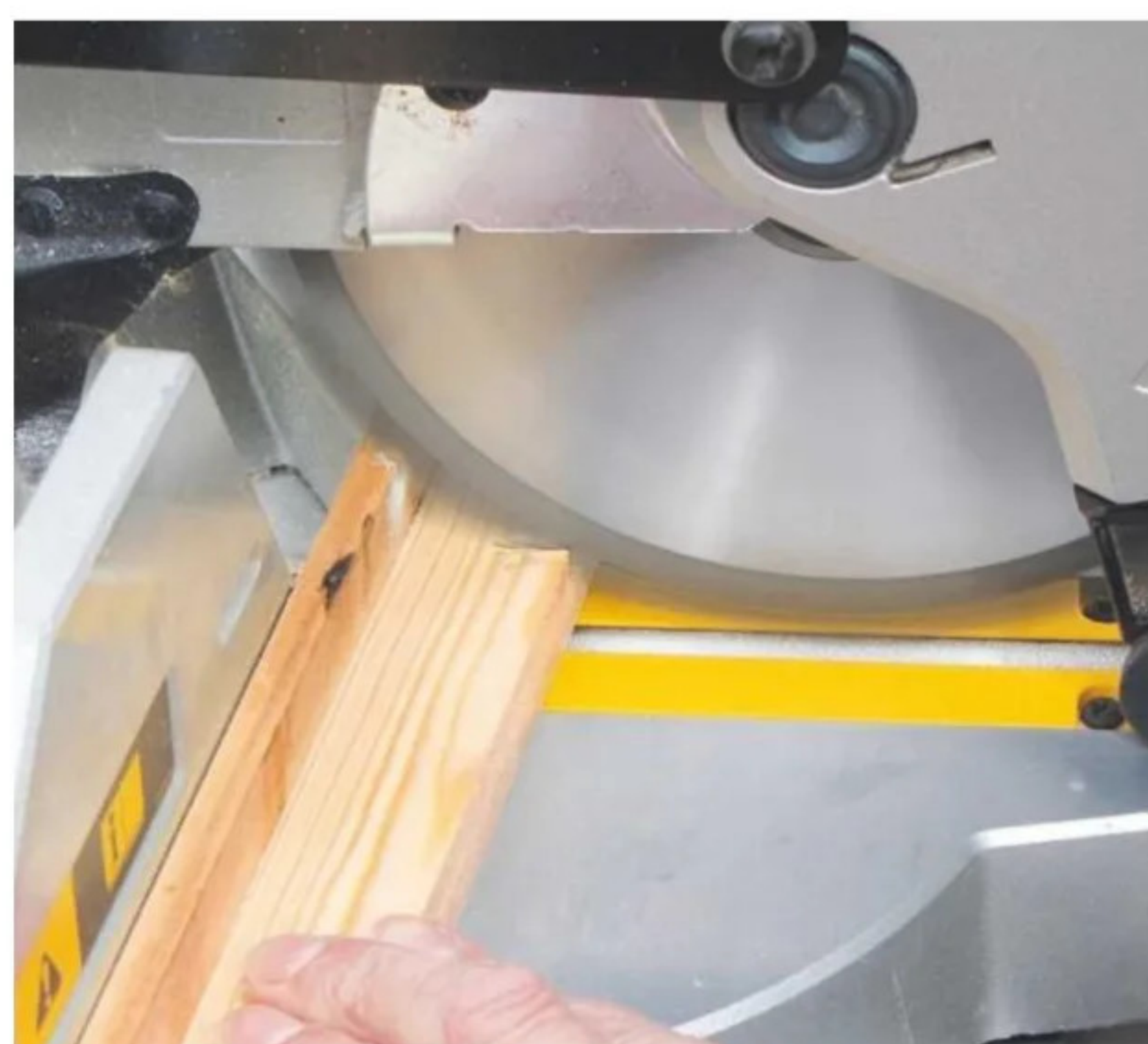
12 Set the mitre saw blade to crosscut at 82°. You can then cut each rail exactly to length
