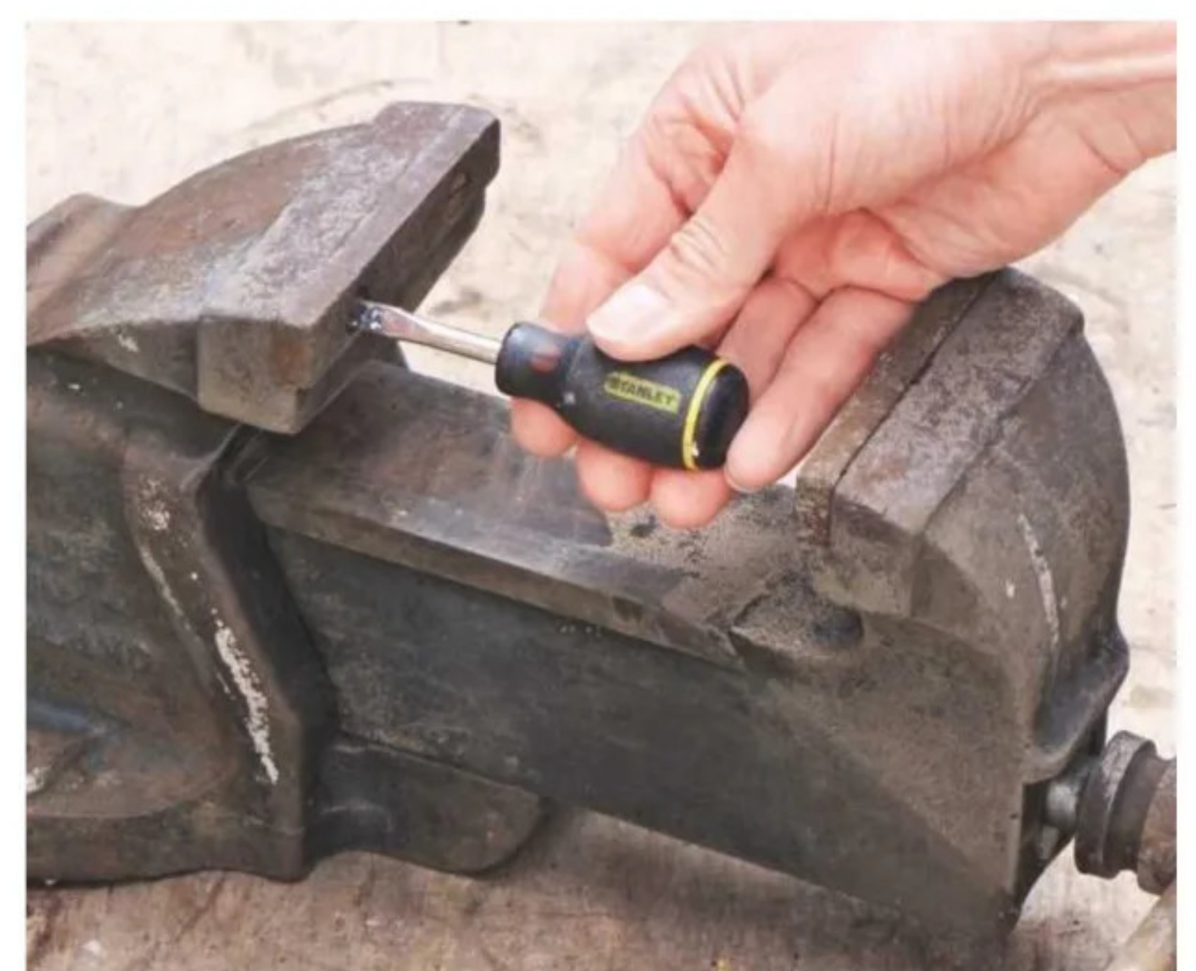
6 Remove jaw facings; if screws are seized, try heat gun or WD40, but you'll need to repeat degreasing
