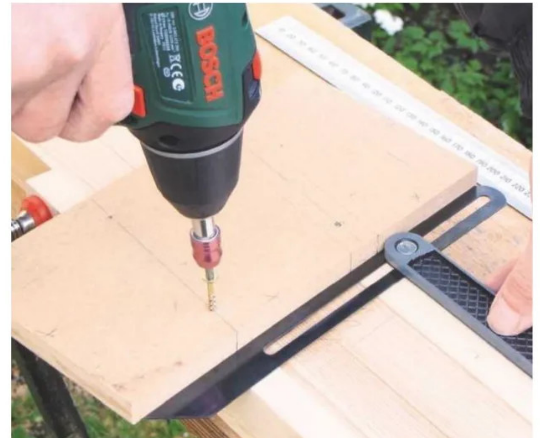
4 To make the jig, screw a piece of MDF to battens placed either side of the legs, checking the angle
