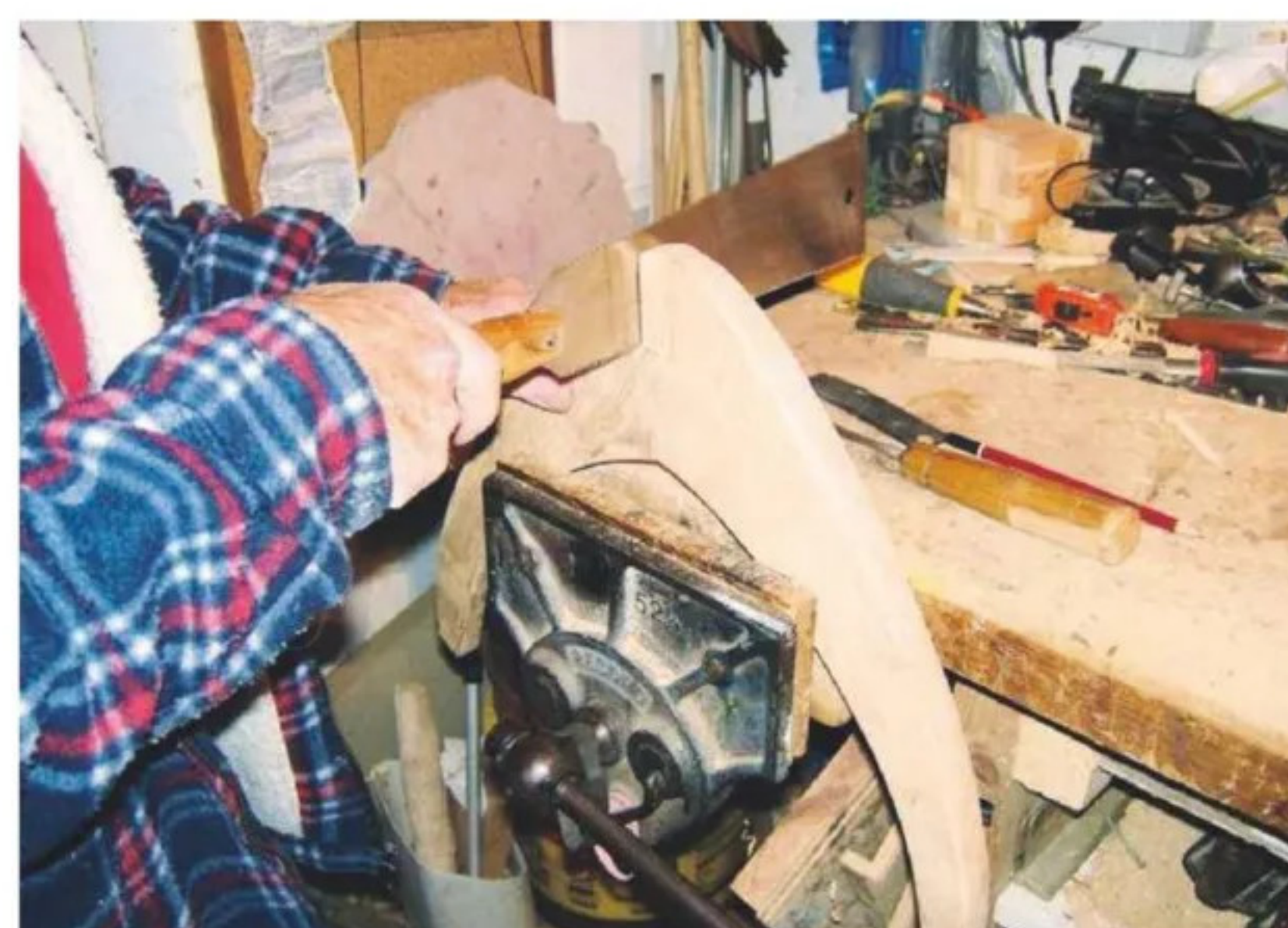
1 Cutting a slot in the base...
