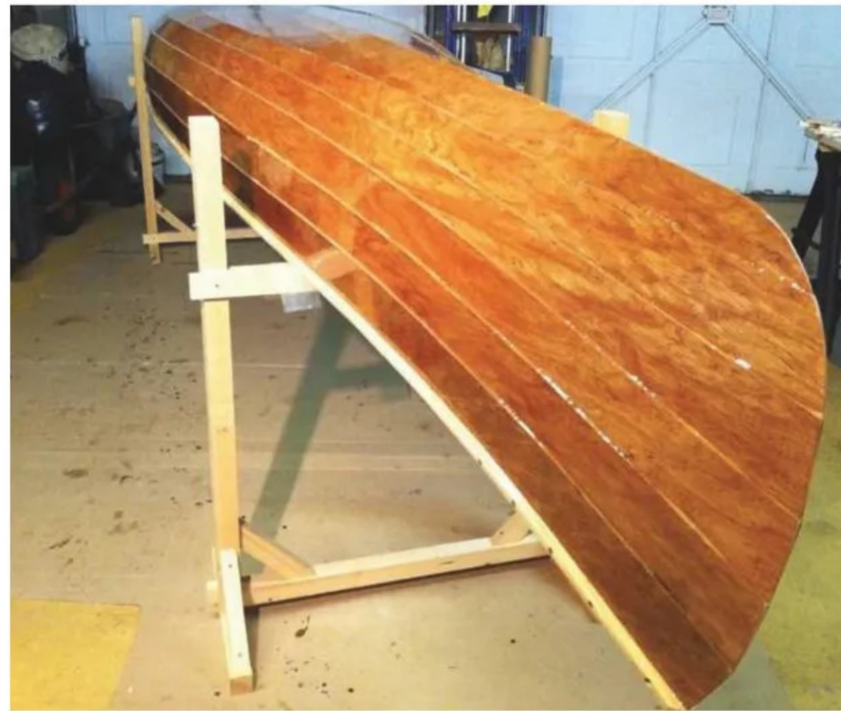
14 Finally, the canoe exterior could be epoxied – just look at that lustre!
