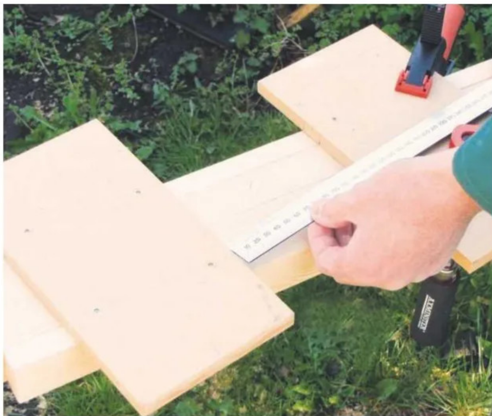
5 Fix the second piece of MDF so that your chosen router bit cuts the exact housing width required
