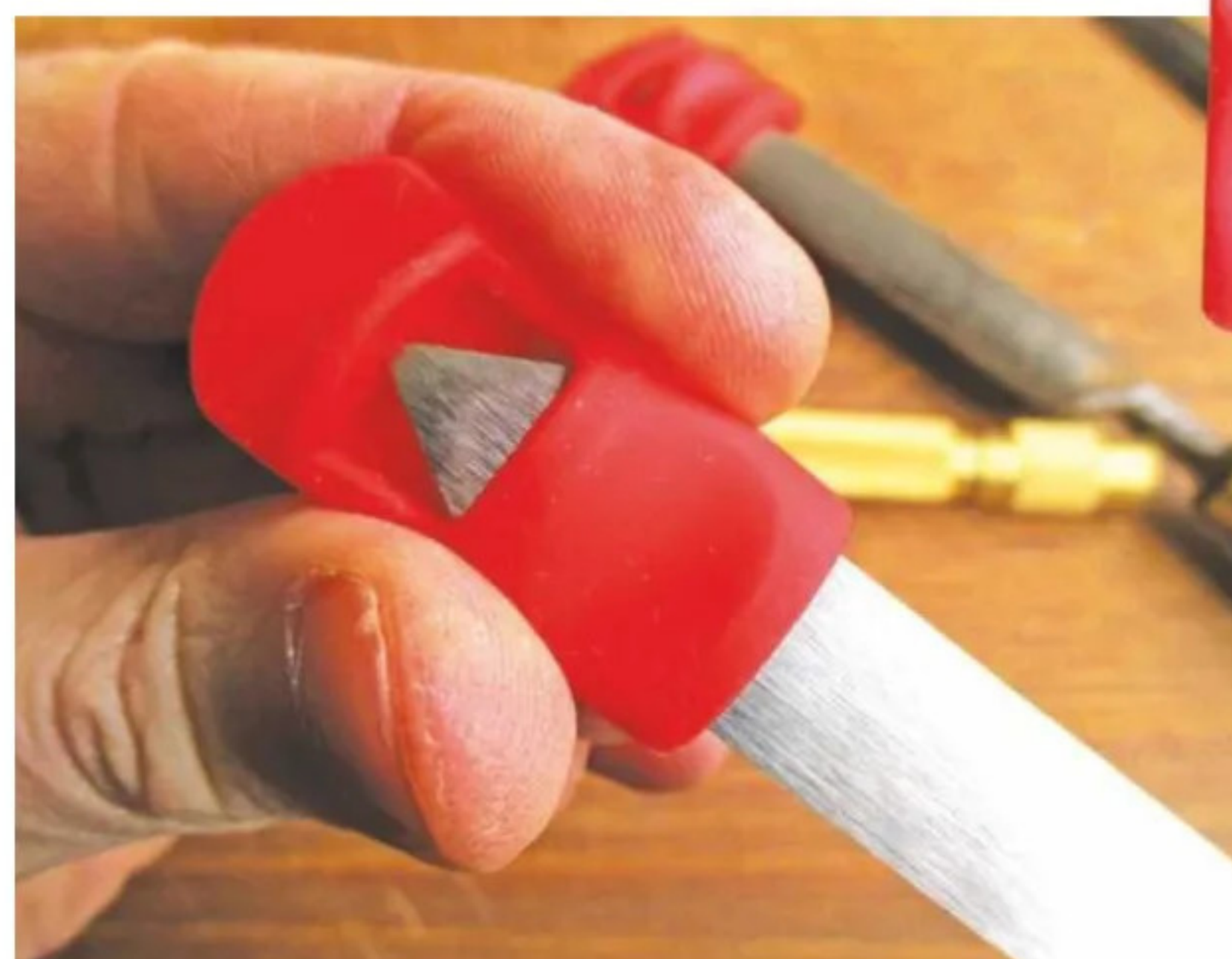
The window allows you to check progress
