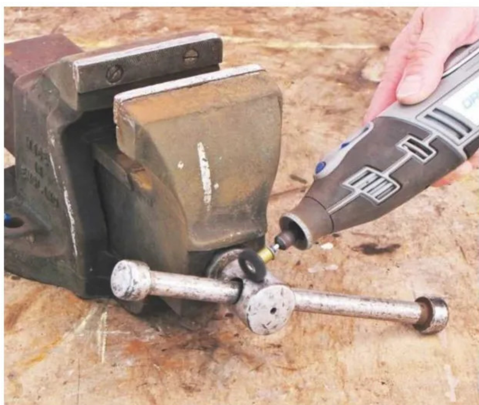
7 The finish on the handle can be revived with a Dremel multi-tool and abrasive brushes, but ensure to wear eye protection throughout
