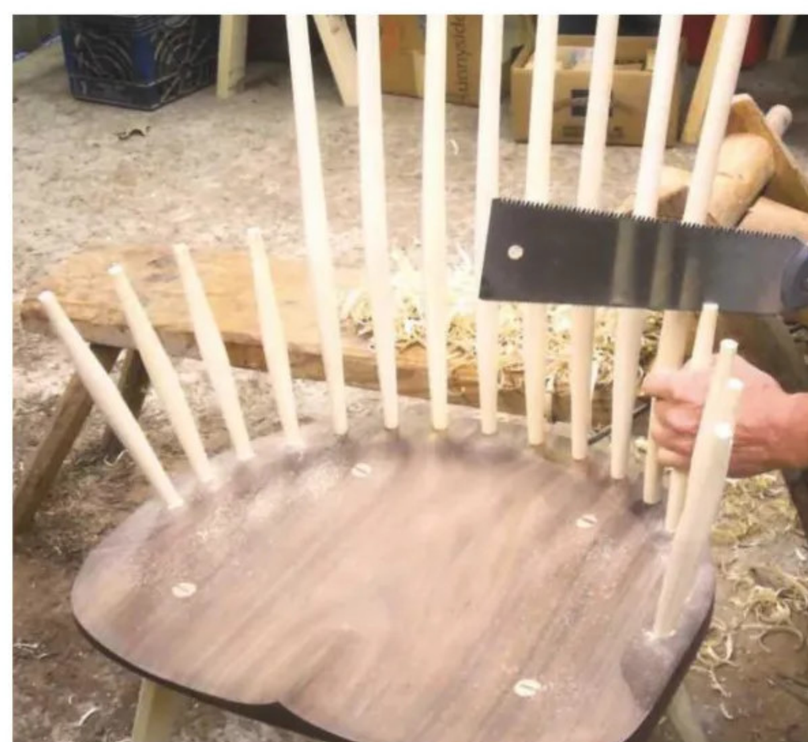
8 Cutting the kerf for wedges
