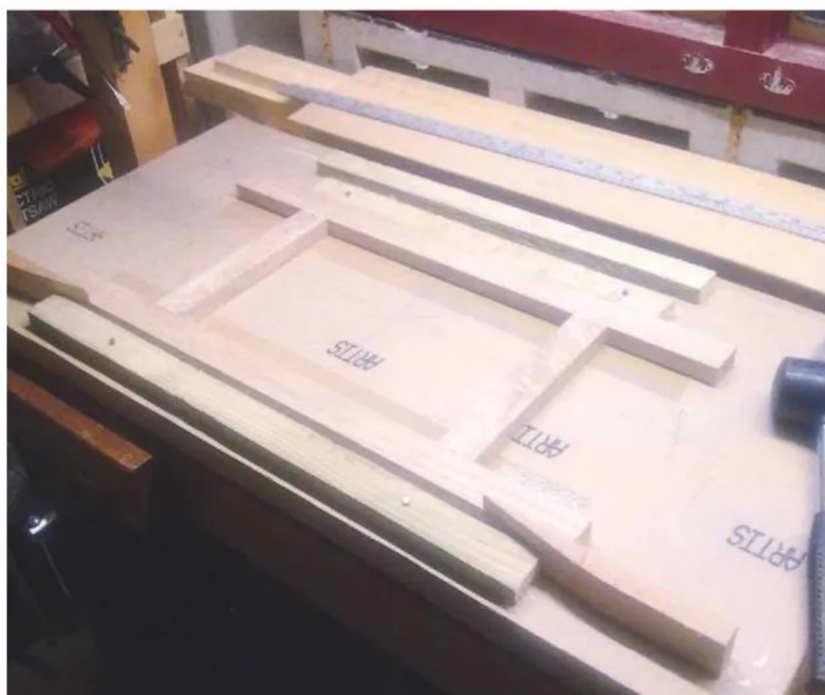
1 This jig was produced to help with making the frame components
