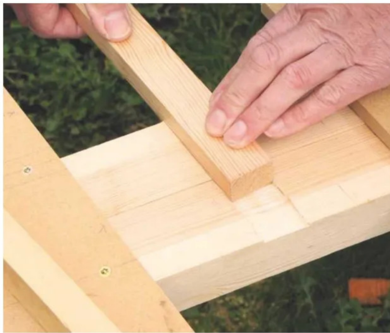
6 Cramp the jig in position and make a test cut. Check the rail fits snugly and adjust the jig if needed
