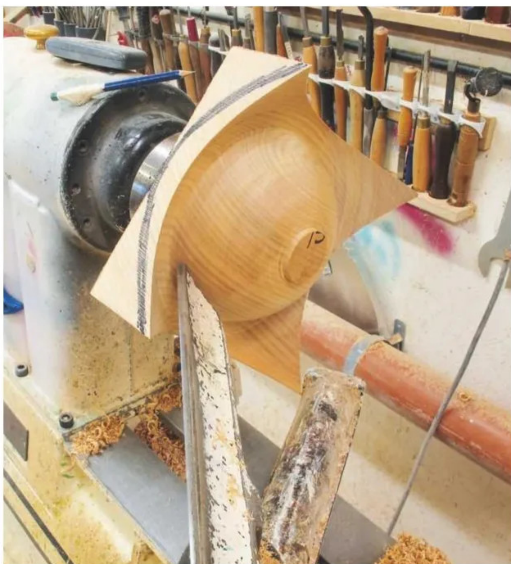
13 I've managed to position the toolrest inside the wings, but the problem now is that I'll have to work right on the blank's end. Ensure everything is tight here as if it moves, you'll break the piece
