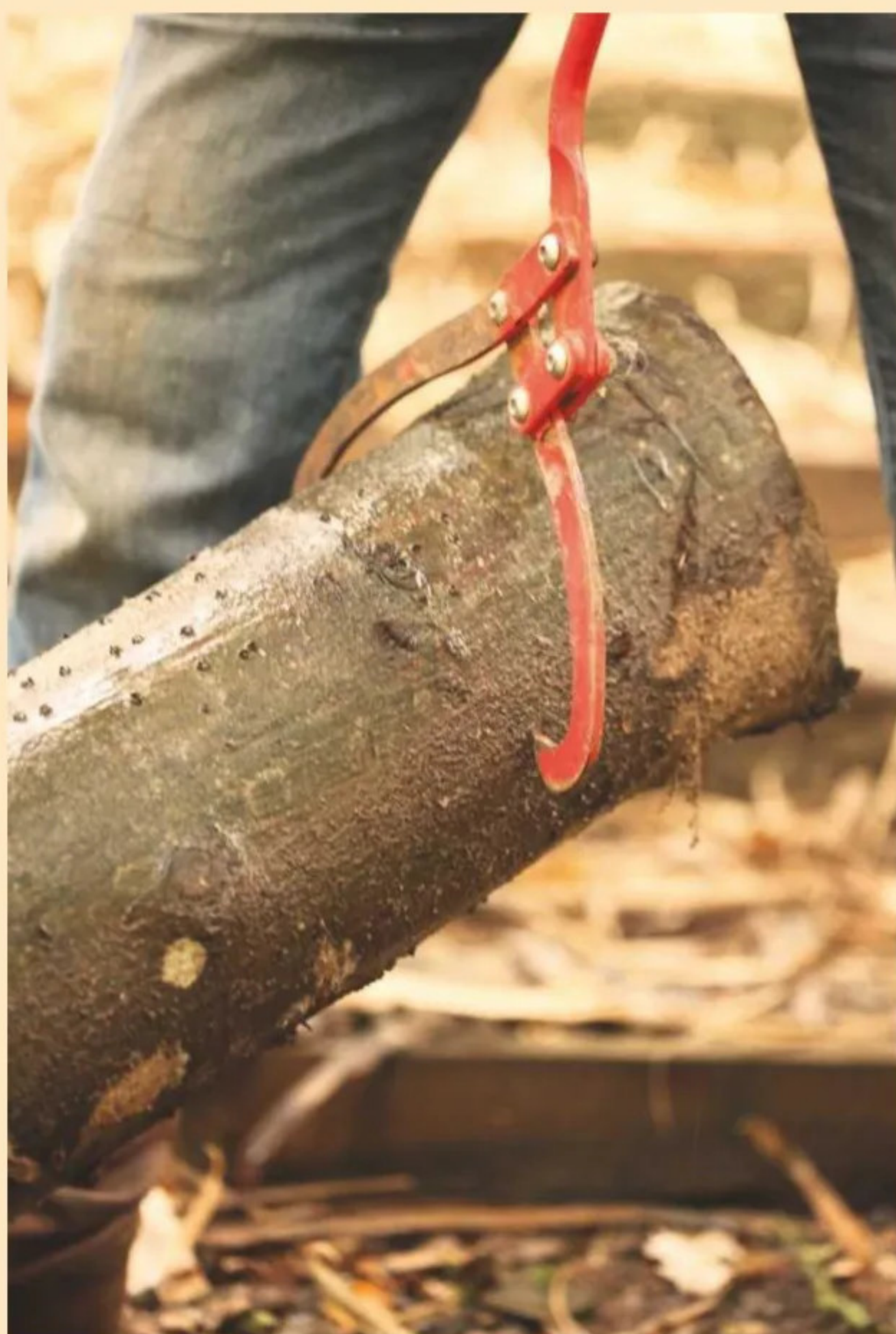
A cunning device for lifting a log – the weight forces it to lock on
