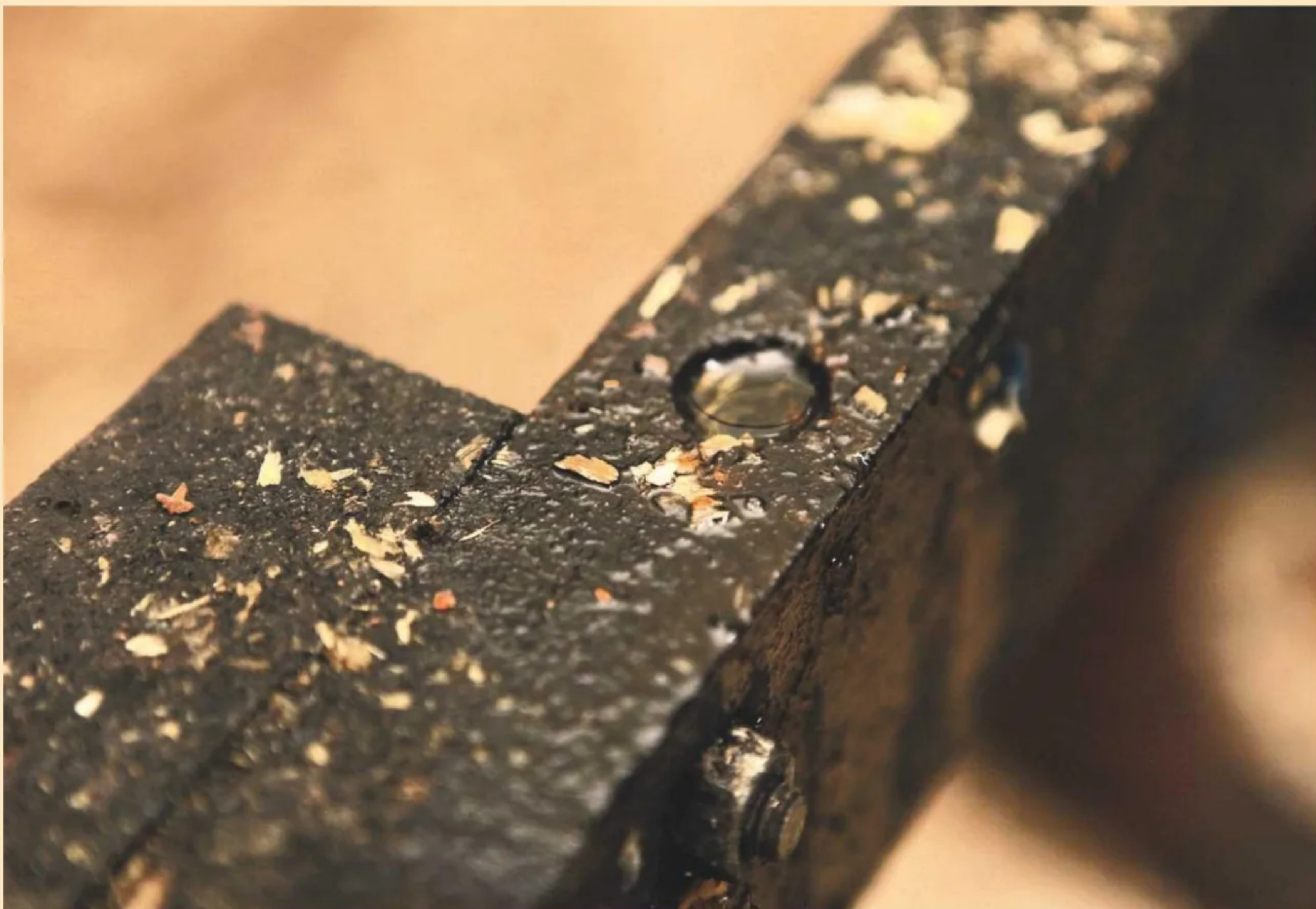
A handy drill hole to hold a reservoir of walnut oil; this lubricates the end-grain, which turn easily in the centre rods
