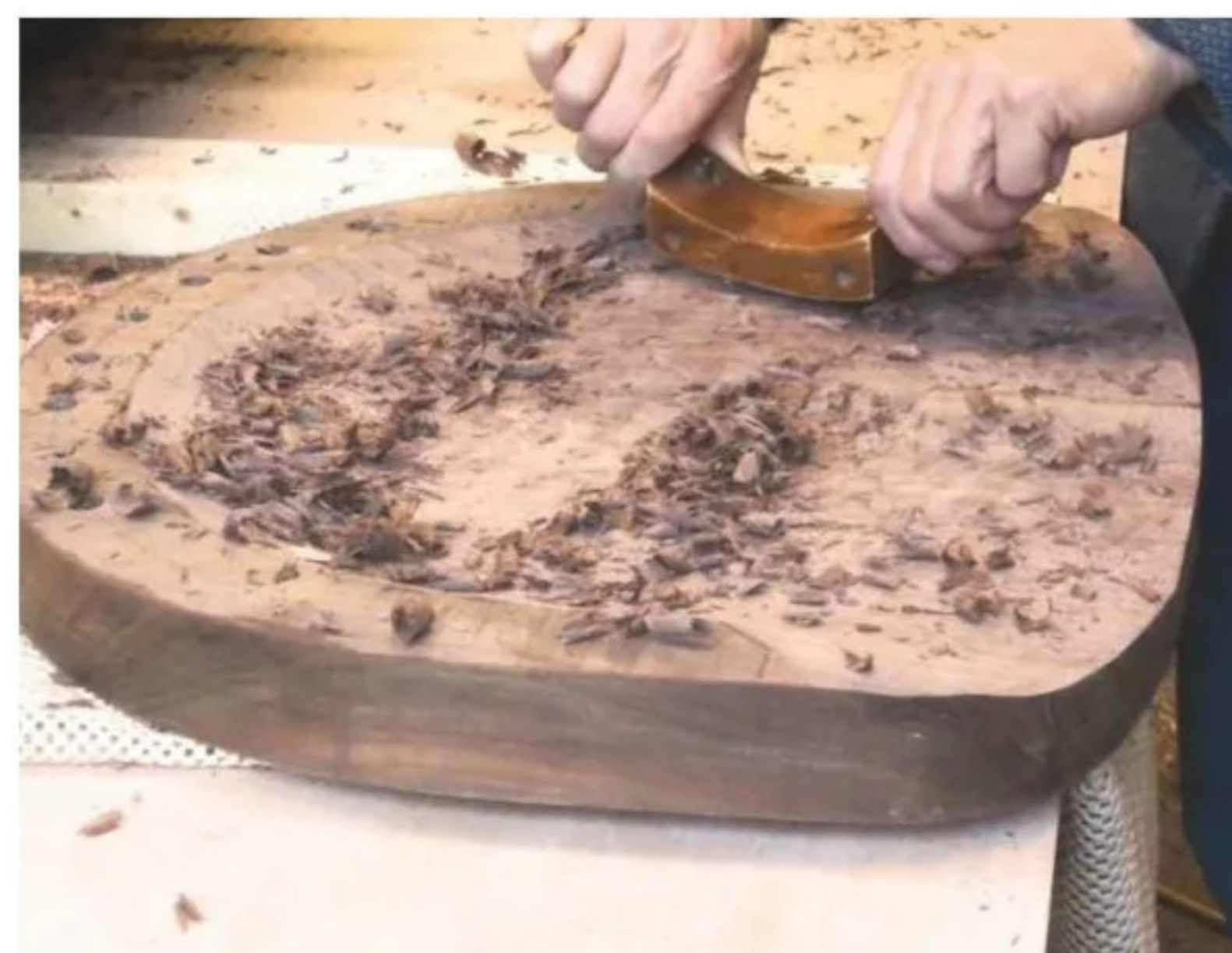
4 Using a travisher to hollow the seat
