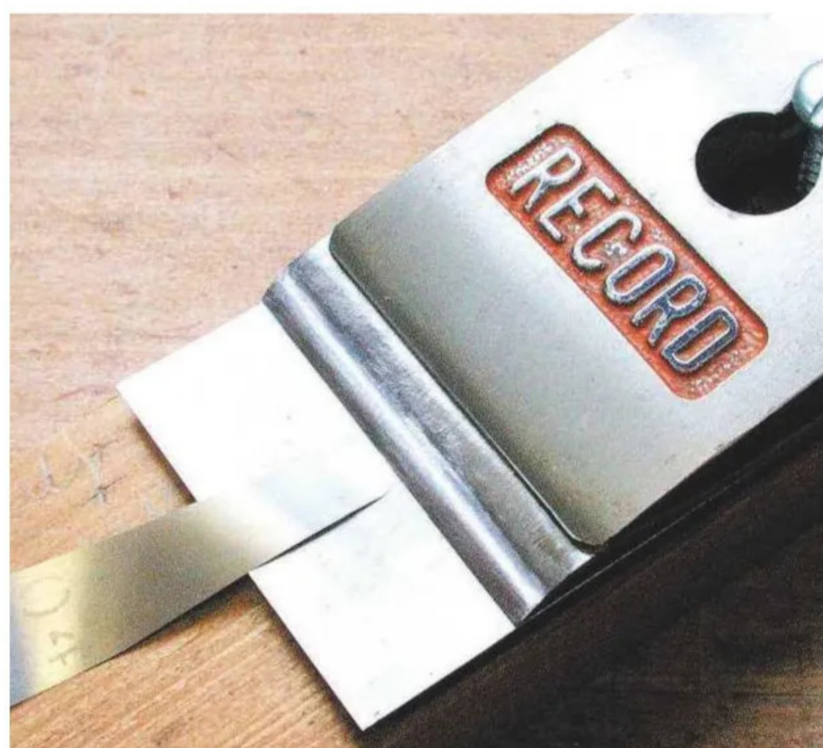
1 I've made a jig that lets me check the cap iron's fit while under pressure
