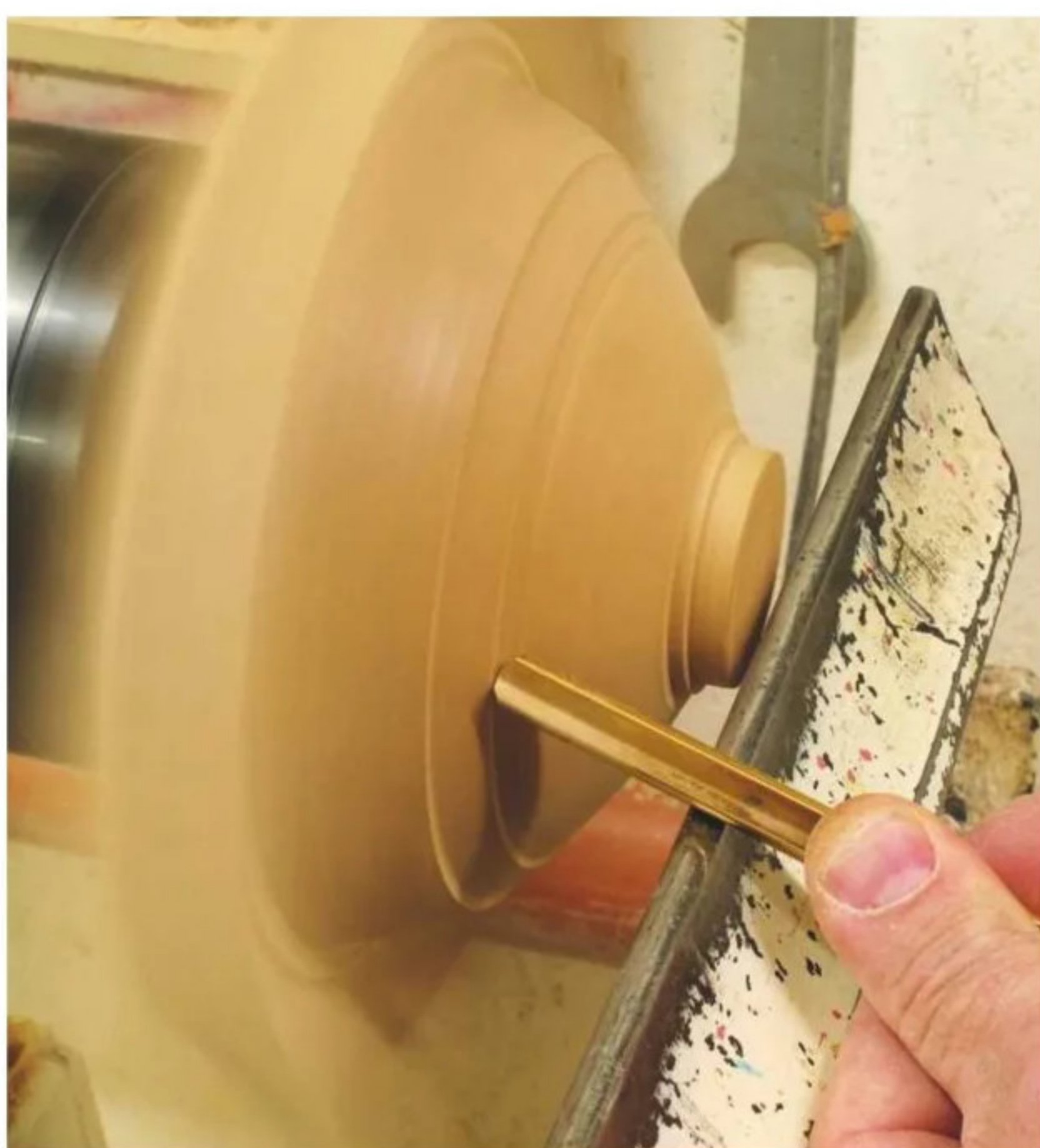
16 It's difficult to achieve a good finish, so I decided to revert to using the 6mm bowl gouge with a light bevel rubbing cut, which will result in a good, sandable finish. Vibration may pose a problem as you near completion
