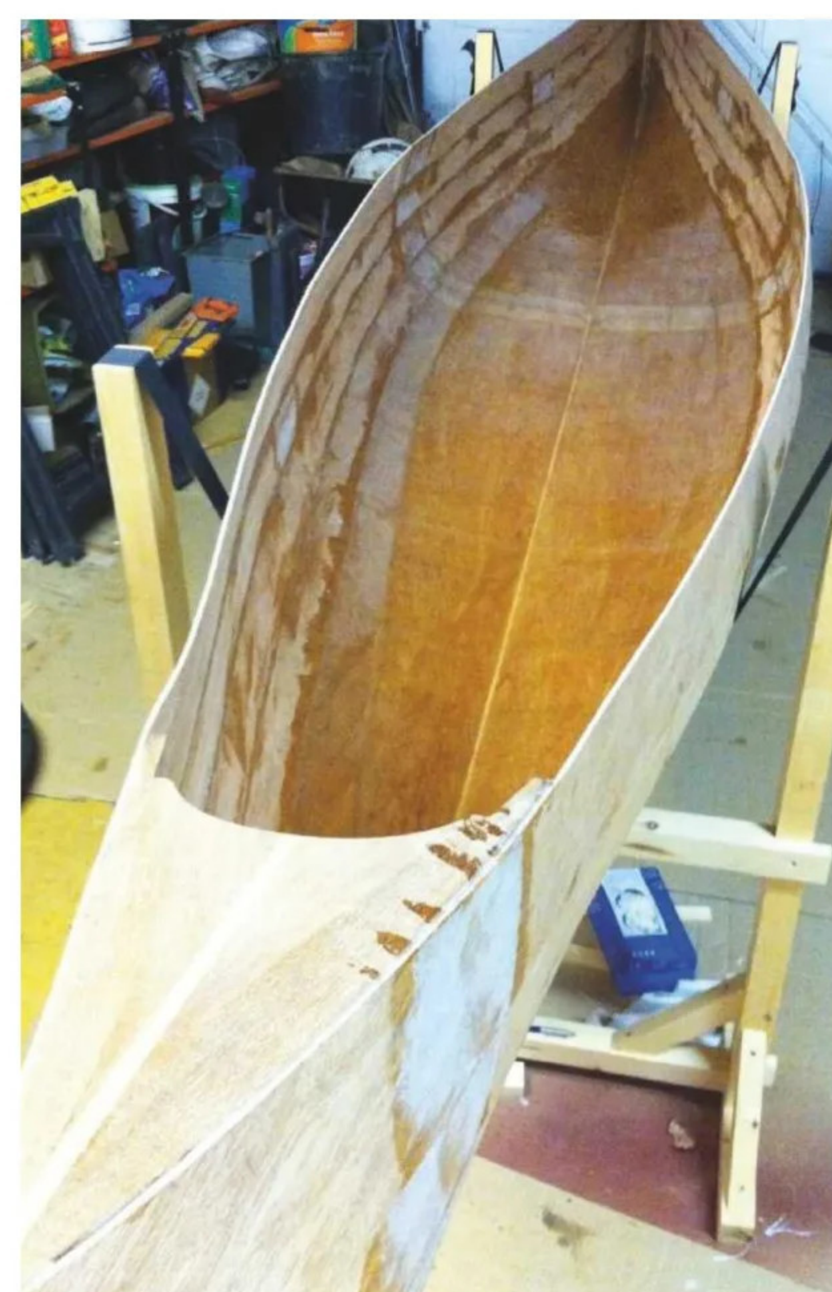
12 ... and the hull interior epoxied
