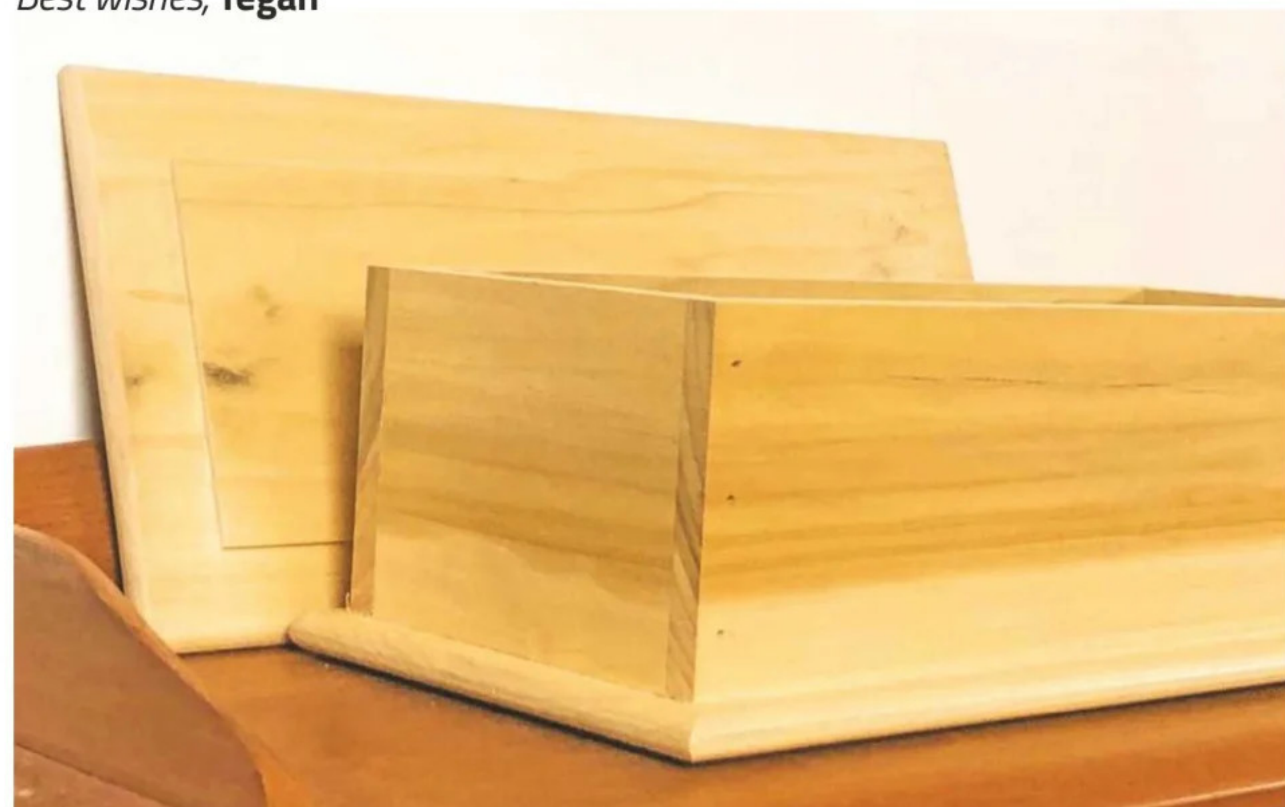
Phil's box was made using butt joints and held together with glue and nails
