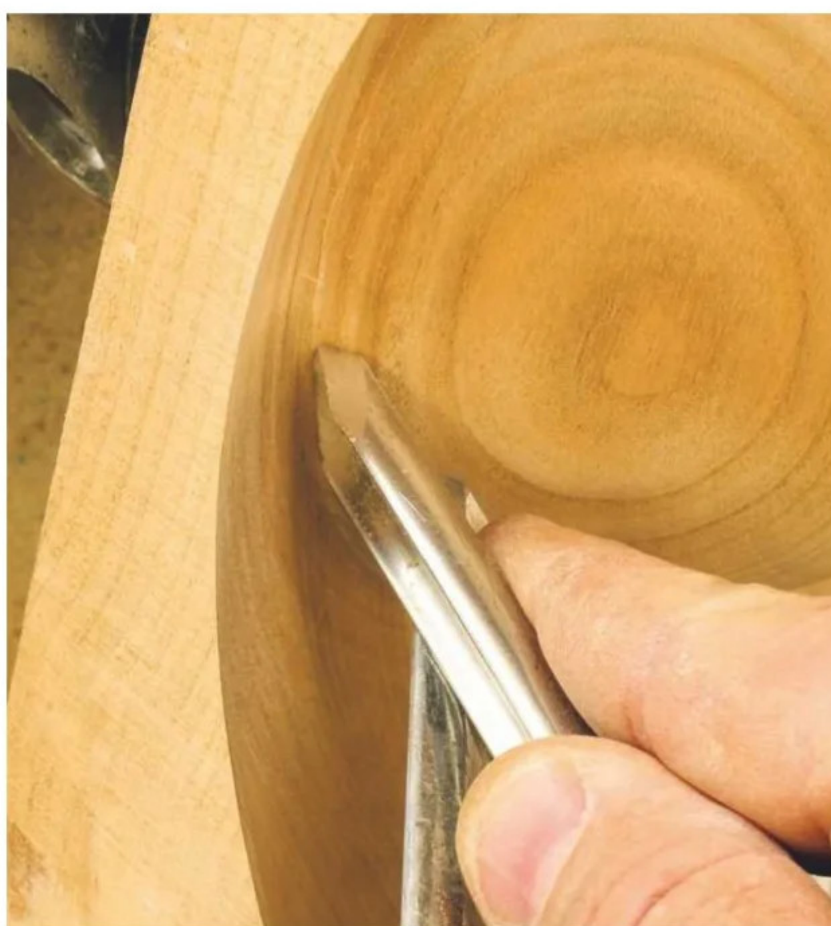
17 I like to have a sharp punctuation point between shape transitions. To get into this tight spot, I changed to my signature gouge, which has a sharper bevel angle of around 40°
