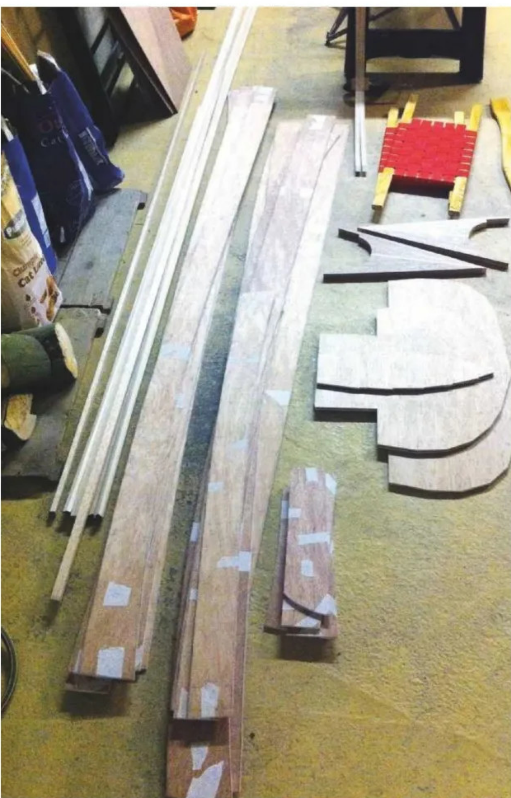
5 The stack of parts amounted to a homemade kit awaiting transport and hull construction
