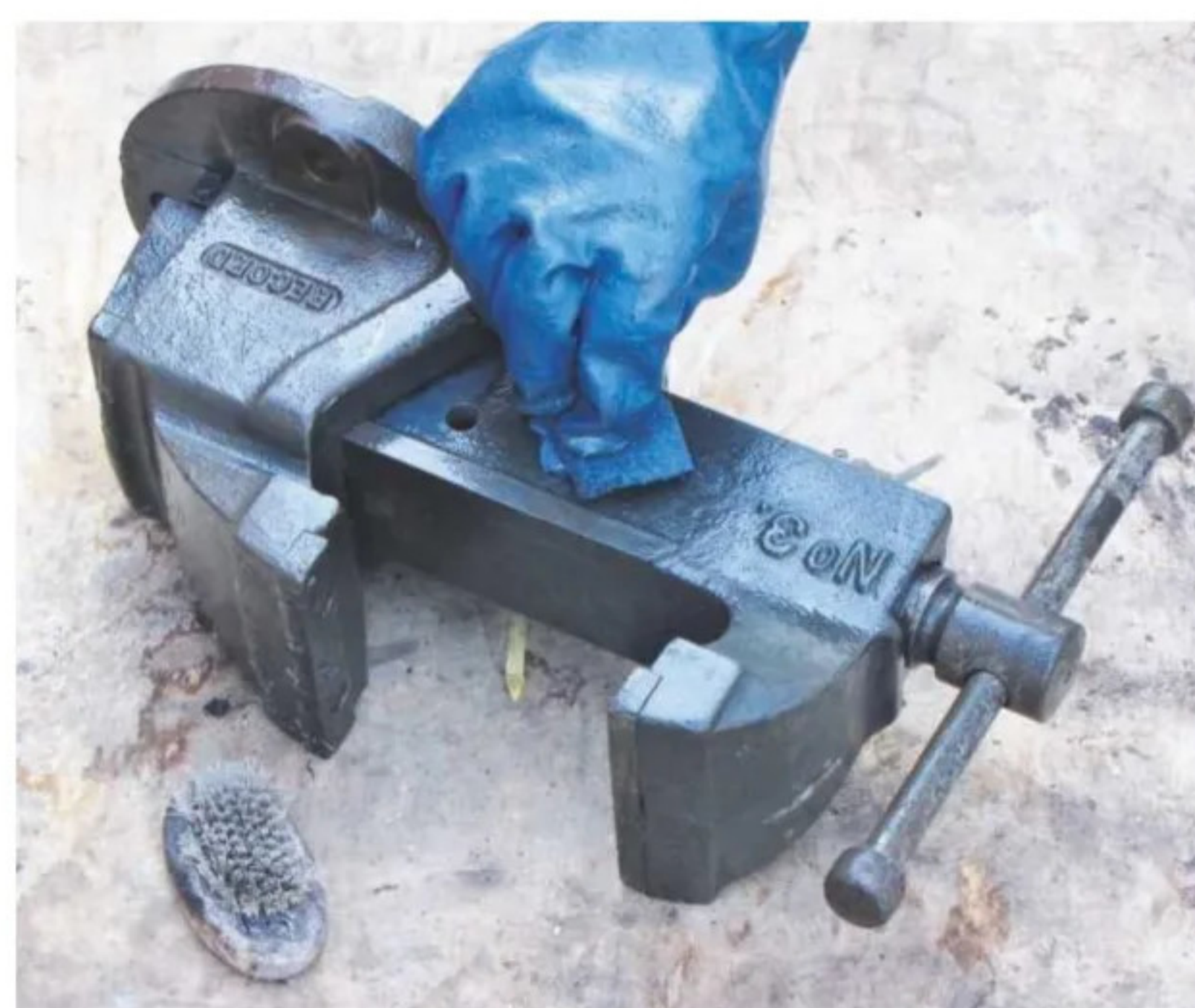
5 Remove black deposit from surfaces with water and an abrasive pad; repeat dip process if necessary
