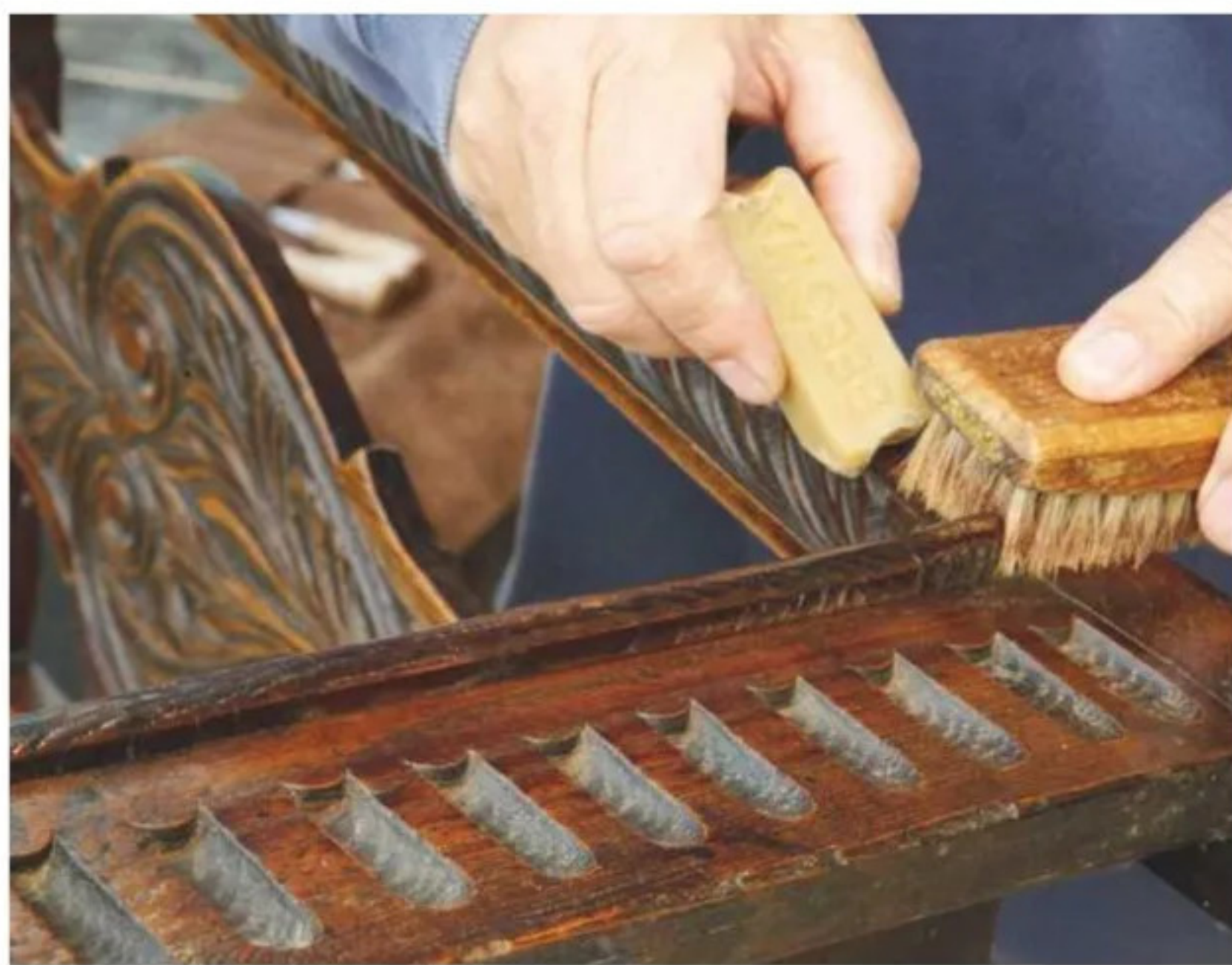
11 Pure beeswax can be rubbed onto coarse-grained and carved surfaces, then worked in with a brush
