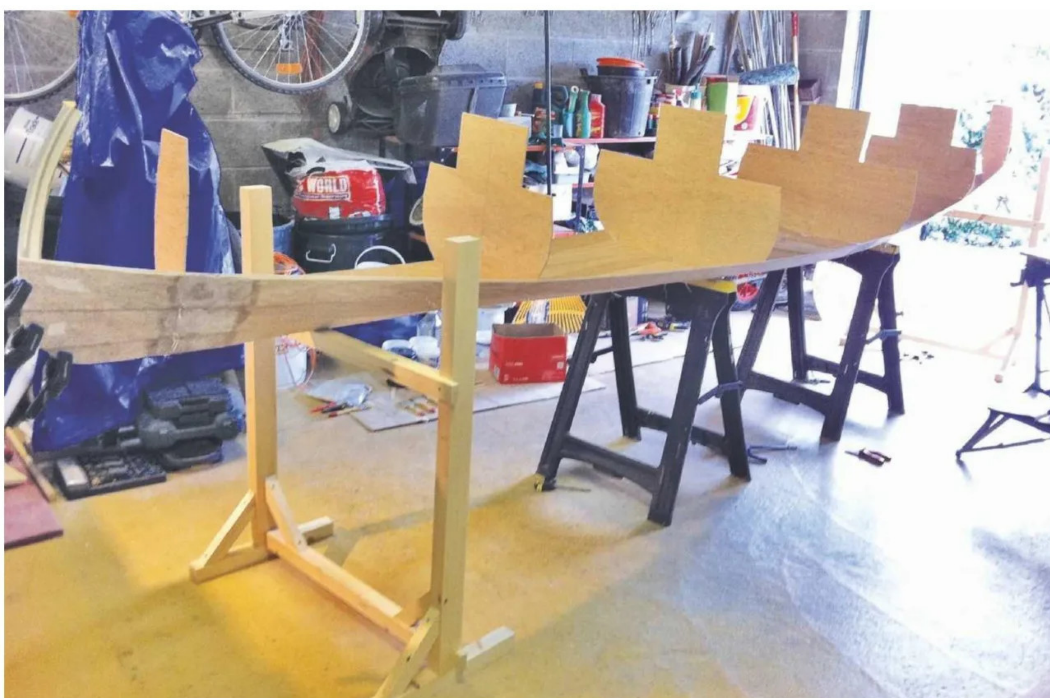
7 At this stage, it's already starting to look like a canoe – note the station moulds used to keep it in shape during construction
