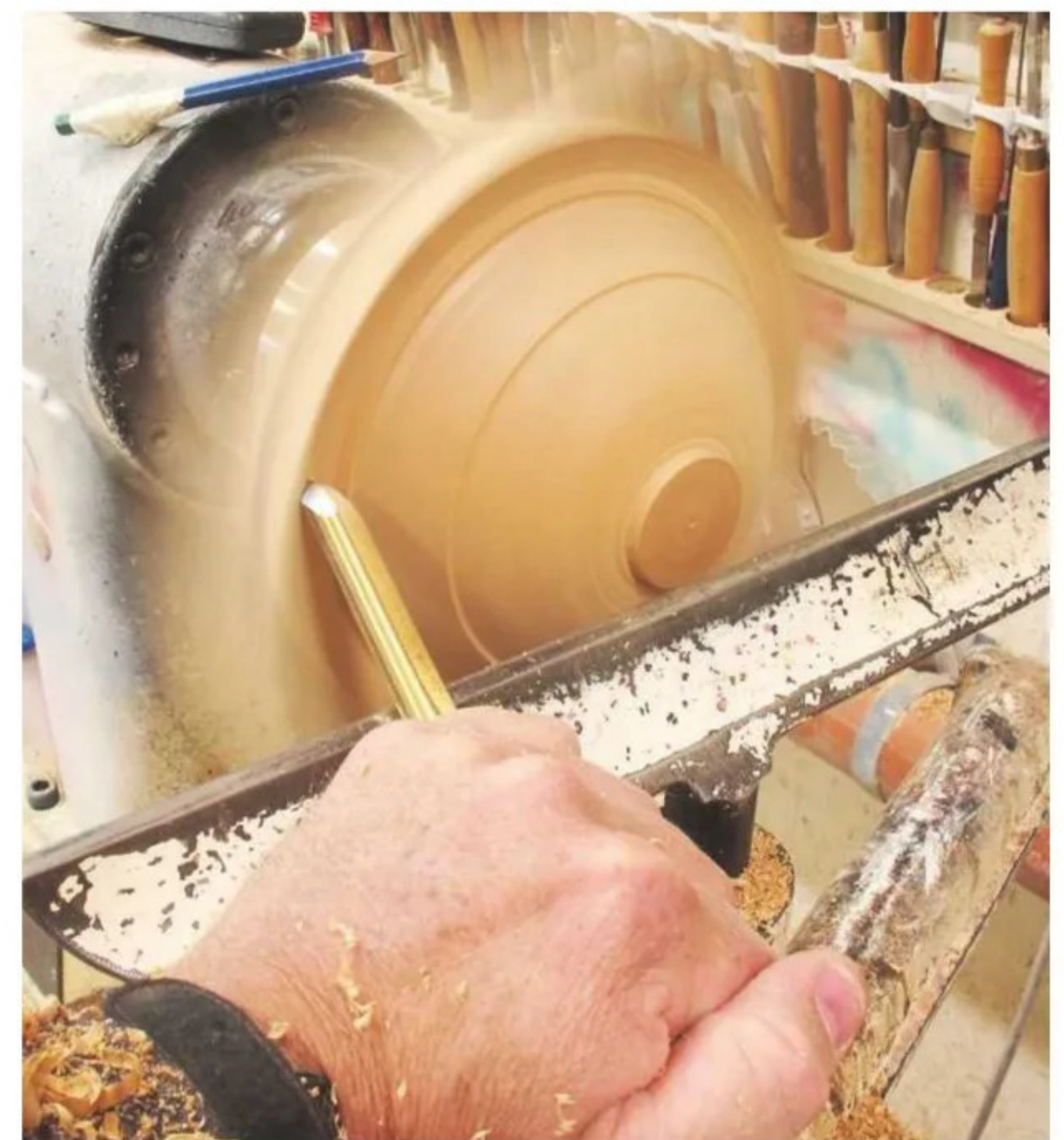
12 I find it's best to work each shape by doing a bit on one side, followed by a little on the other. My right hand has to go towards the floor during this cut, which raises the cutting tip and keeps the tool's bevel in contact with the wood
