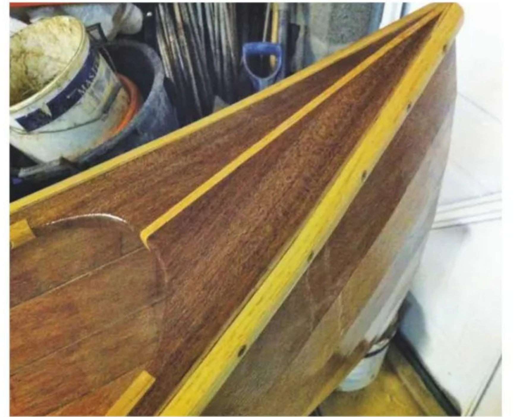
15 The meranti scuppers provide useful tying points for securing bags and the like
