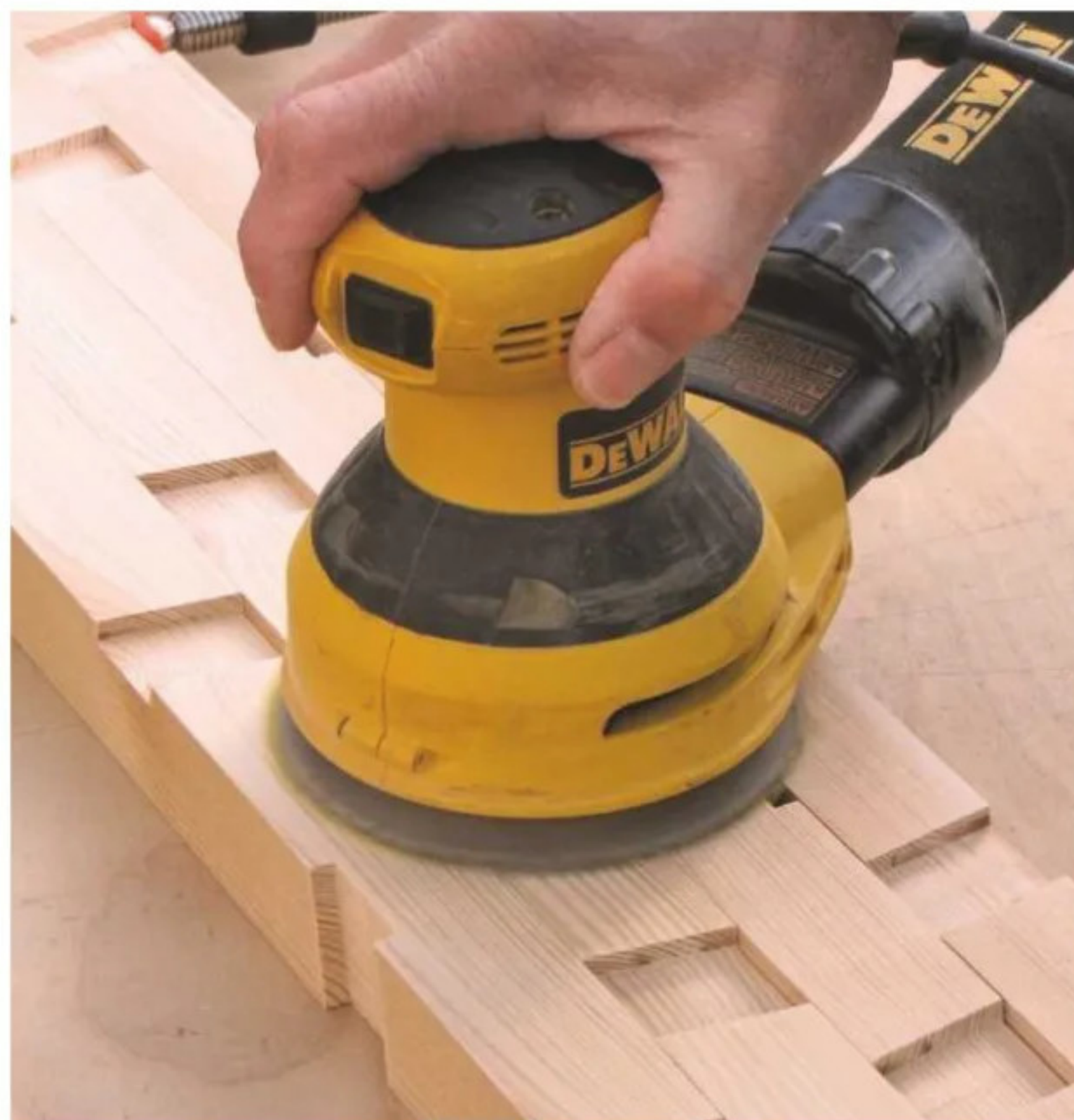
9 Saw legs to length, with compound mitres at the bottom. Sand after routing and remove the arrises
