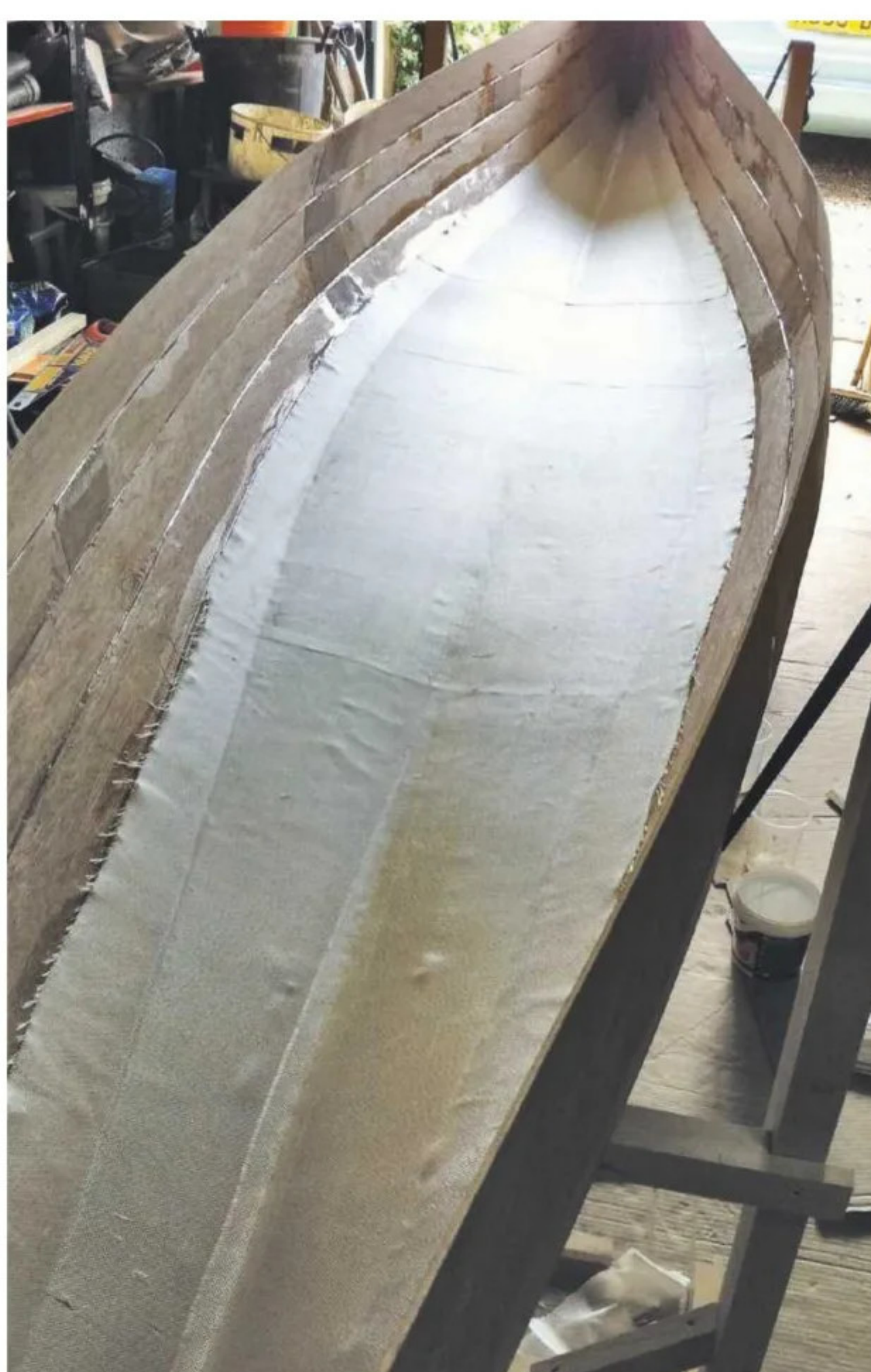
11 The bottom of the canoe was fibreglassed...
