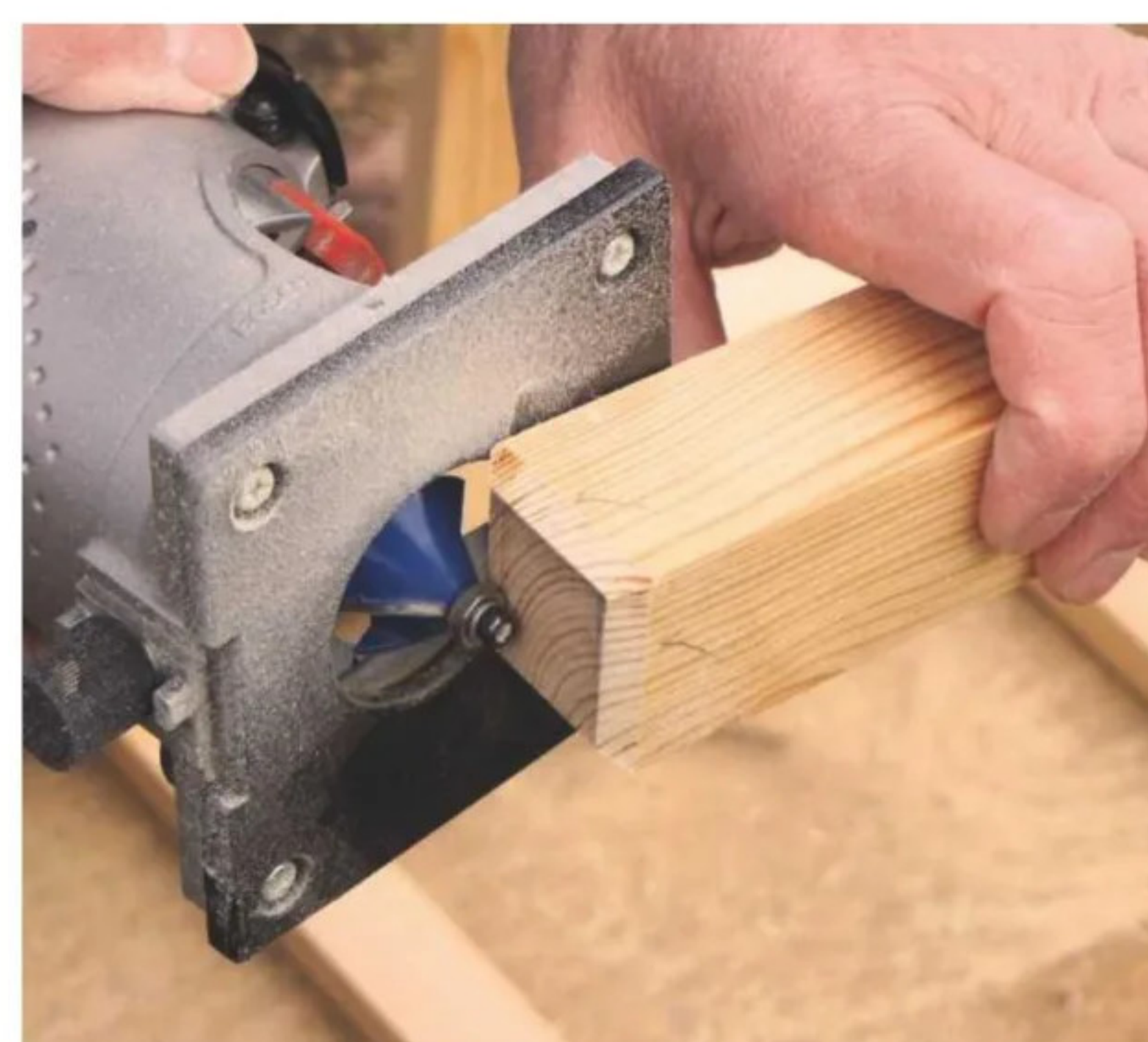
16 Carefully run a chamfer around the end of each leg, using either a small router or block plane
