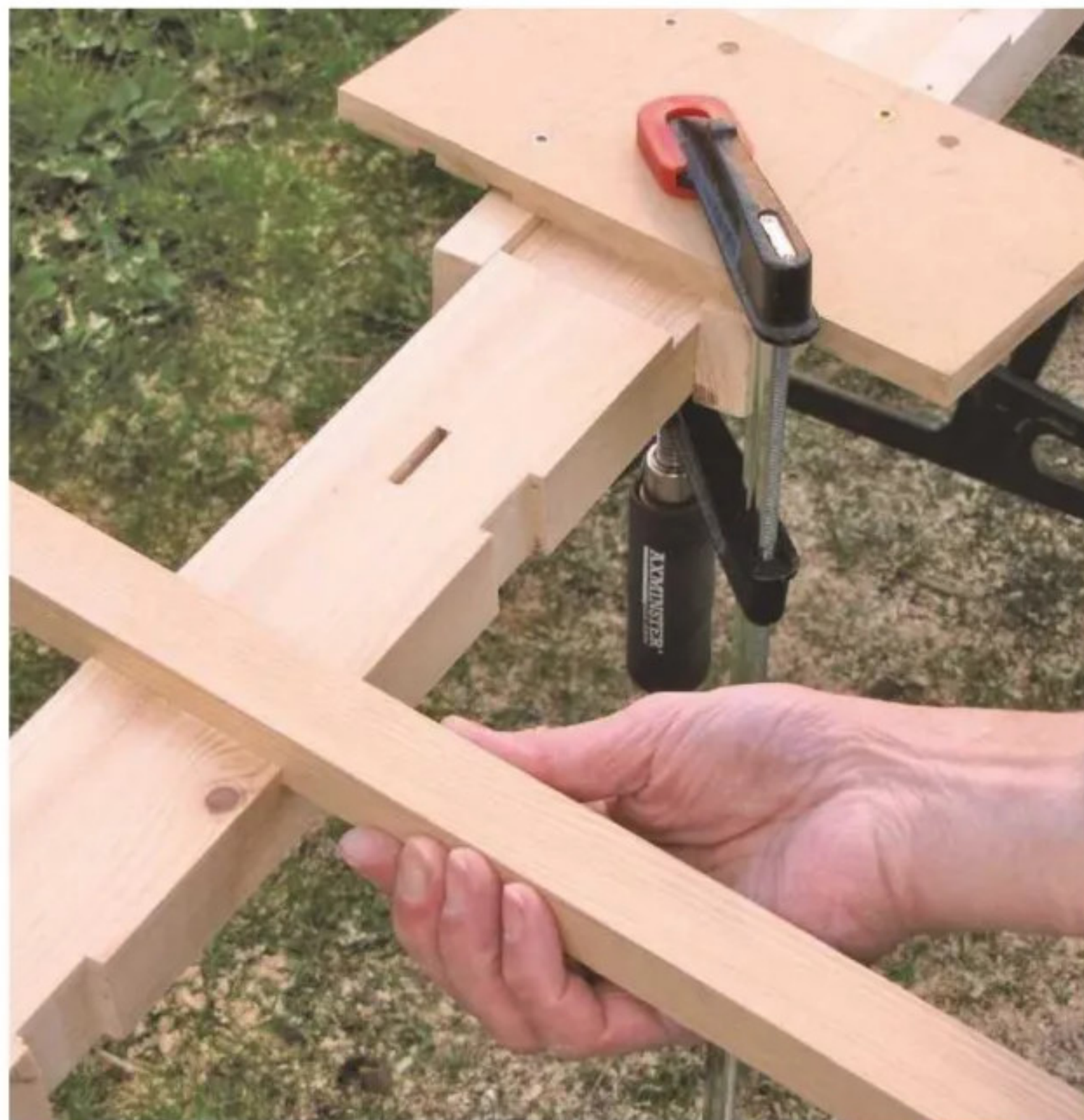
8 Slide a rail across the housings to keep the legs aligned while you move the jig along for the next cut
