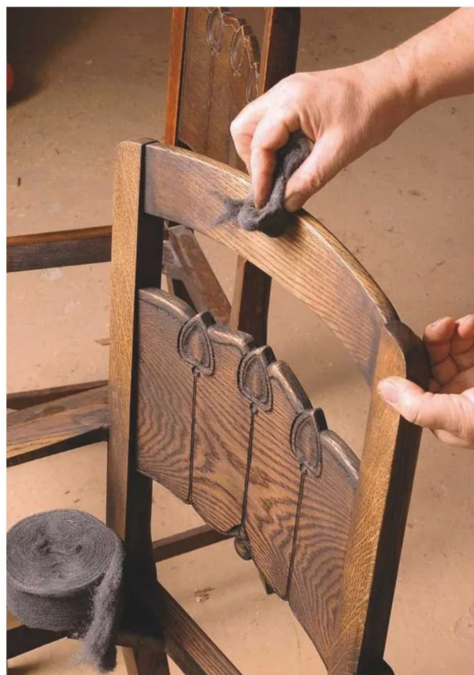
15 Steel wool rubbed in beeswax polish can be used to burnish a surface and shade the colouring with a stained paste
