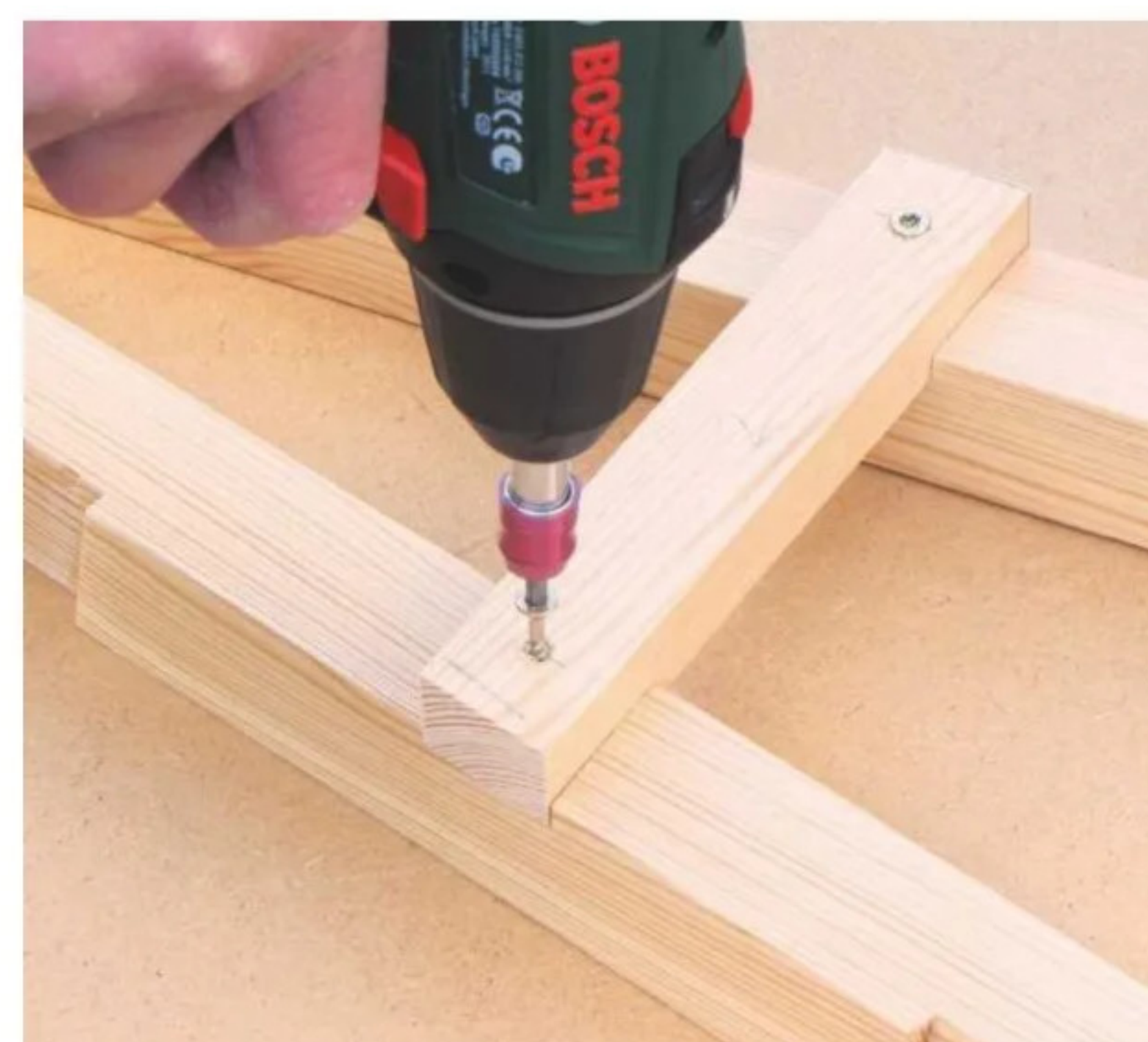
13 Drill pilot holes at both ends of each rail, then screw to the legs. Fix top and bottom rails first
