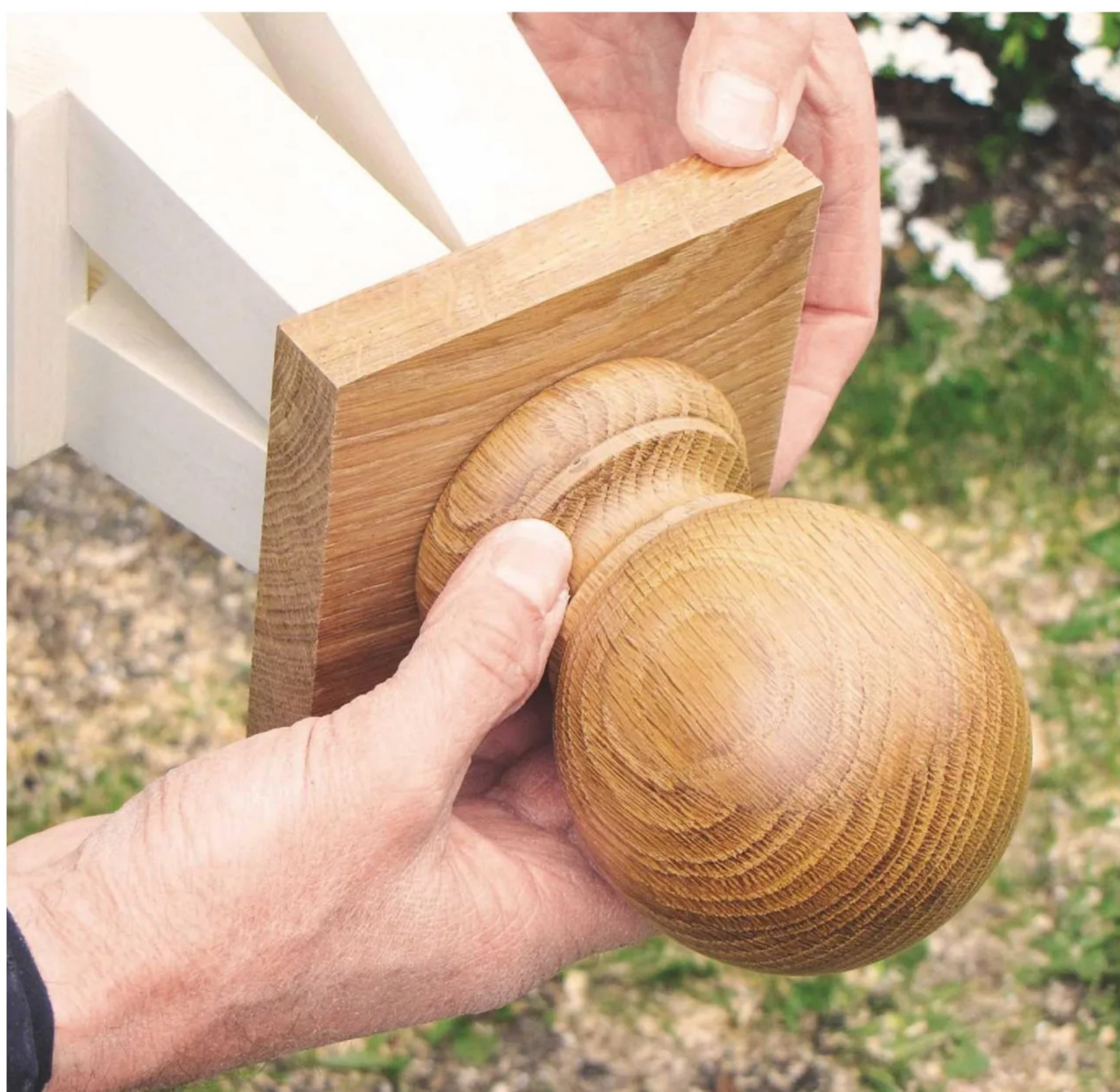
19 To complete the trellis, add a decorative ball or tapered finial, glued into a cap that tops off the legs
