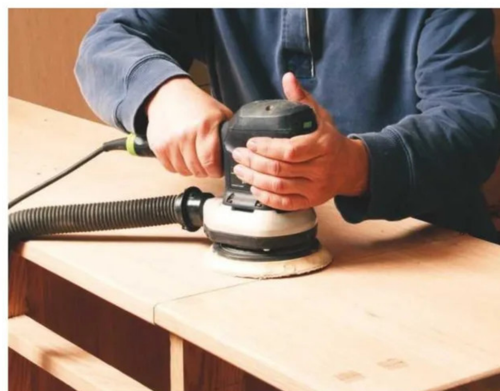
7 The random orbit sander also produces spiral tracks, but each one is different from the last so that no pattern builds up and the effect is smoother
