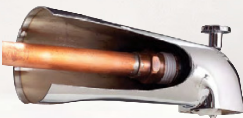
B Screw-on spouts have threads deep inside. They can connect to a copper threaded fitting or to steel pipe.
