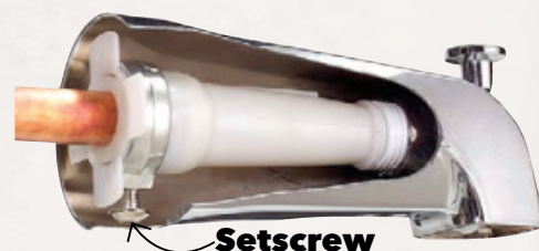
A Slip-on spouts slide over 1/2-in. copper pipe and fasten with a setscrew. This "universal" version also has threads inside, so it can screw onto threaded pipe.
