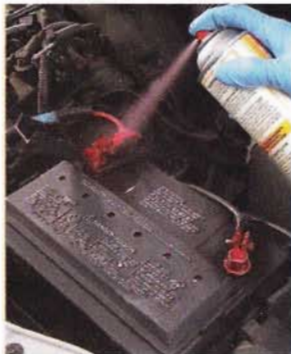
3 Apply a light coat of battery terminal protective spray.
