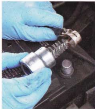
2 Clean the inside of the terminals with the opposite end of the cleaning tool.
