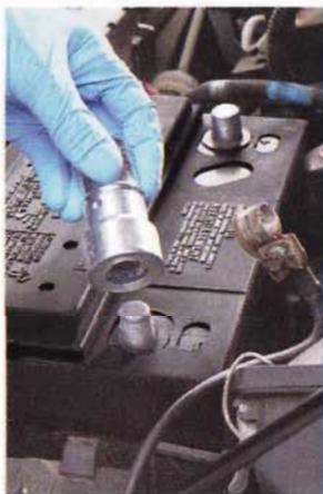
1 Disconnect the battery terminals and use a wire terminal cleaner to clean the posts.
