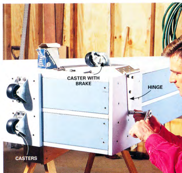
6 Attach the four casters and the strap leaf of the hinges with 1/4-in. x 1-1/2-in. lag screws. Place the caster with a brake on the outer front edge of the rack to hold the rack stationary when sliding items in and out.
