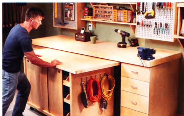
When you're done working, just tuck the rollout bench back under the fixed bench.
