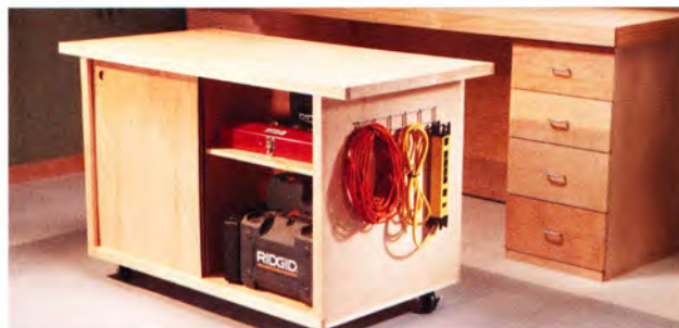
The rollout opens from both sides—one side for large tools, the other for small fasteners and supplies. Hooks at each end hold cords and hanging tools.
