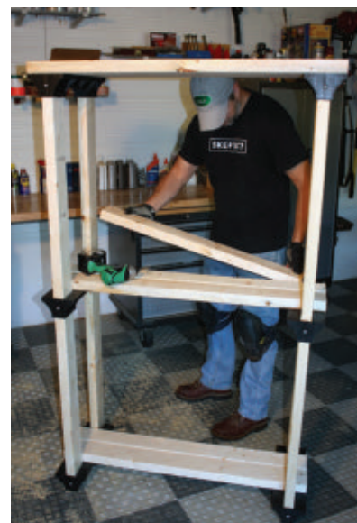
The shelves simply slide over the 2x4 legs. Fasten the shelf brackets in place and then complete the lower and middle shelves by cutting 2x4's to fit between the legs.
