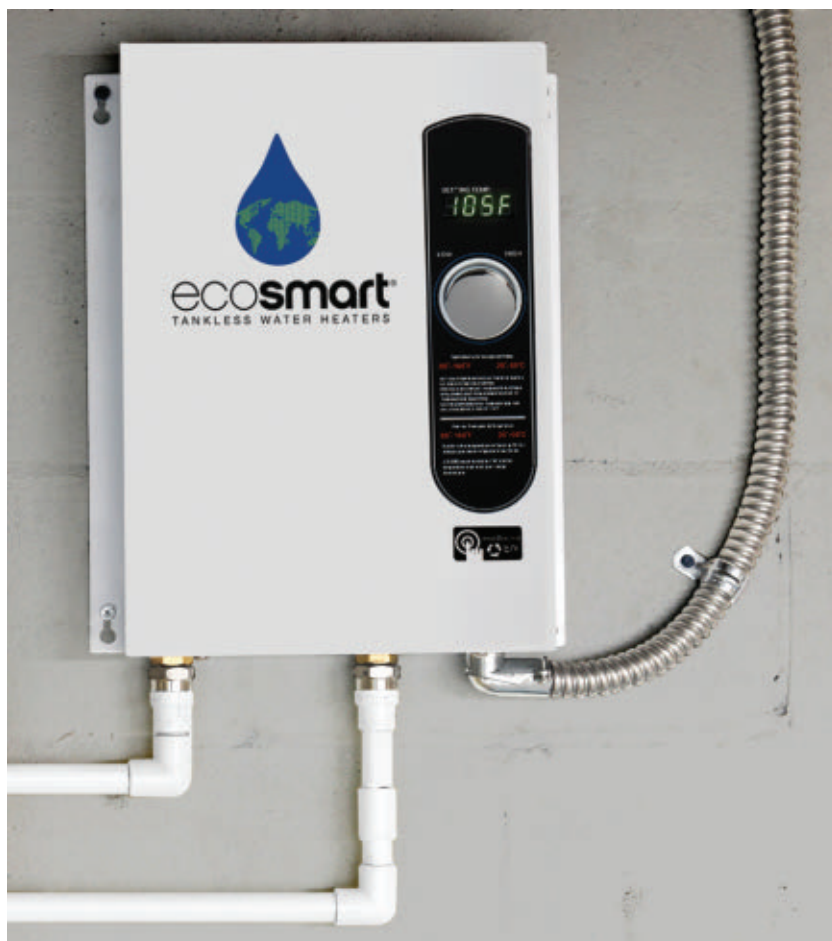
The EcoSmart Eco-18 model requires two 40-amp breakers for installation and has a 75-amp draw.
