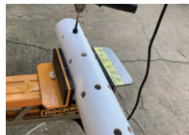
I drilled three 3/4" holes every six inches into the bottom of the pipe.
