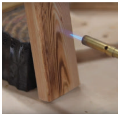
A Bernzomatic hand torch works well for charring wood.
