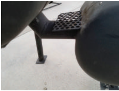
Weld L-shaped metal tubing to connect the smoke chamber and fire box.
