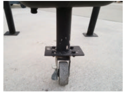
A wheel installed on the leg support will help with mobility.
