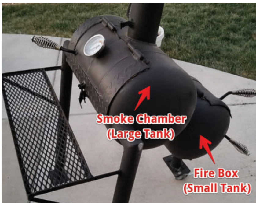
Two 30-lb. propane tanks are cut and welded together as the smoke chamber. A single tank is used for the fire box.
