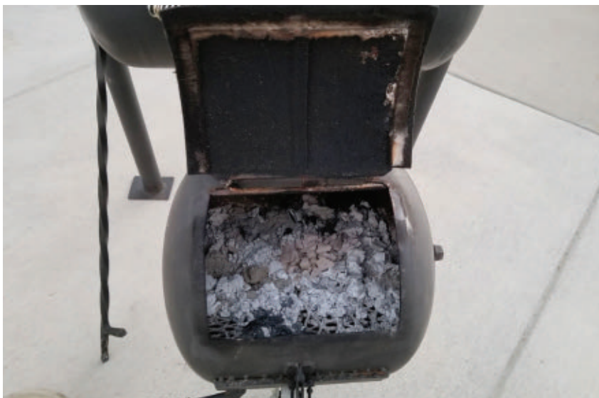
Construct a hinged fire-box lid from diamond plate.
