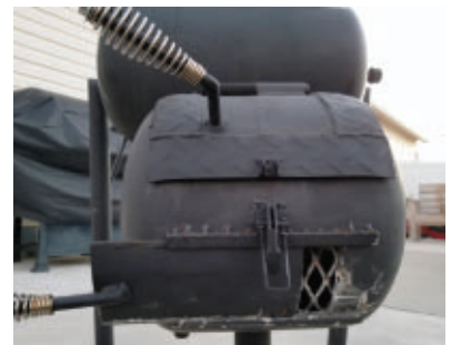
Near the bottom of the fire box, add an air-intake that can slide back and forth to regulate airflow and heat. Use covers on the bar-stock handles to protect your hands from the hot metal.
