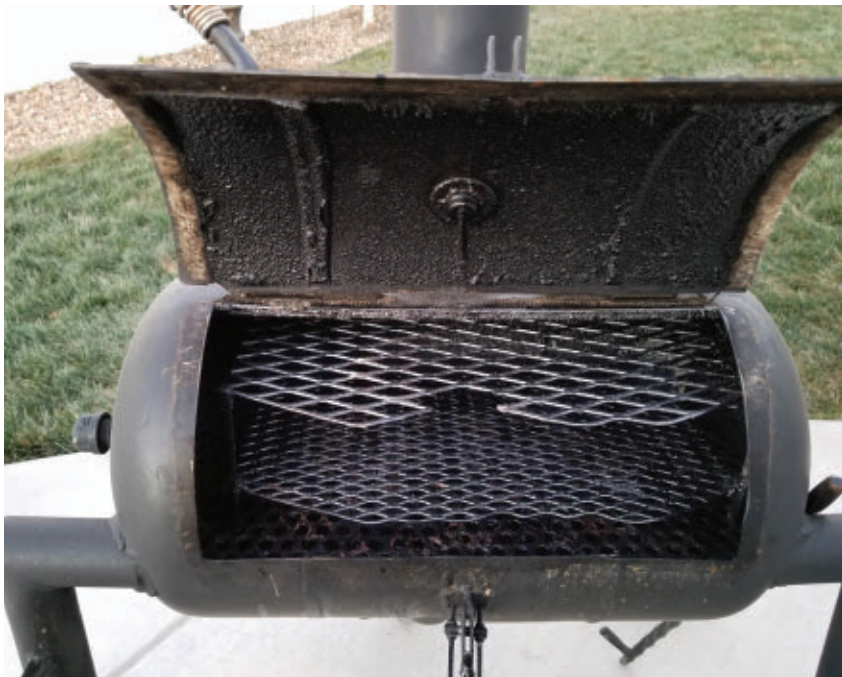
Expanded metal is used for the grill surface.
