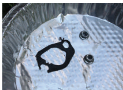
The carburetor will be sealed to the other parts of the mower with gaskets, so look for damage to the gaskets as you remove it.
