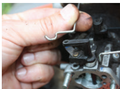
Remove the throttle cable and any other connections from the carburetor.
