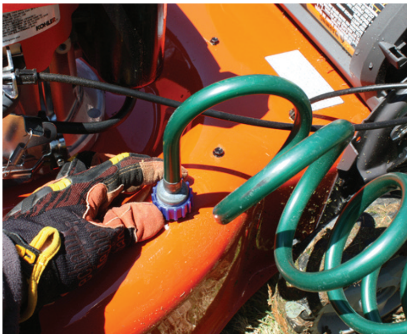
Clean and lubricate your equipment on a routine basis to keep it running in top condition. The Husqvarna mower shown has a garden hose inlet that makes it easy to wash out the deck.
