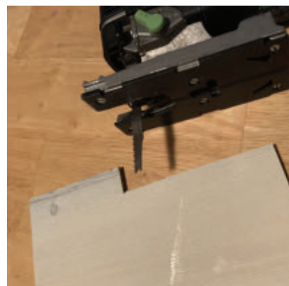
The thin blade of a jigsaw is easy to maneuver when making notches or intricate cuts.
