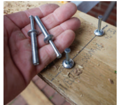
The sleeves of the masonry anchors expand when the fasteners are driven inside them.
