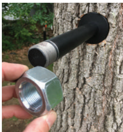
A tab nut is used to keep brackets on the perch.
