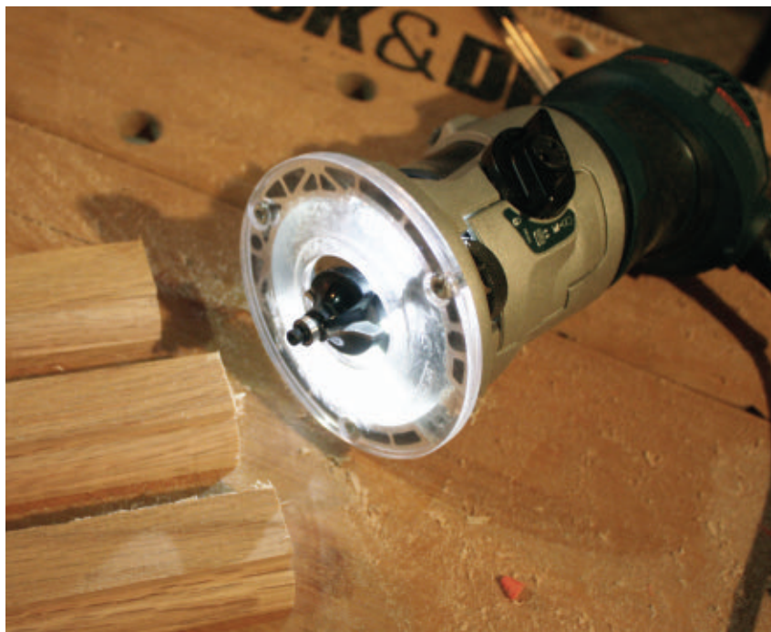
An LED work light is another helpful feature to aid cutting visibility.
