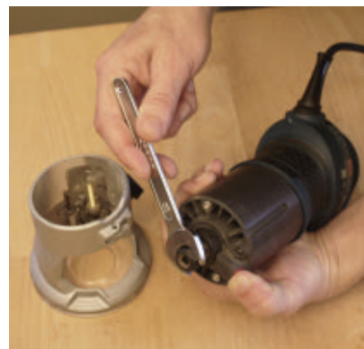
An easy-to-remove router base is a welcome feature when it's time to change the bit.
