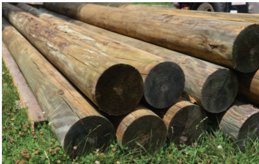
The posts of this fence are made of 6" pressure-treated round poles.
