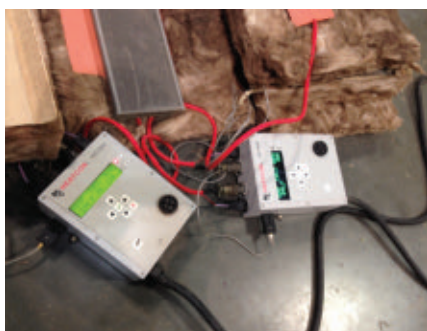
Heatcon units control the temperature.
