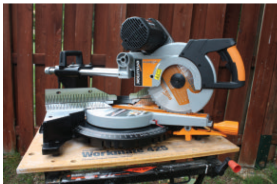
Evolution's RAGE3 10" TCT Multipurpose Sliding Miter Saw cuts steel, aluminum and wood using the same blade.
