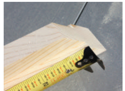
When measuring for the plywood, take the measurement from the corner of the rabbet, not the outside corner of the stock.
