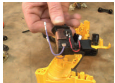
The wires of the switch can be tested with a multimeter. Test the current on both switches.
