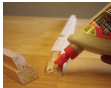
Apply glue to the corners and clean up any excess that squeezes from the joint.
