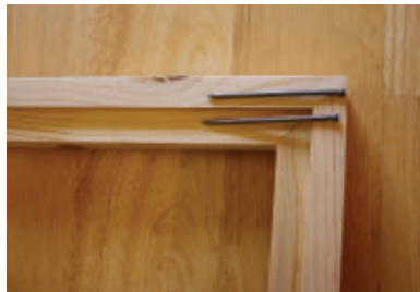
I fastened the corners with a combination of 3" finish nails and wood glue.
