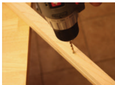
Predrill the cleat for the mounting screws.
