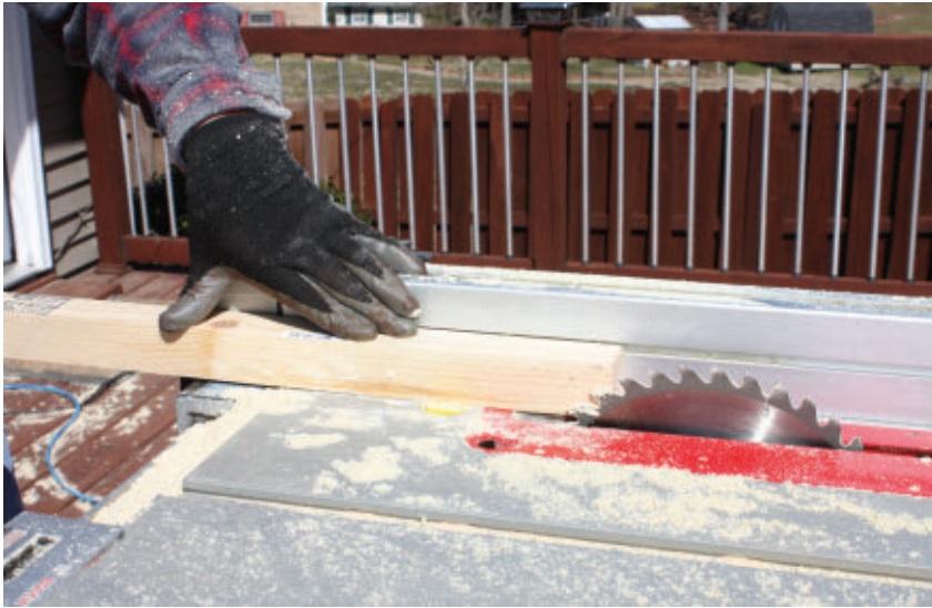
Rip 2x4's into 2x2's and square the edges of the 2x stock.
