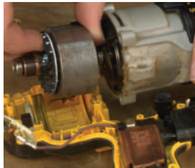
Pull the motor and transmission assembly from the drill.
