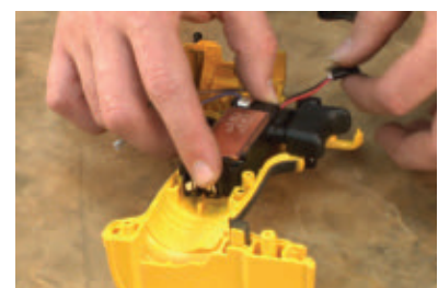
Set the new switch.
