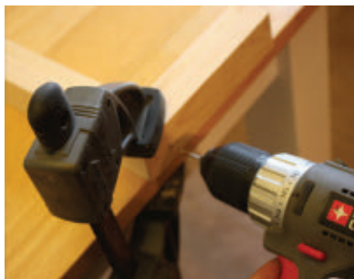
Predrill holes for the fasteners.
