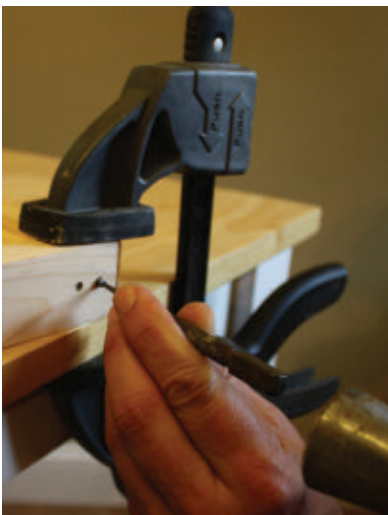
Set the nail heads below the wood surface to leave room for wood filler.
