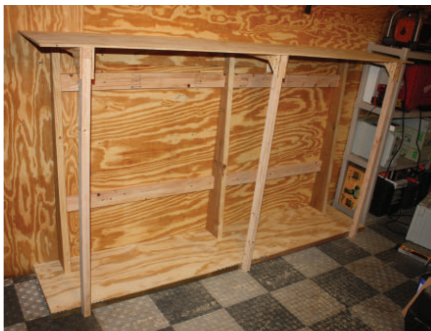
The top shelf is made from 1/2" plywood to provide additional storage space.
