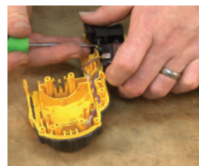
Route wires into the housing.
