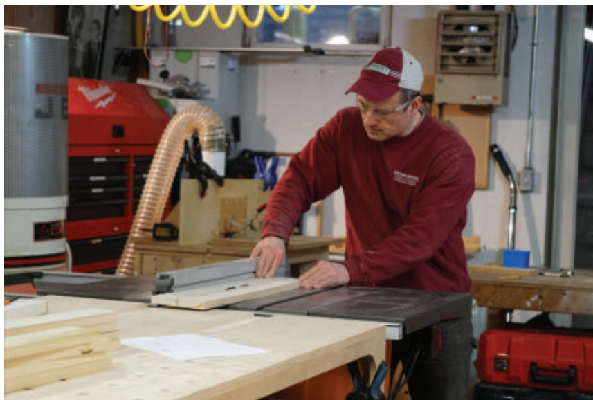
Rip legs and stiles to width on a table saw.
