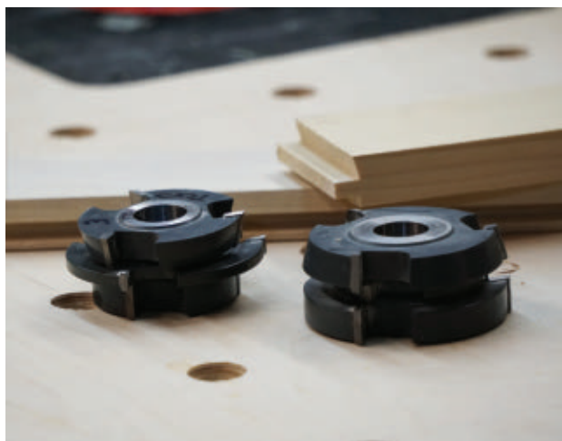
A typical reversible bit set includes one cutter that cuts both the sticking and the cope, and one slot cutter for cutting a panel groove.
