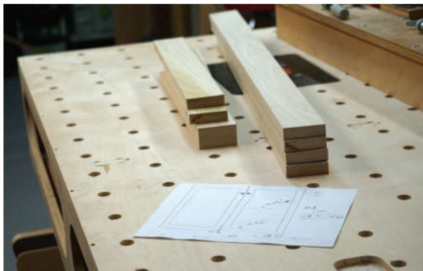
For these shaker-style cabinet doors, the legs and stiles measured 2-3/4" wide.
