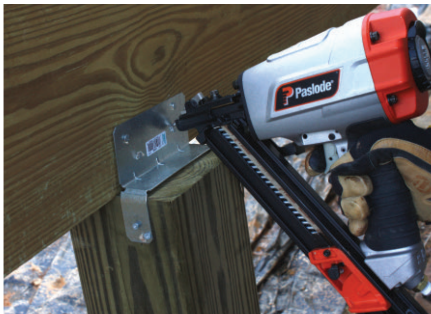
Paslode's Positive Placement Nailer has a special guide tip designed to shoot the nails right into the tiny holes of metal construction hardware without the imprecise impact of a hammer — a real timesaver.
