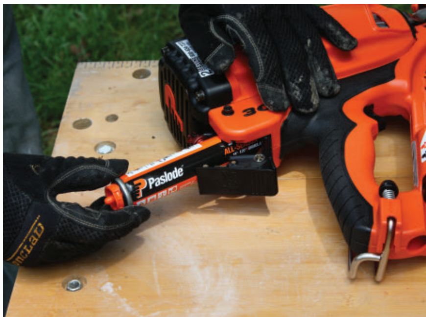
Cordless framing nailers are powered by a combination of lithium-ion batteries and gas fuel rods.
