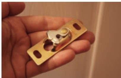
Metal lock tabs are mounted to the top of the door will connect to the hangers.
