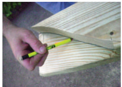
We then used the template to mark the decorative profile on the board ends.
