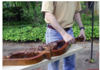
We used an old piece of furniture to create a template for the decorative detail on the ends of the boards.
