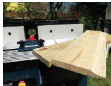
This photo shows the resulting cove cut at the top of the treated wood siding.
