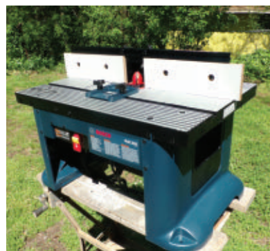
For a stable work surface and smooth, consistent cutting, we milled the siding using a router mounted in a router table.
