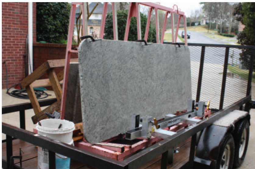
The granite slabs are transported on special racks that reduce vibration on the road.
