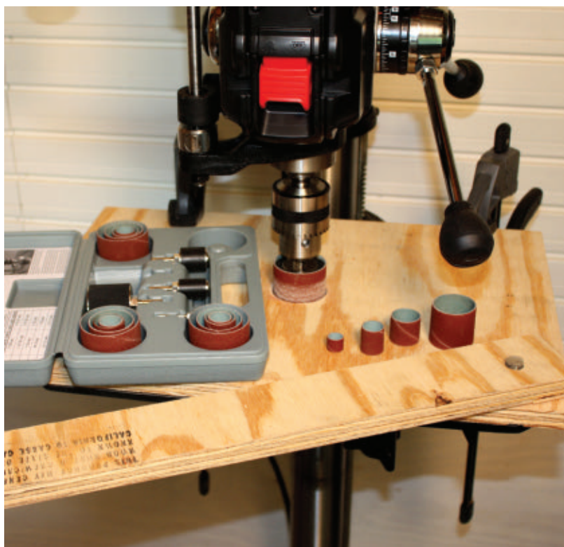
Drum-sanding attachments enable a drill press to sand the edges of boards and panels for assembling furniture and cabinetry.
