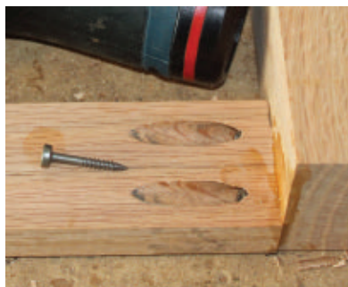
Glue and screw the frame pieces to the legs using the square-drive bit furnished with the kit.
