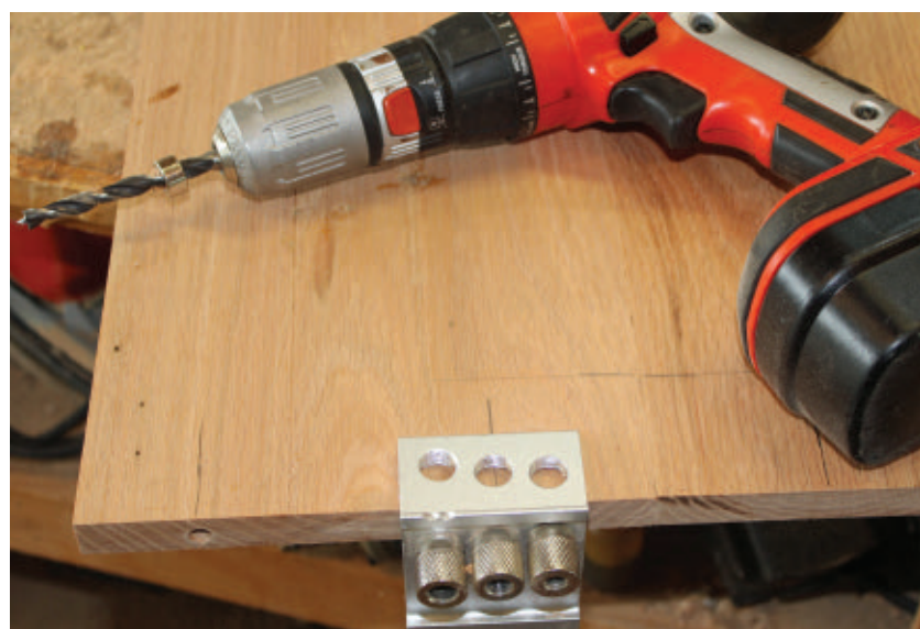
The breadboard ends are fastened in place with dowels. Mark and bore the holes, then add glue and dowels.
