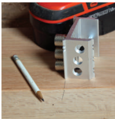
Lay the boards to be doweled together and mark across their edges. Then, using the doweling jig, bore the dowel holes.
