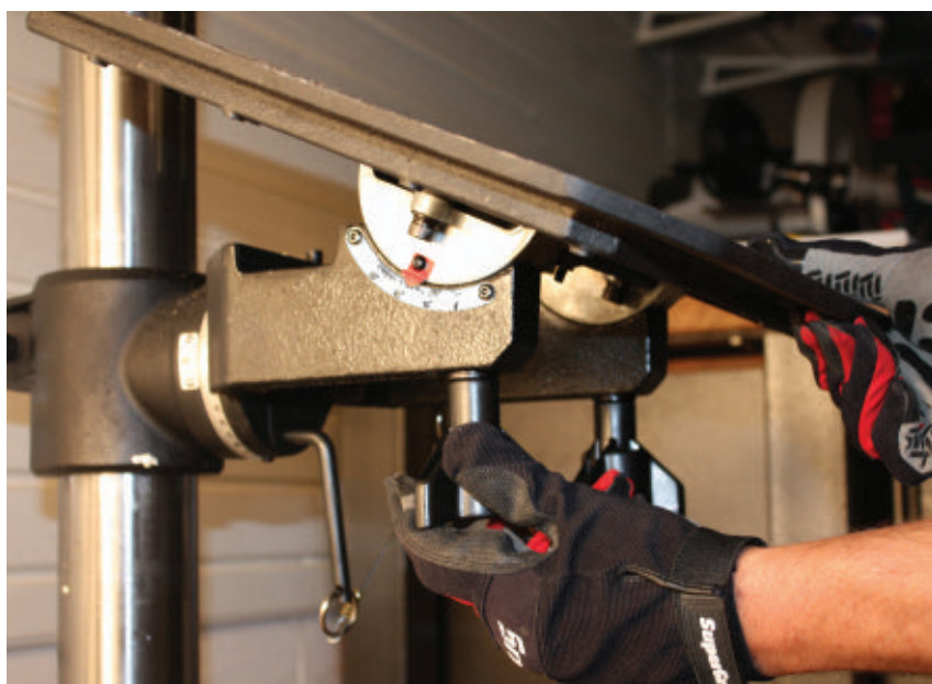
A work-support table is mounted to the post, and the table can be raised, lowered and pivoted to drill holes at a wide range of angles in workpieces of many different sizes.
