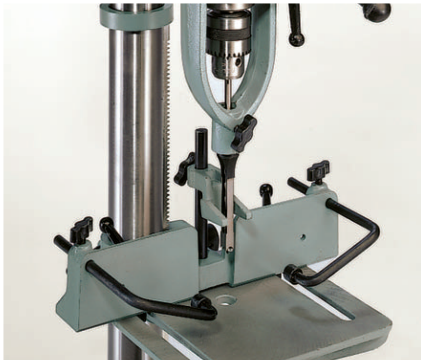
When equipped with a special accessory, drill presses can cut a mortise, which is a square or rectangular hole that receives a tenon, forming a strong woodworking joint. Photo courtesy Delta Machinery.
