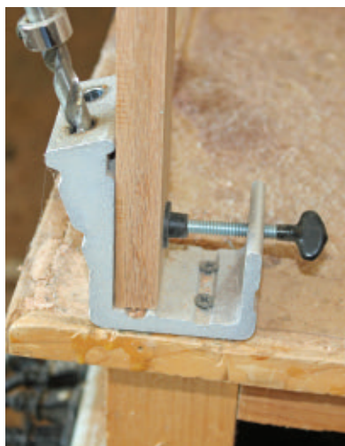
Fasten the jig to a sturdy work surface, and then bore the pocket holes using the stepped bit furnished with the kit. The stop collar on the bit sets the drilling depth.
