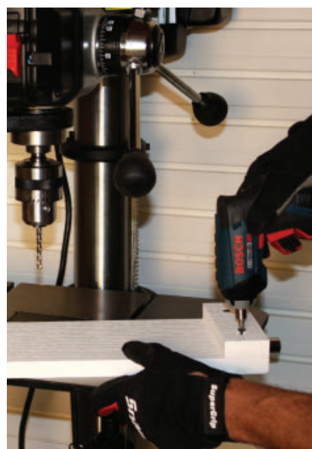
To assemble a straight-edge fence, fasten two rectangular blocks at the edges of a very straight board to tightly bracket the drill press table and guide the workpiece for repetitive drilling.
