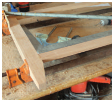
With the front and back frame pieces fastened to the legs, clamp until the glue sets. Use a carpenter's square and clamp to ensure the assembly is square before the glue sets up. Leave overnight.
