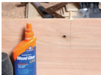
Run a bead of glue down in the dowel holes of one board and along the edge of the joining board and into the dowel holes. Tap the two together with a rubber mallet.
