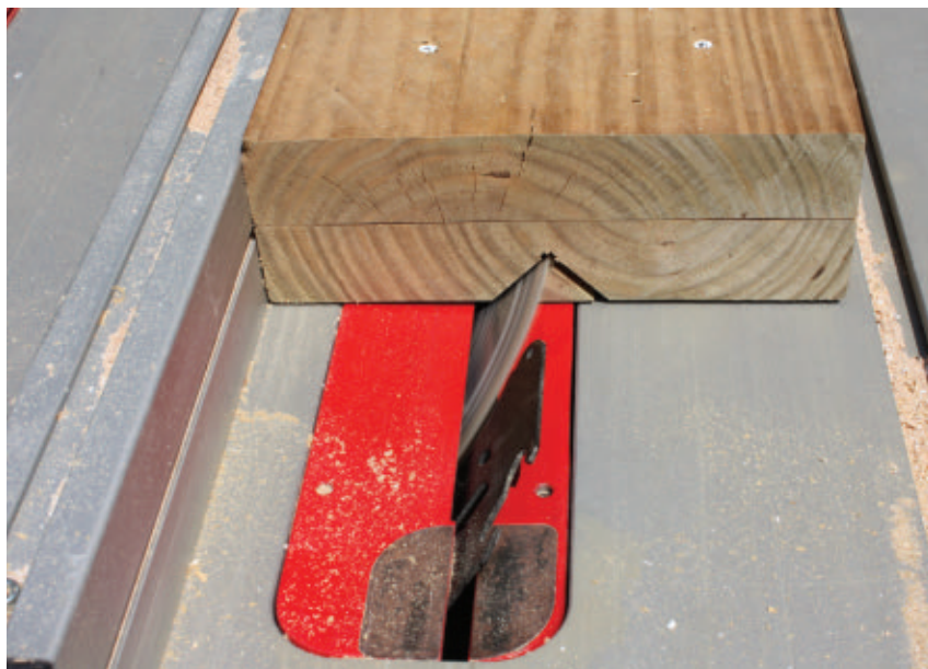
To make the pipe jig, I fastened together two 2x8s and cut a 90-degree V-notch down the center with a table saw.
