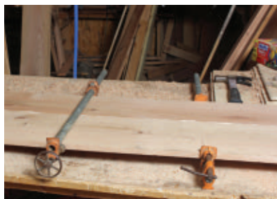
Clamp the glued-up stock and leave overnight. Make sure it is flat and not warped.
