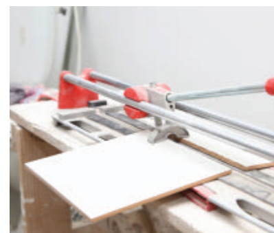
A snap tile cutter scores the face of the tile so you can break it cleanly along the score line.
