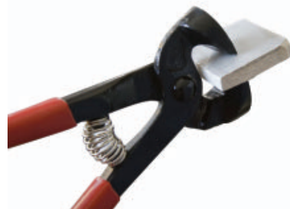
Use tile nippers to take small, controlled bites out of tile when fitting around an obstacle. Picture © feferoni / 123RF
