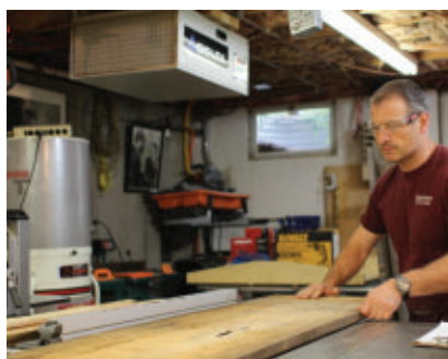
First step was to cut the door blanks to size with a table saw.
