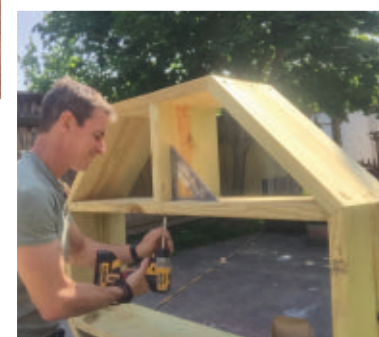
Using a 1x to mark the 2x for the half-miter on shelf material is easier than measuring.
