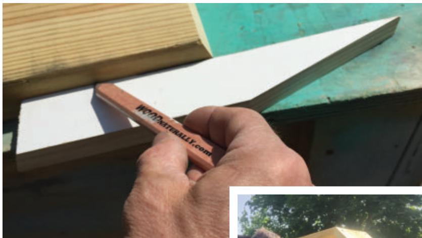
Using a 1x to mark the 2x for the half-miter on shelf material is easier than measuring.
