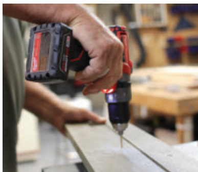
Finally, drill holes to mount the knobs or pulls.
