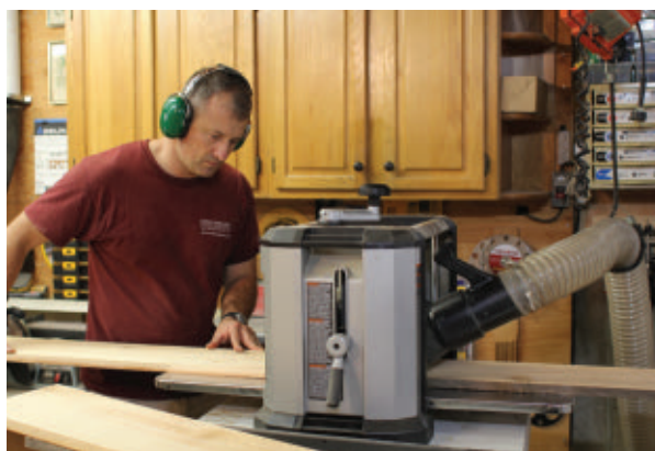
A power planer is an excellent tool for thinning the wood stock.
