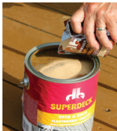
The additive, made of ground walnut hulls, is used one packet per gallon of product.
