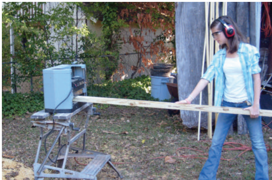
After removing the old boards, the first step was to plane down each "2x4" from 1-1/2 to 1-1/8 inch thick.
