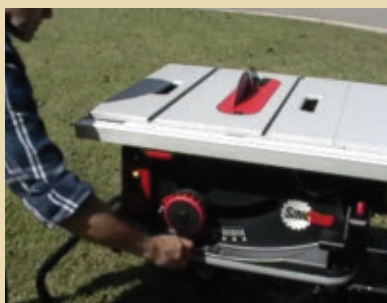
Raise blade with single turn of the wheel.
