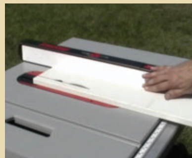
Accurate cuts with T-style rip fence.
