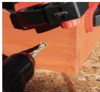
Drill a hole through both mating boards for the carriage bolt.
