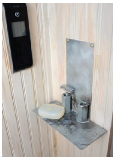
I added a little of my own personalization. A shower caddy soldered with my Bernzomatic propane torch, some threaded couplings and nailing plates. To keep it from rusting (mostly on the back) I sprayed a few coats of Krylon clear coat. The soap adds near instant patina.
