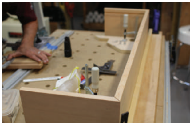
Assembly begins with one long wall and two side panels for each window box.
