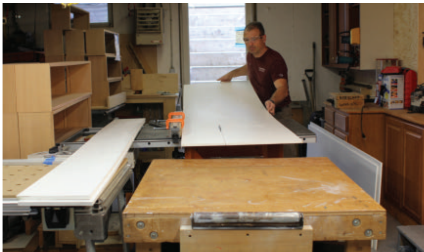
The bottom panels are cut from rot-resistant PVC.
