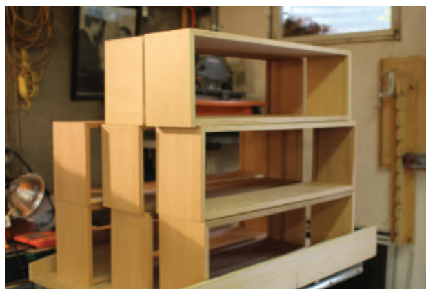
Dry-fit all the panels before final assembly.
