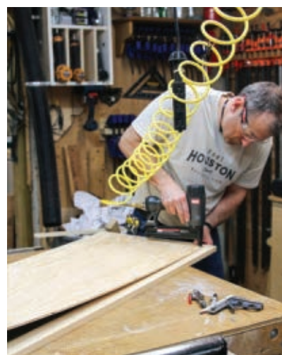
Fasten the backer-board over the rear of the slate.
