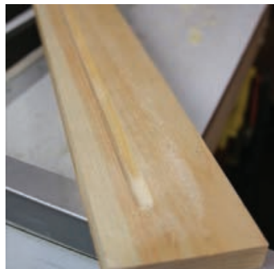
Use a thumbnail router bit to cut the slot.
