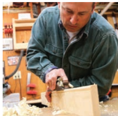
Remove any mill marks from the router with a block plane.
