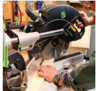
Cut miters to join the frame components.
