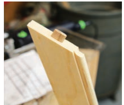
Insert the domino in the slot to bridge the joint.
