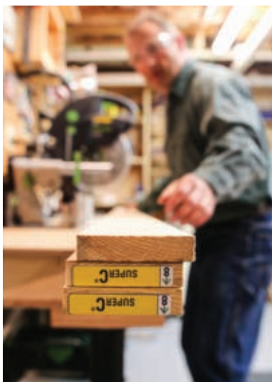
First, source all materials. The frame was built with No.1 pine.
