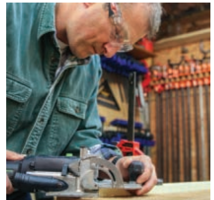
The frame was joined at the miters using a domino cutter, which is similar to a biscuit cutter.
