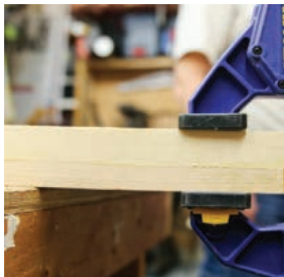
Fasten, glue and clamp the side pieces flush.
