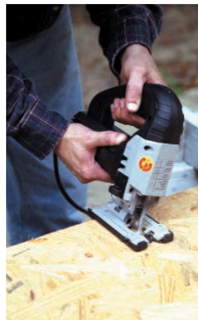
A jigsaw's footplate typically adjusts for bevel cuts between zero and 45 degrees.
