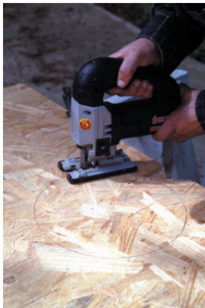
Use a compass to mark the radius for round cuts. Note the traditional D-style handle of this Freud jigsaw.
