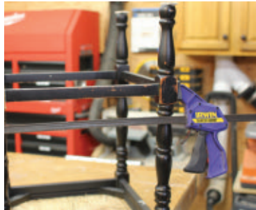
Clamp the repair overnight.
