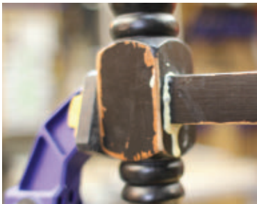
Reinsert the tenon and wipe away excess glue.
