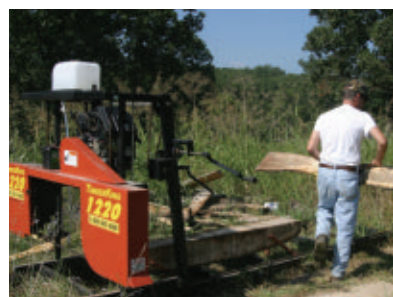
The ultimate for home-shop milling is a bandsaw mill, such as the Timber King model shown. These mills are portable, waste little wood and are relatively safe and easy to use.
