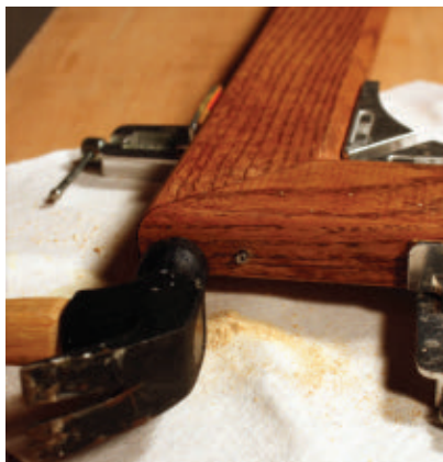
Use finish nails long enough to penetrate substantially into the mating stick of moulding.
