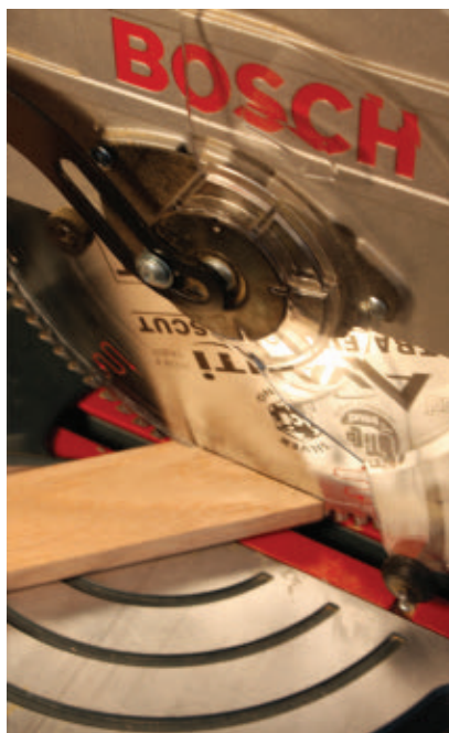
For square frames, all miters are simple 45-degree cuts.
