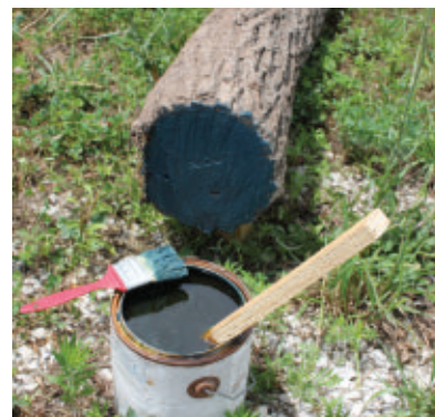
If small logs for turning are to be stored for some time before use, their ends should be coated with exterior house paint.
