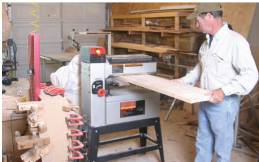
A drum sander is used to sand and smooth the glued-up countertop.
