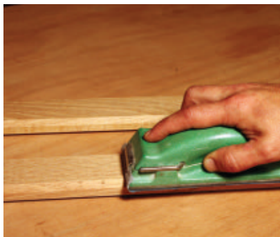
Sand the moulding smooth before applying a wood stain.
