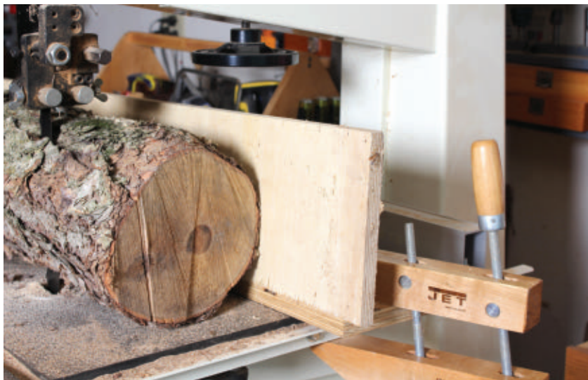
A shop-made fence, clamped to the saw table, holds the logs in place for the cuts. You can cut planks or even veneer with a bandsaw setup.
