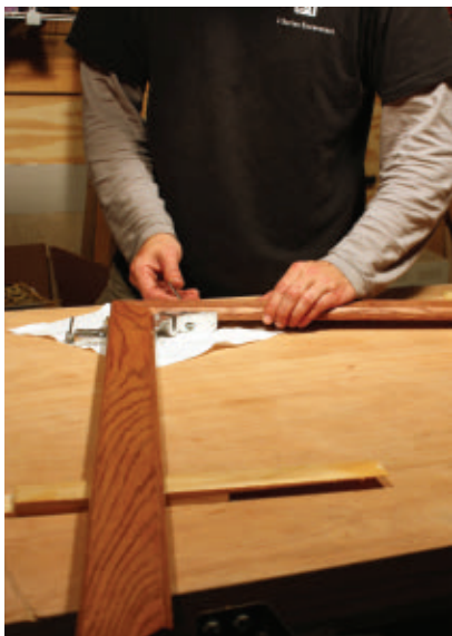
Support the long ends of the moulding sticks with shims to relieve tension on the clamped joints.
