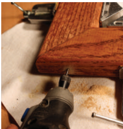
Predrill the nail holes to avoid splitting.
