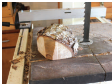
You can also cut wood-turning blanks quickly and easily on the bandsaw. One wood-turning technique is turning green, bark-on bowls. First step is to rough-cut on the bandsaw.
