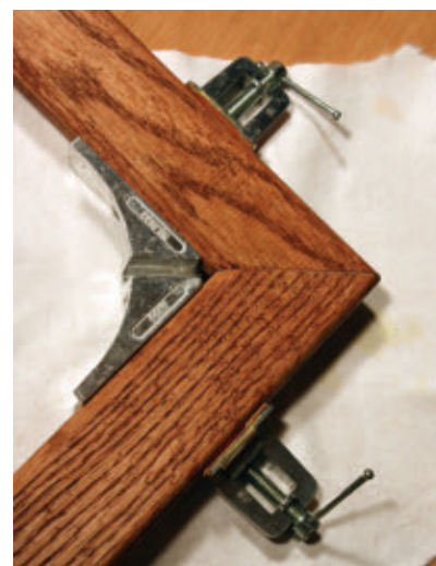
Miter clamps will hold the joints securely while the wood dries and the nails are driven.
