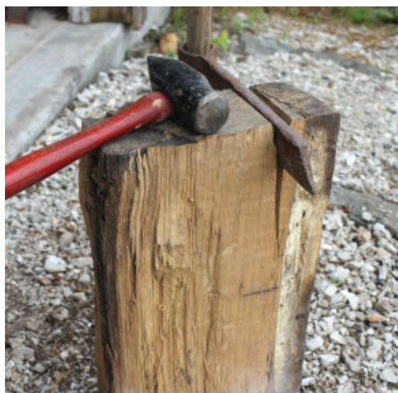
The old-fashioned way of getting small pieces was often using a maul or froe to split log sections. Then, shape the surfaces with a hand plane.
