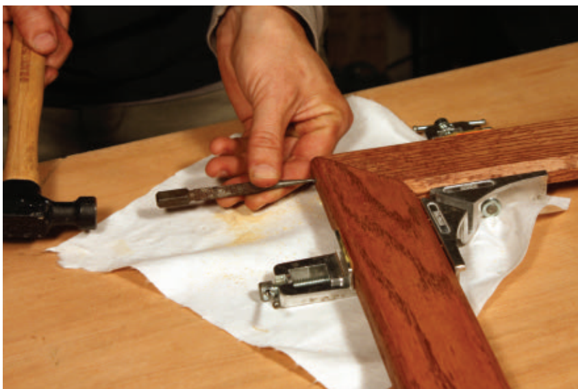
Set the nail heads below the wood surface.
