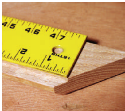
When transferring the dimensions of the artwork to the molding, make sure to take the measurements from the longest point of the rabbet.
