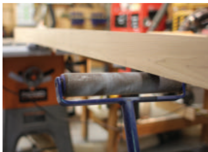
Arrange an outfeed roller or other system to support the workpiece.
