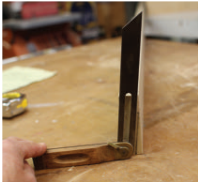
Use an angle gauge to measure the bevel.
