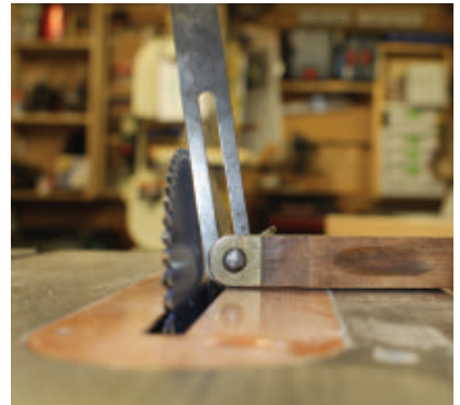
Set your table saw blade to a matching angle.
