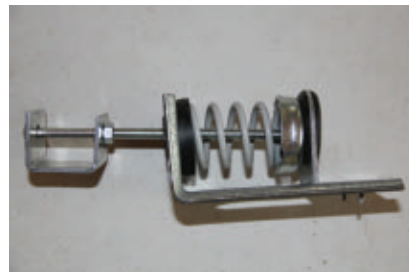
Kinetics Model ICW Wood Frame Ceiling Hangers were installed to decouple the ceiling drywall from the framing.
