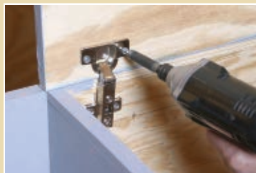
The doors operate using hidden Euro-style hinges.
