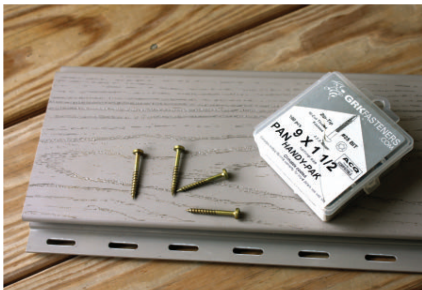
The PVC decking from Genova Products is fastened to the deck joists with pan-head screws driven through slots in a nailing flange, which allow the boards to move with temperature changes.
