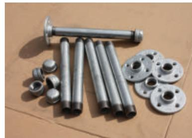
*The shelf brackets are built from 3/4" galvanized pipe, end caps and floor flanges.*
