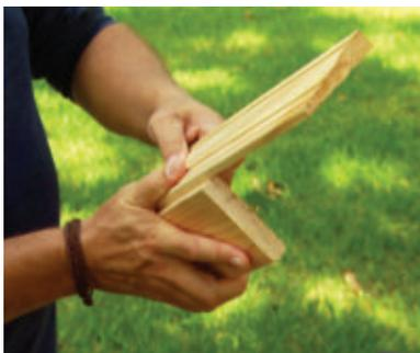
The molding should reveal 1/8" of the box's inner edge.
