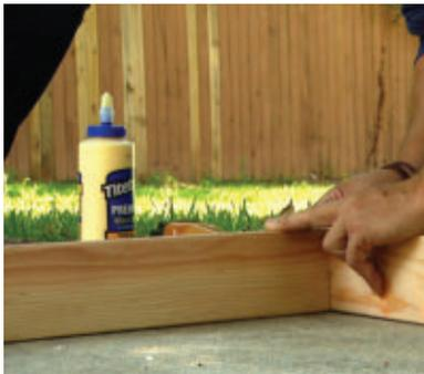
Apply wood glue to the miter joints.
