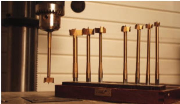
on the edge of a block of wood to create channels, and can also be used to create overlapping holes. The Kik bits also come in a nice, dovetailed wooden box to protect the cutting edges. Visit [www.mytgtools.com](http://www.mytgtools.com) or booth 39087.
