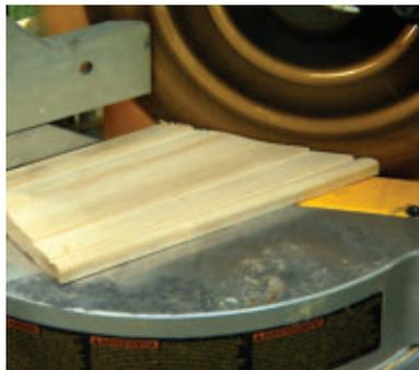
Cut inside miters with the long points on the thick edge of the molding.
