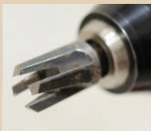
We used this plug cutter to cut plugs for the newel post with matching material.
