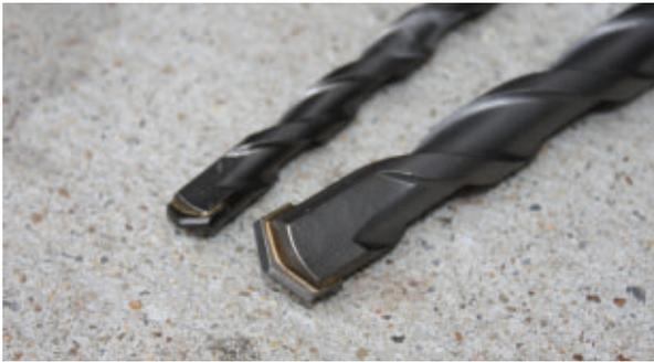
Vanadium steel for toughness and long life. The carbide tip is made of heavier stock than common masonry drills and silver soldered in place. The shoulders of the Chrome Vanadium drill shaft are then precision ground to expose the carbide properly to the material. Visit [www.mytgtools.com](http://www.mytgtools.com) or booth 39087.
