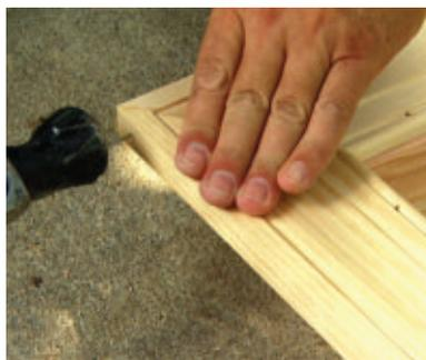
Carefully fasten the joints with small finish nails or an air-driven pin nailer.
