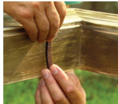
Apply felt strips to the inside of the box.
