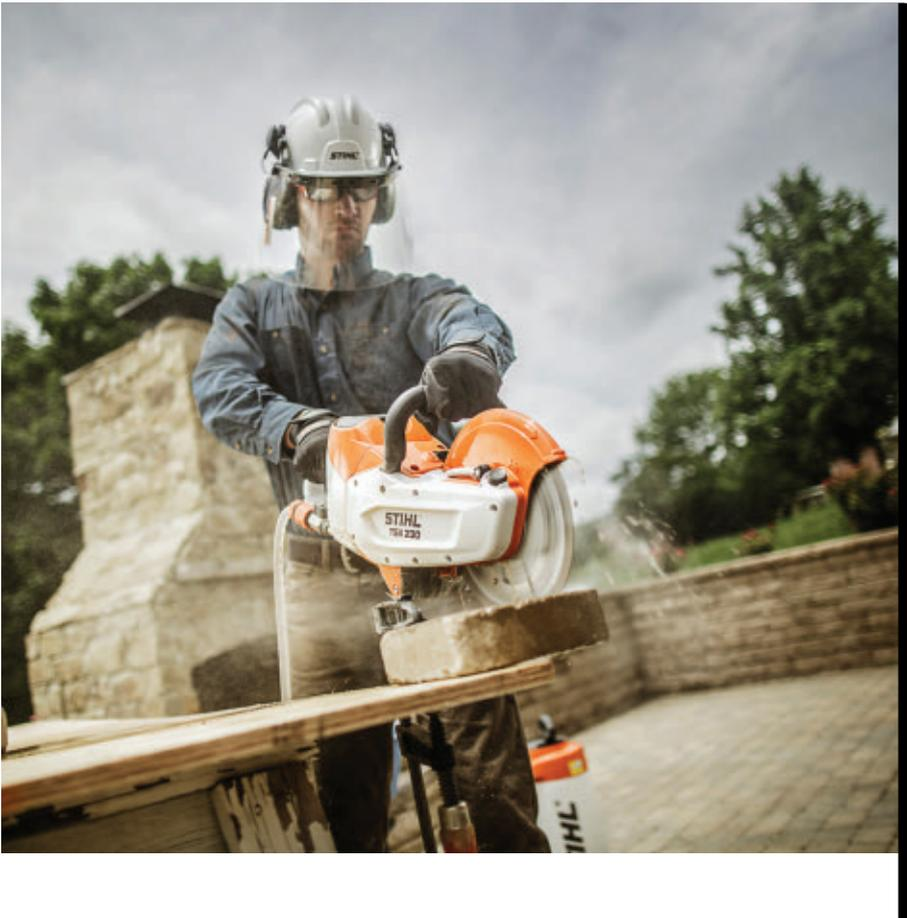
water-control suppresses masonry dust, and a tool-free locking device prevents wheel rotation when removing the wheel-attachment bolt. The TSA 230 also requires less maintenance and is priced below its gasoline-powered counterpart. (Battery and charger are sold separately.) Learn more at [www.stihlusa.com](http://www.stihlusa.com).
