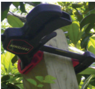
If working alone, a strong wood clamp can support the weight of one end of a 2x6 while you fasten the other.
