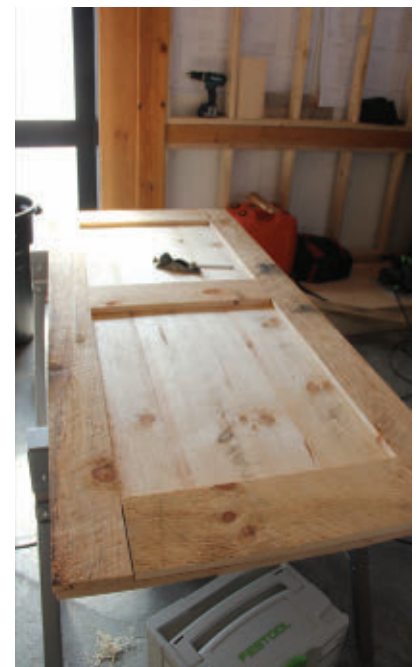
Cedar is often the preferred lumber for its inherent resistance to rot and insect infestation.
