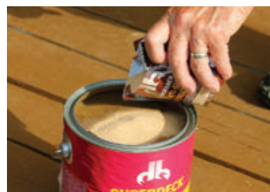
The additive, made of ground walnut hulls, is used one packet per gallon of product.
