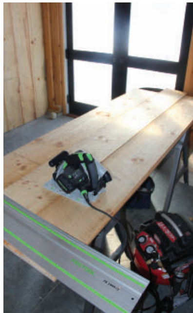
A circular saw with ripping gauge serves as an excellent tool combo for making long, accurate cuts.
