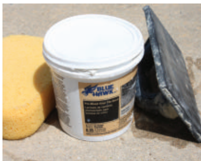
I used a pre-mixed grout specified for vinyl tile.
