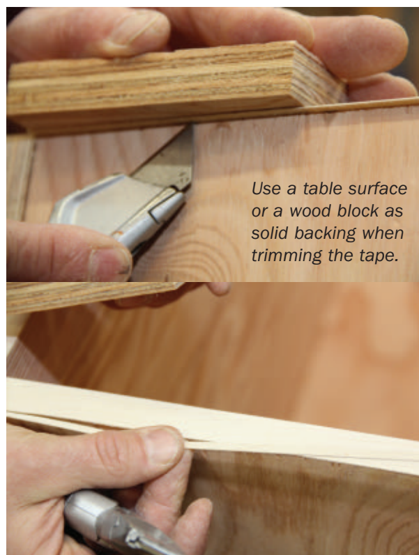
A sharp utility knife will make a clean cut through the tape.
