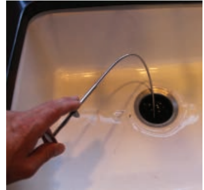
A prong retrieval tool has a flexible shaft to snake inside the pipes.
