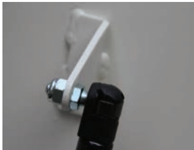
The gas spring pistons attach to brackets on the doors.
