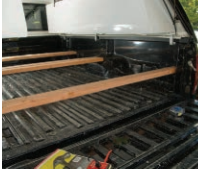
Two-by-4 cross supports fit into pockets in the bed walls.
