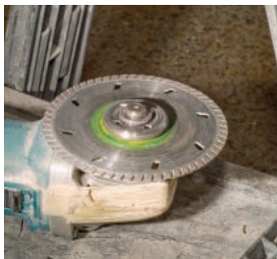
An angle grinder and diamond cut-off wheel are the primary tools of the stone counter do-it-yourselfer.
