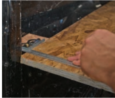
The shelf had to be fit to the irregular contours of the pickup bed walls. A combination square can be used to transfer marks.
