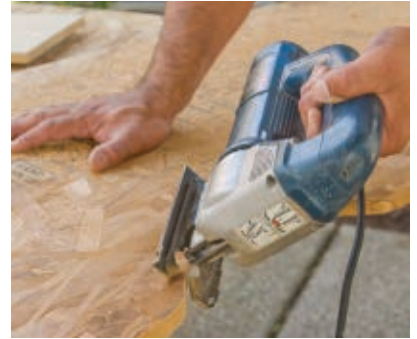
A jigsaw does a good job of cutting the scribe lines on the shelf. After adjusting the shelf with some back cuts, we used it to trace a layout for the other side of the pickup bed.
