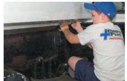
Eleven year old Garrett Christoffersen, an experienced canopy man, installs the clamps that attach the truck cap to the bed rails.
