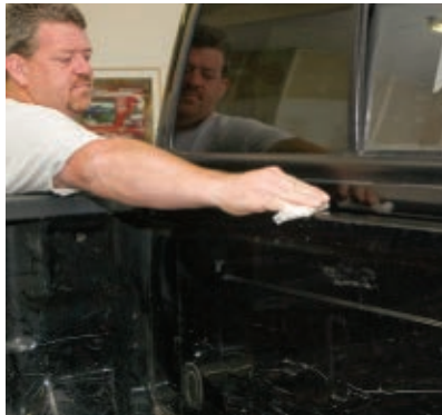
Harley Christoffersen of Canopies Plus, an A.R.E. dealer in Eugene, Oregon, preps the bed rails for the weather seals.
