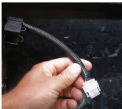
One of the secrets to a successful truck cap installation is getting a wiring harness for your application.
