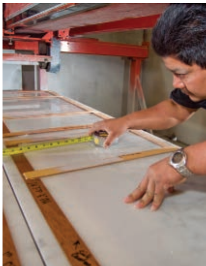
Wood-strip templates hold their shape in the wet conditions of a large stone saw.
