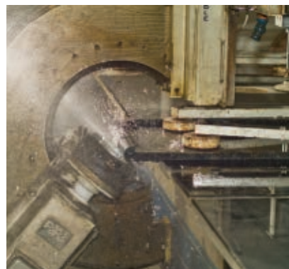
An automated edge shaping machine cuts and polishes a bull nose.
