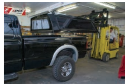
You probably don't have a fork lift with extended, padded forks, but a friend on each corner will do.
